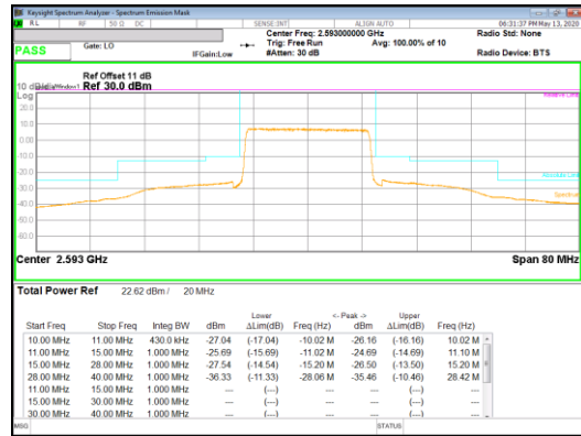
16QAM Mid channel FRB
