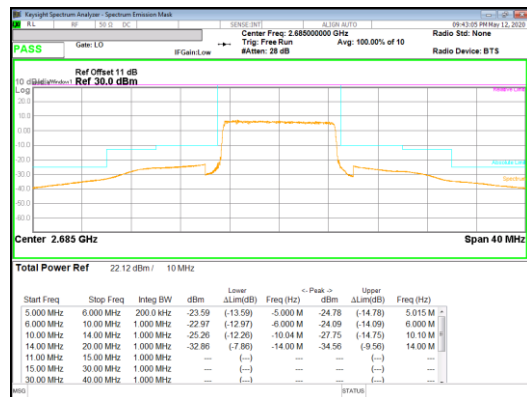
16QAM High channel FRB
