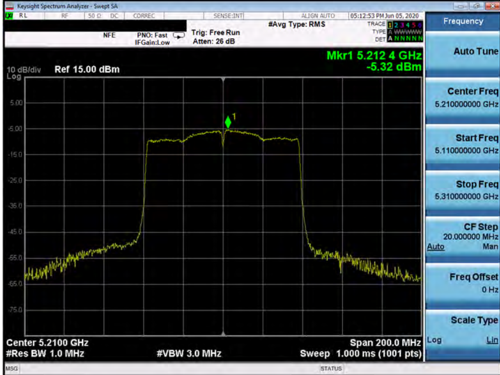
Plot 7-141. Power Spectral Density Plot SISO ANT1 (80MHz BW 802.11ax (UNII Band 1) – Ch. 42)
