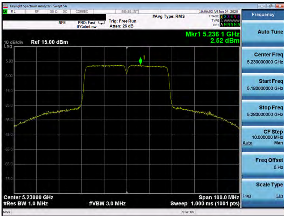
Plot 7-203. Power Spectral Density Plot SISO ANT2 (40MHz BW 802.11n (UNII Band 1) – Ch. 46)
