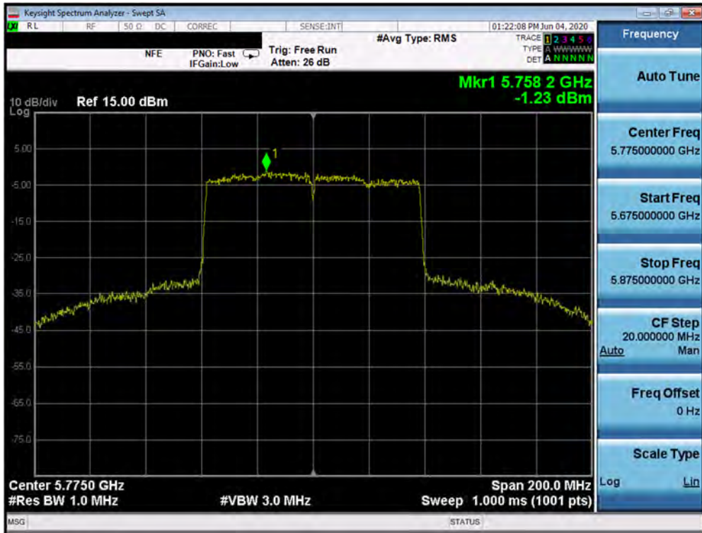
Plot 7-257. Power Spectral Density Plot SISO ANT2 (80MHz BW 802.11ac (UNII Band 3) – Ch. 155)
