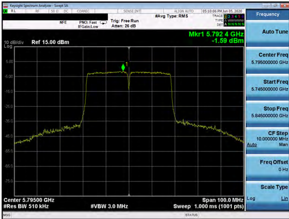
Plot 7-188. Power Spectral Density Plot SISO ANT1 (40MHz BW 802.11n (UNII Band 3) – Ch. 159)
