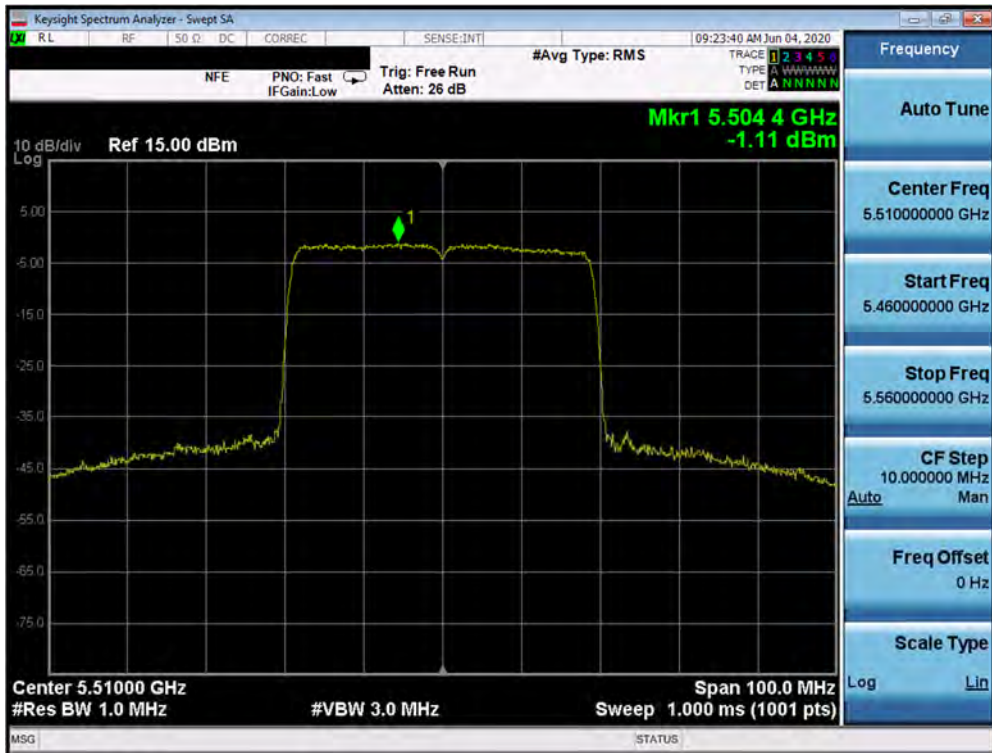
Plot 7-235. Power Spectral Density Plot SISO ANT2 (40MHz BW 802.11ax (UNII Band 2C) – Ch. 102)
