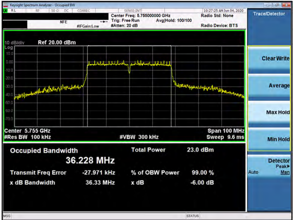
Plot 7-121. 6dB Bandwidth Plot SISO ANT2 (40MHz BW 802.11n (UNII Band 3) – Ch. 151)
