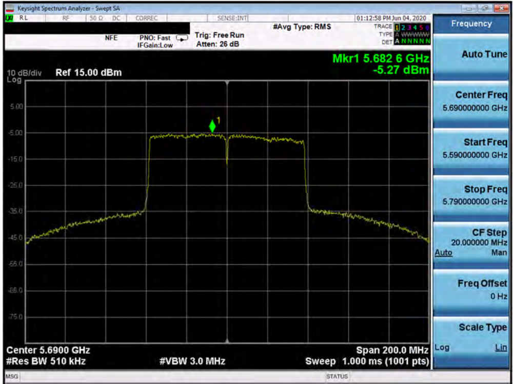
Plot 7-240. Power Spectral Density Plot SISO ANT2 (80MHz BW 802.11ac (UNII Band 2C) – Ch. 138)
