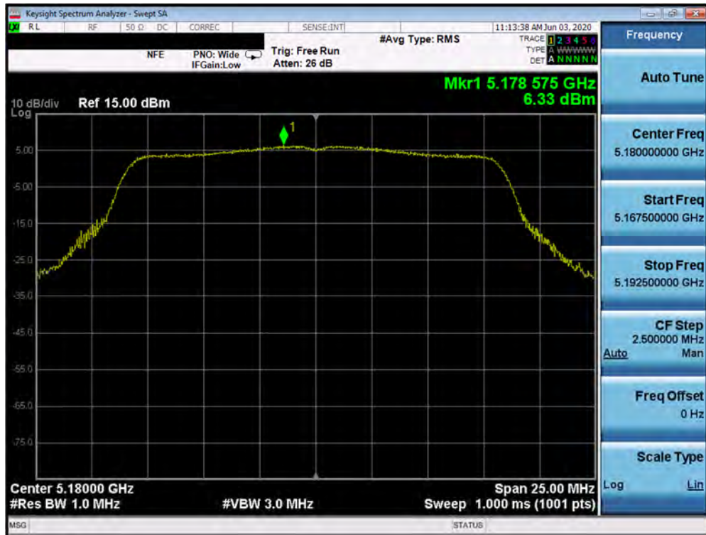
Plot 7-193. Power Spectral Density Plot SISO ANT2 (802.11a (UNII Band 1) – Ch. 36)
