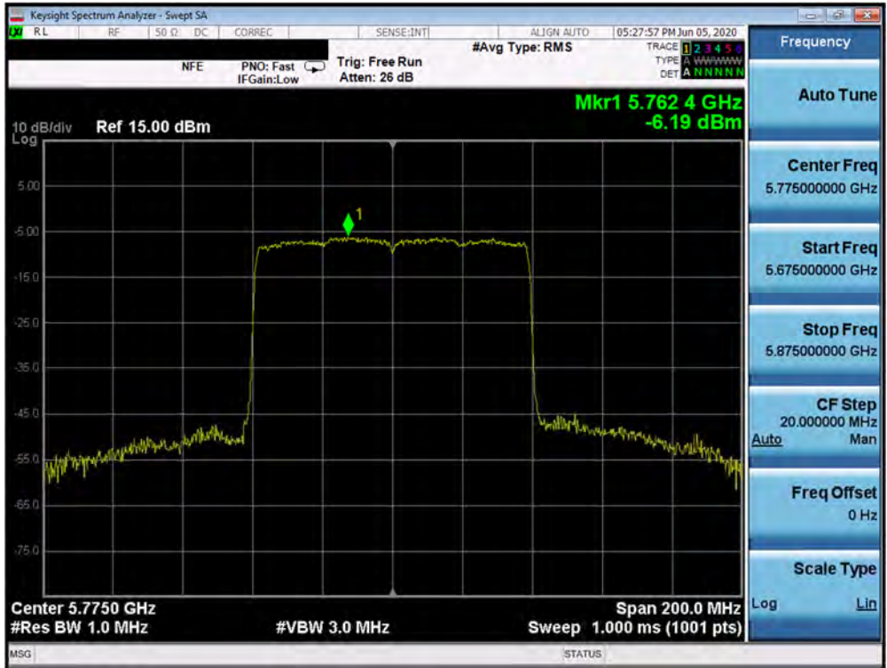
Plot 7-192. Power Spectral Density Plot SISO ANT1 (80MHz BW 802.11ax (UNII Band 3) – Ch. 155)
