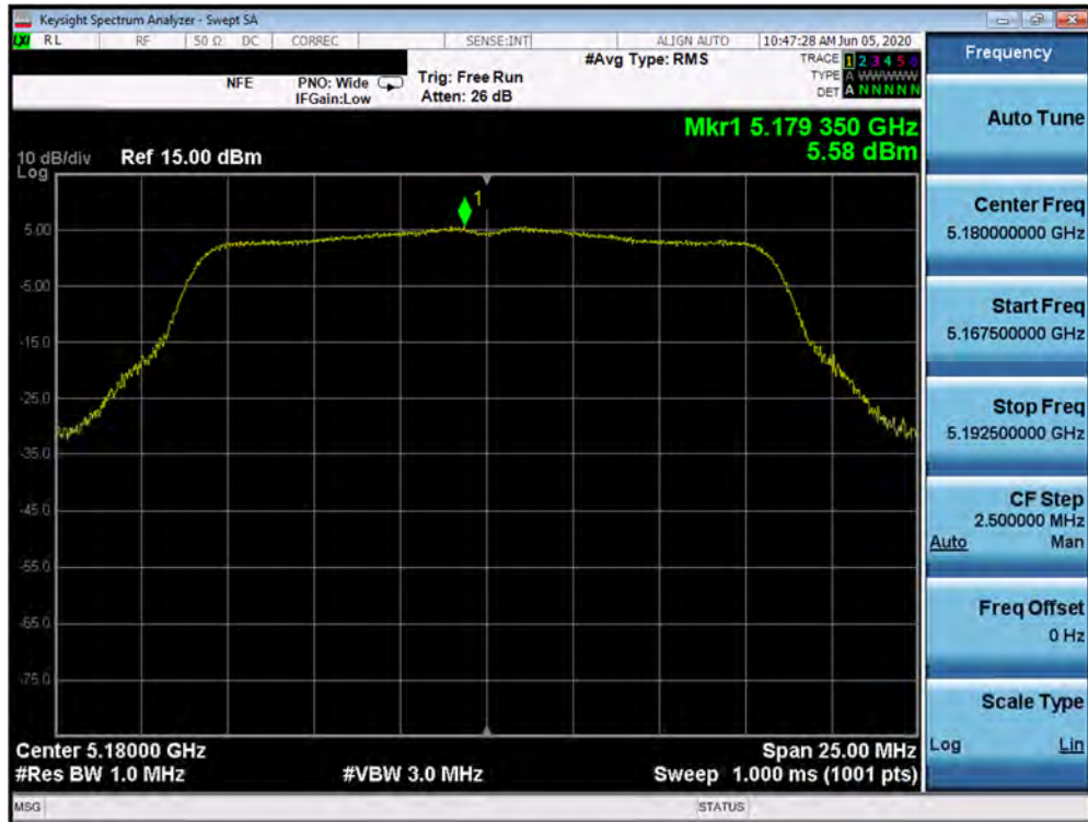
Plot 7-127. Power Spectral Density Plot SISO ANT1 (802.11a (UNII Band 1) – Ch. 36)
