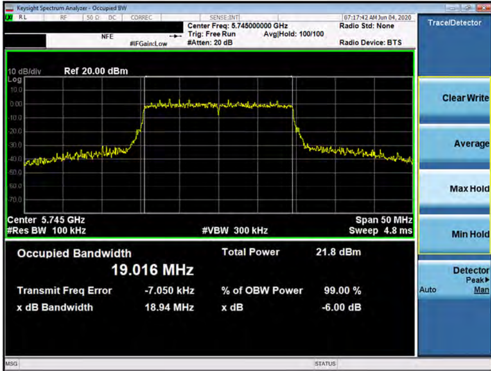
Plot 7-118. 6dB Bandwidth Plot SISO ANT2 (20MHz BW 802.11ax (UNII Band 3) – Ch. 149)
