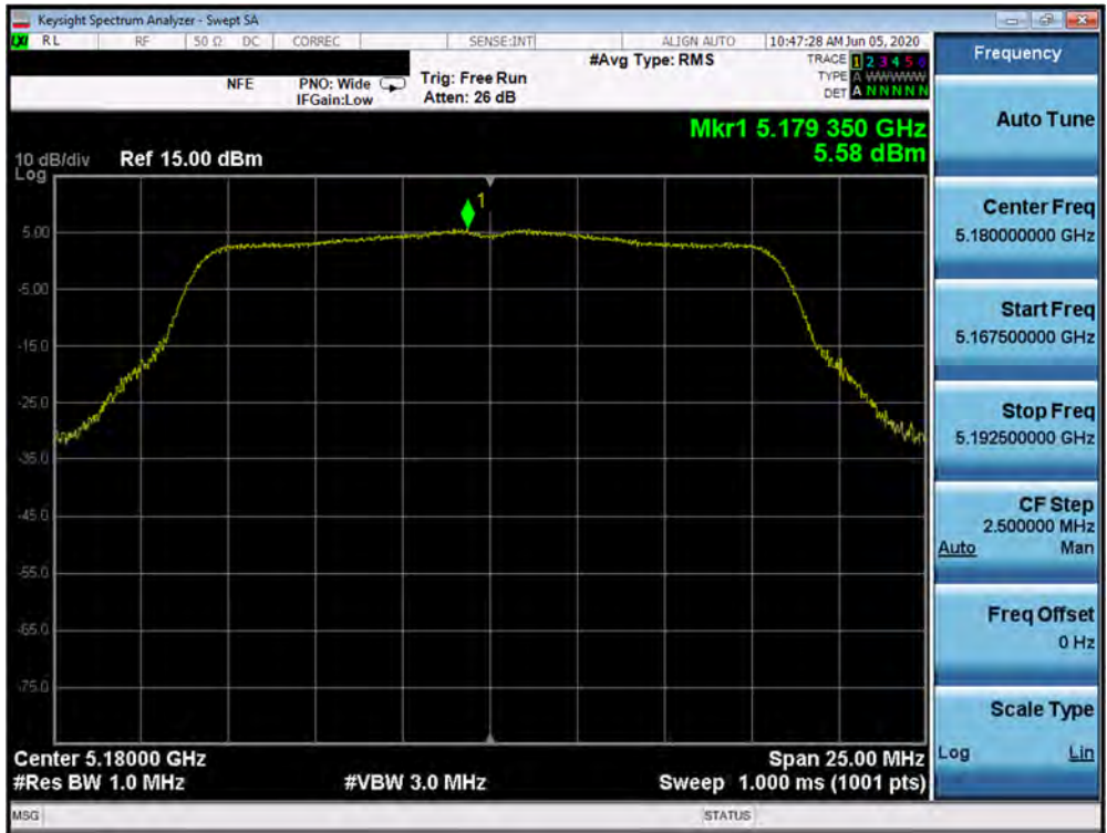
Plot 7-142. Power Spectral Density Plot SISO ANT1 (802.11a (UNII Band 2A) – Ch. 52)
