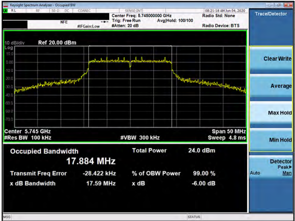
Plot 7-115. 6dB Bandwidth Plot SISO ANT2 (20MHz BW 802.11n (UNII Band 3) – Ch. 149)
