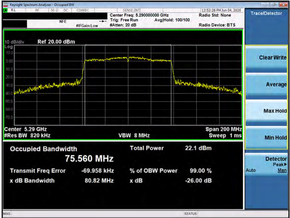
Plot 7-74. 26dB Bandwidth Plot SISO ANT2 (80MHz BW 802.11ac (UNII Band 2A) – Ch. 58)
