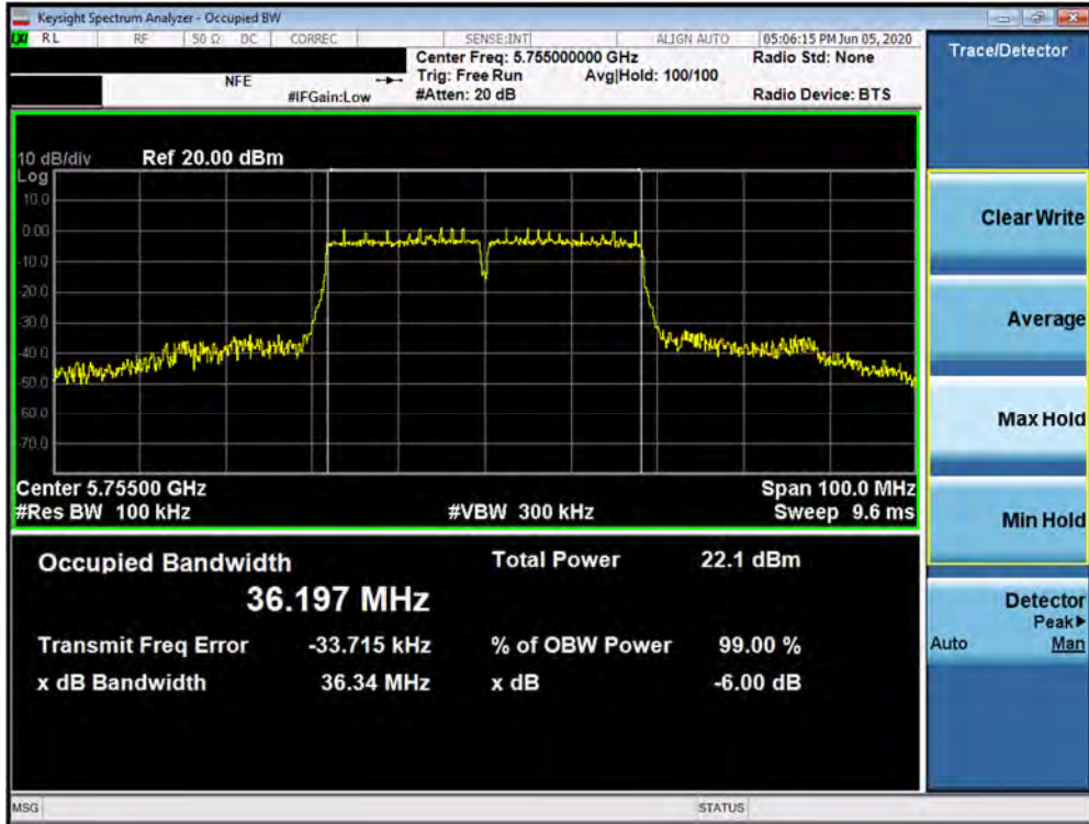
Plot 7-106. 6dB Bandwidth Plot SISO ANT1 (40MHz BW 802.11n (UNII Band 3) – Ch. 151)
