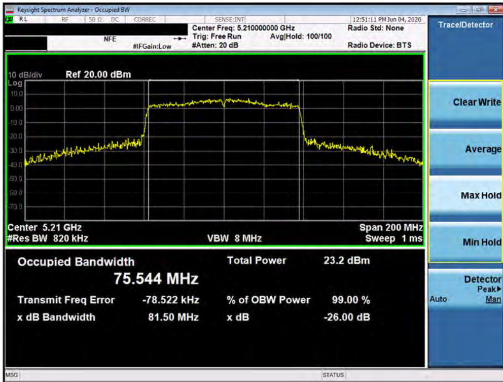
Plot 7-59. 26dB Bandwidth Plot SISO ANT2 (80MHz BW 802.11ac (UNII Band 1) – Ch. 42)
