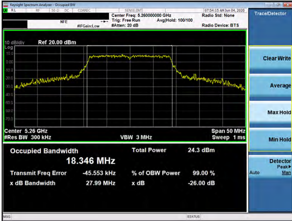
Plot 7-64. 26dB Bandwidth Plot SISO ANT2 (20MHz BW 802.11n (UNII Band 2A) – Ch. 52)
