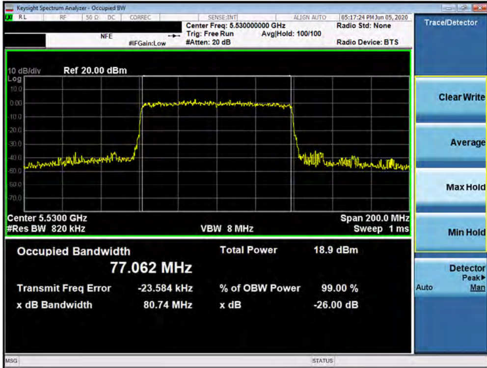
Plot 7-43. 26dB Bandwidth Plot SISO ANT1 (80MHz BW 802.11ax (UNII Band 2C) – Ch. 106)
