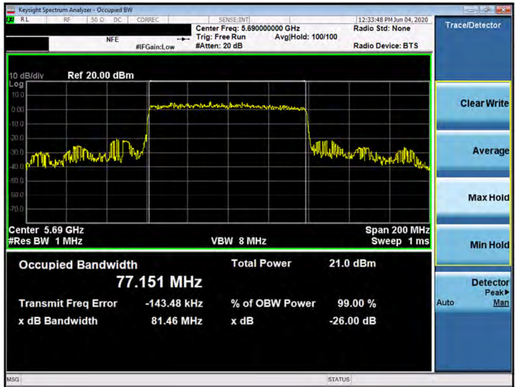
Plot 7-96. 26dB Bandwidth Plot SISO ANT2 (80MHz BW 802.11ax (UNII Band 2C) – Ch. 138)
