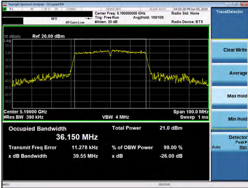
Plot 7-7. 26dB Bandwidth Plot SISO ANT1 (40MHz BW 802.11n (UNII Band 1) – Ch. 38)
