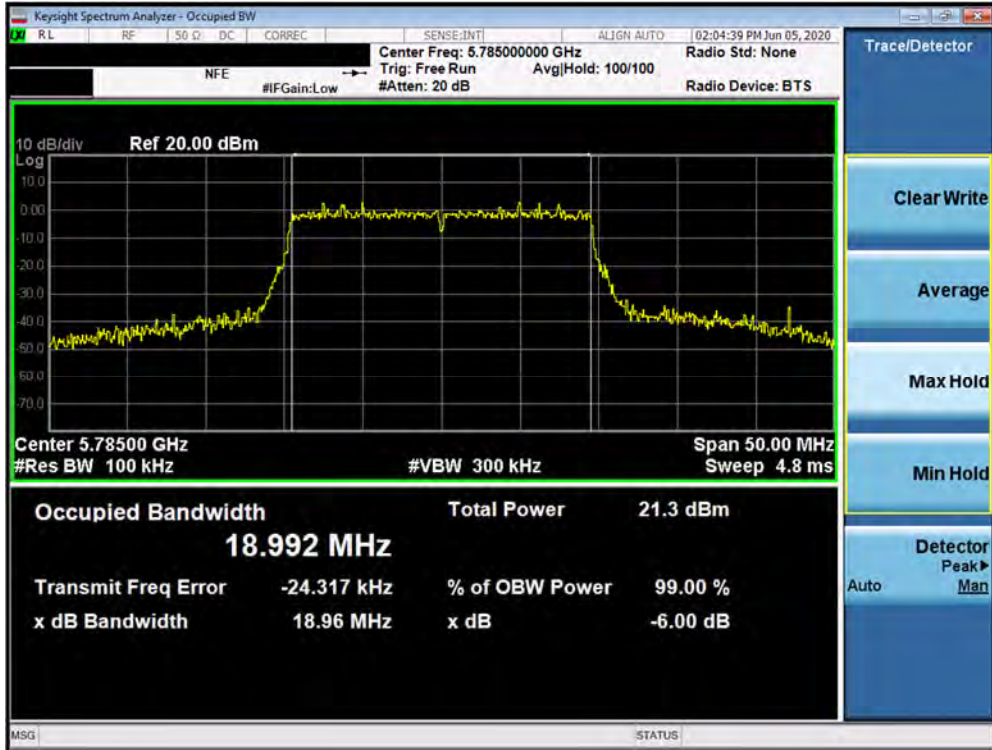
Plot 7-104. 6dB Bandwidth Plot SISO ANT1 (20MHz BW 802.11ax (UNII Band 3) – Ch. 157)
