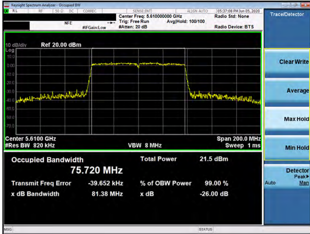
Plot 7-41. 26dB Bandwidth Plot SISO ANT1 (80MHz BW 802.11ac (UNII Band 2C) – Ch. 122)
