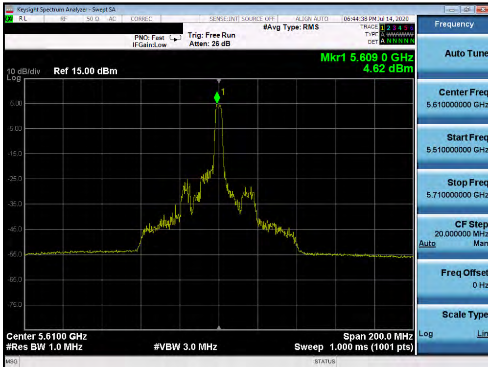
Plot 7-236. Power Spectral Density Plot MIMO ANT1 (80MHz BW 802.11ax – 26 Tones (UNII Band 2C) – Ch. 122)
