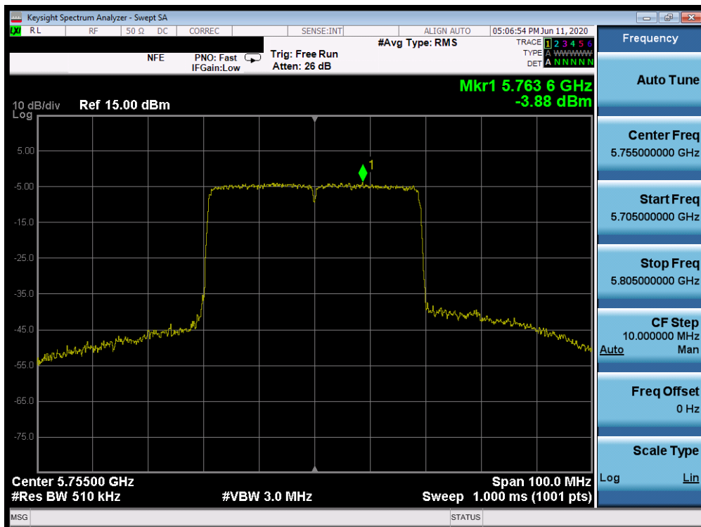
Plot 7-214. Power Spectral Density Plot SISO ANT2 (40MHz BW 802.11ax – Full Tones (UNII Band 3) – Ch. 151)
