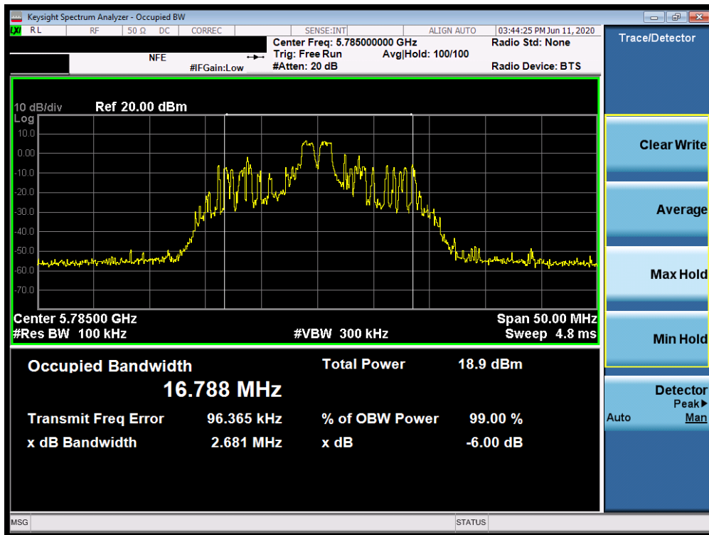
Plot 7-98. 6dB Bandwidth Plot SISO ANT2 (20MHz BW 802.11ax – 26 Tones (UNII Band 3) – Ch. 157)
