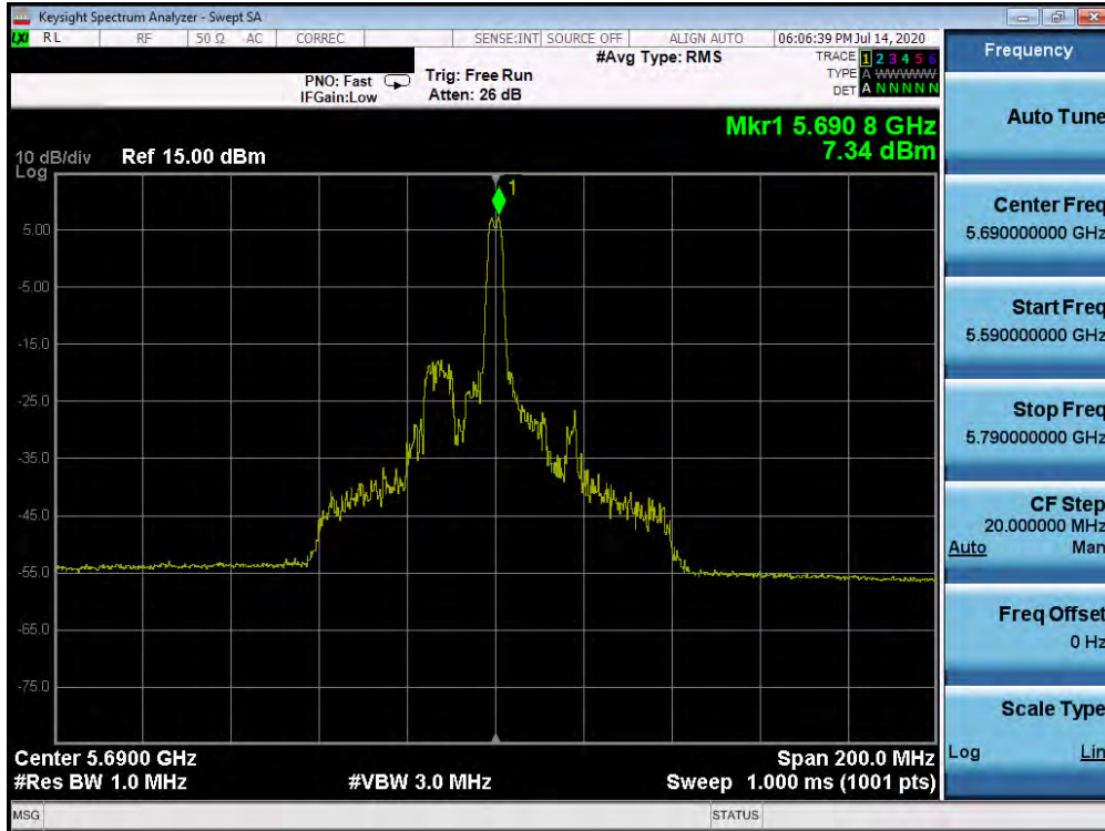
Plot 7-183. Power Spectral Density Plot SISO ANT2 (80MHz BW 802.11ax – 26 Tones (UNII Band 2C) – Ch. 138)
