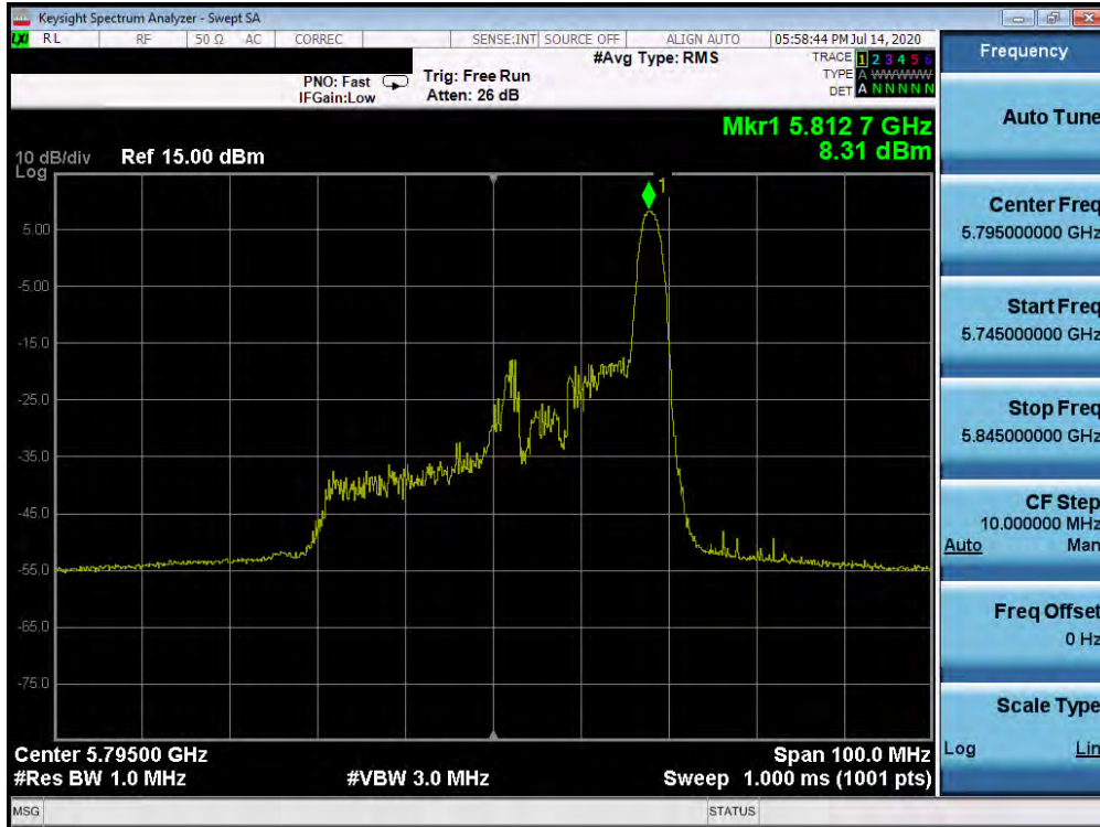
Plot 7-188. Power Spectral Density Plot SISO ANT2 (40MHz BW 802.11ax – 26 Tones (UNII Band 3) – Ch. 159)
