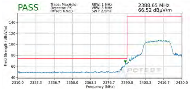
Plot 7-89. Radiated Restricted Lower Band Edge Measurement SISO ANT1 (Peak)
