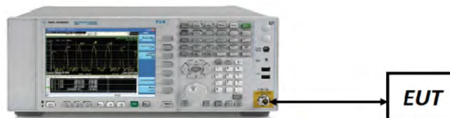
Figure 7-1. Test Instrument & Measurement Setup
