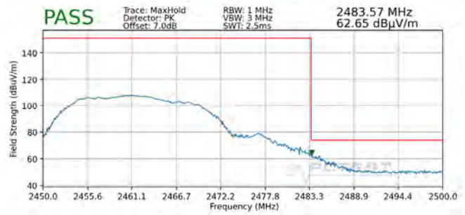
Plot 7-91. Radiated Restricted Upper Band Edge Measurement SISO ANT1 (Peak)
