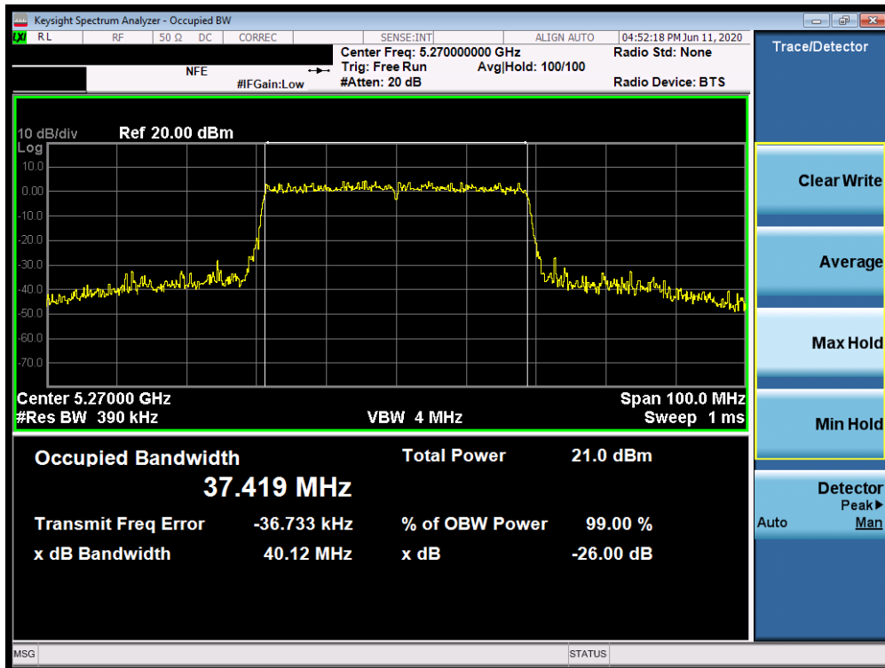
Plot 7-73. 26dB Bandwidth Plot SISO ANT2 (40MHz BW 802.11ax – 484 Tones (UNII Band 2A) – Ch. 54)
