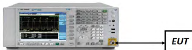
Figure 7-1. Test Instrument & Measurement Setup
