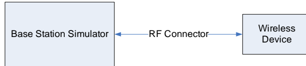
Figure 9-3 Power Measurement Setup
