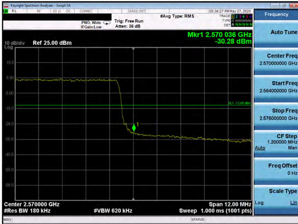
Plot 7-442. Upper Band Edge Plot (Band 7 - 15.0MHz QPSK - Full RB Configuration)
