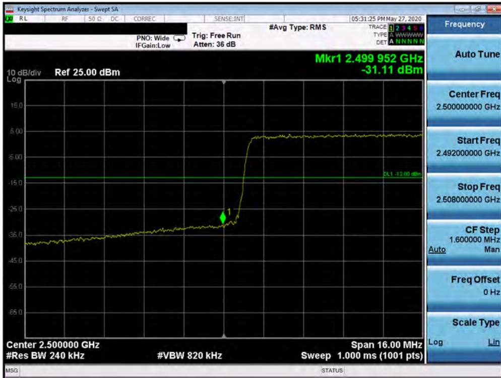
Plot 7-444. Lower Band Edge Plot (Band 7 - 20.0MHz QPSK - Full RB Configuration)
