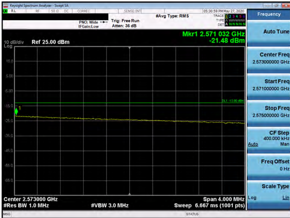
Plot 7-447. Upper Extended Band Edge Plot (Band 7 - 20.0MHz QPSK - Full RB Configuration)
