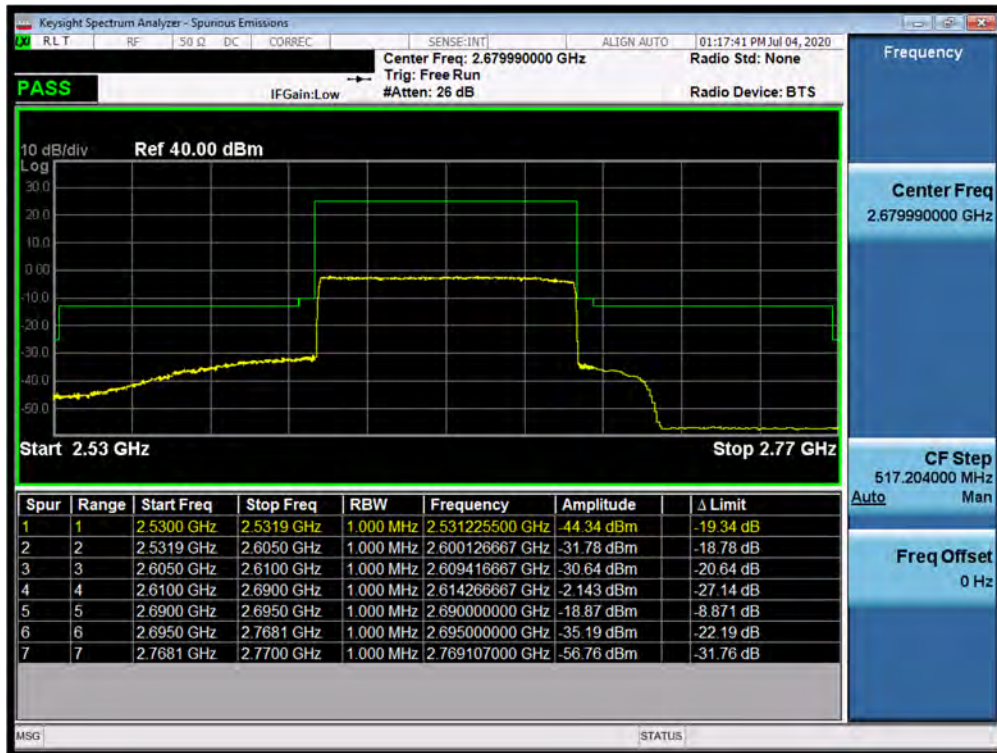
Plot 7-465. Upper ACP Plot (Band 41 - 80.0MHz DFT-s-OFDM-QPSK - Full RB Configuration)
