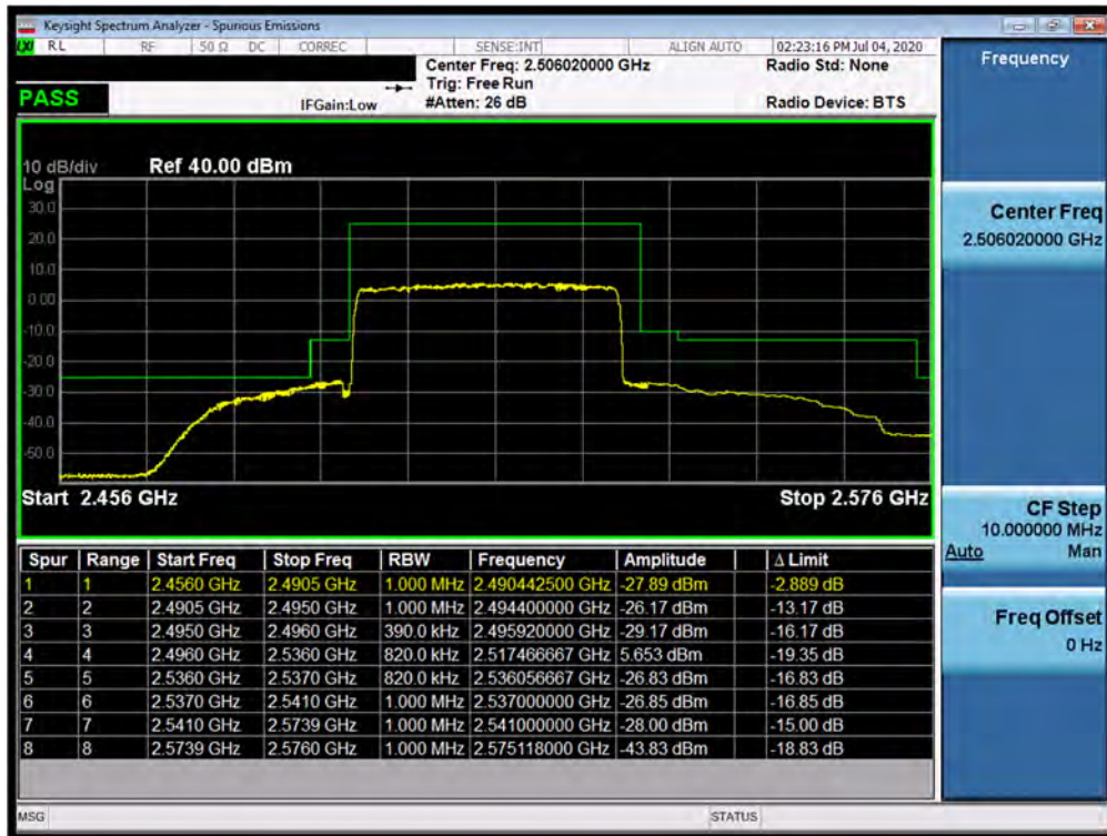
Plot 7-458. Lower ACP Plot at 2496 MHz (n41 - 40.0MHz DFT-s-OFDM-QPSK - Full RB Configuration)
