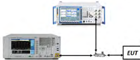
Figure 7-4. Test Instrument & Measurement Setup
