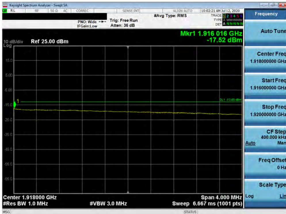
Plot 7-423. Upper Extended Band Edge Plot (Band 25 - 20.0MHz QPSK - Full RB Configuration)
