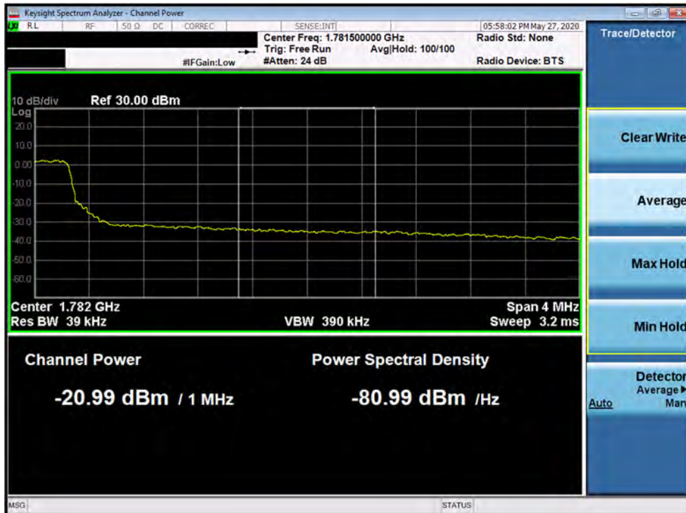
Plot 7-355. Upper Extended Band Edge Plot (Band 66 - 5.0MHz QPSK - Full RB Configuration)
