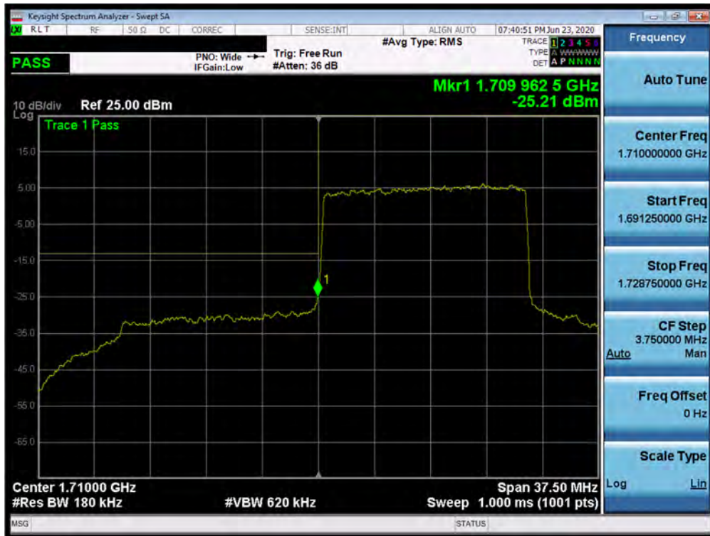
Plot 7-380. Lower Band Edge Plot (n66 - 15MHz DFT-s-OFDM-QPSK - Full RB Configuration)
