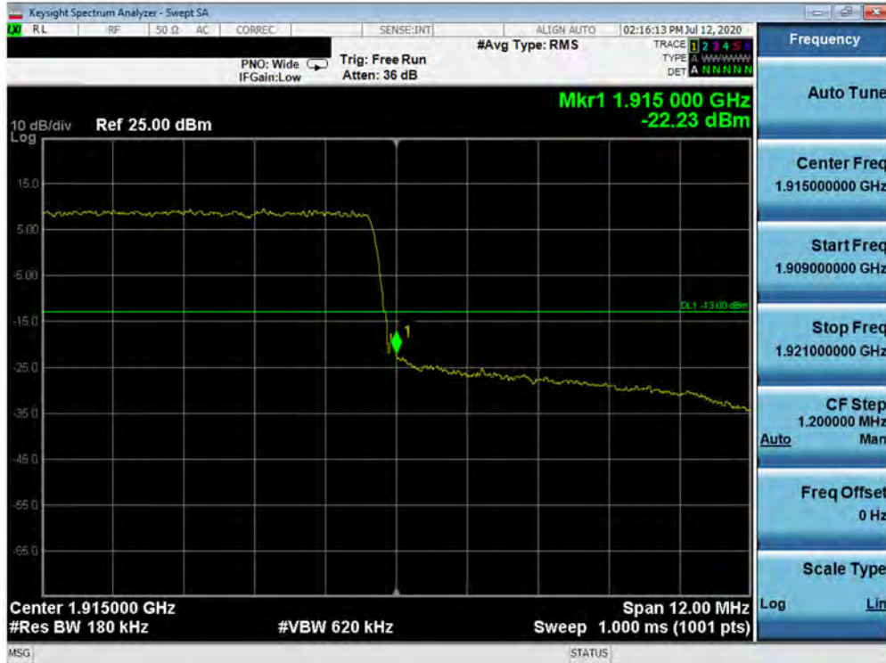
Plot 7-416. Upper Band Edge Plot (Band 25 - 15.0MHz QPSK - Full RB Configuration)
