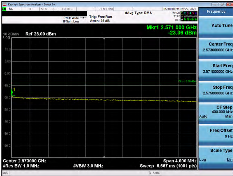
Plot 7-439. Upper Extended Band Edge Plot (Band 7 - 10.0MHz QPSK - Full RB Configuration)
