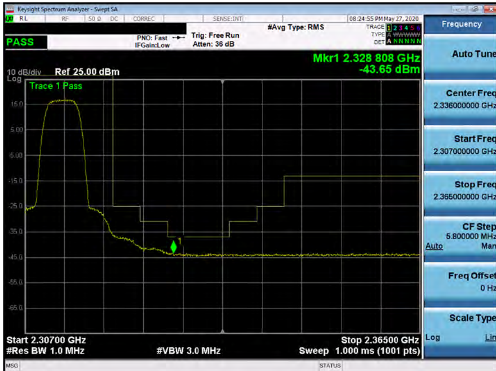
Plot 7-427. Upper Extended Band Edge Plot (Band 30 - 5.0MHz QPSK - Full RB Configuration)
