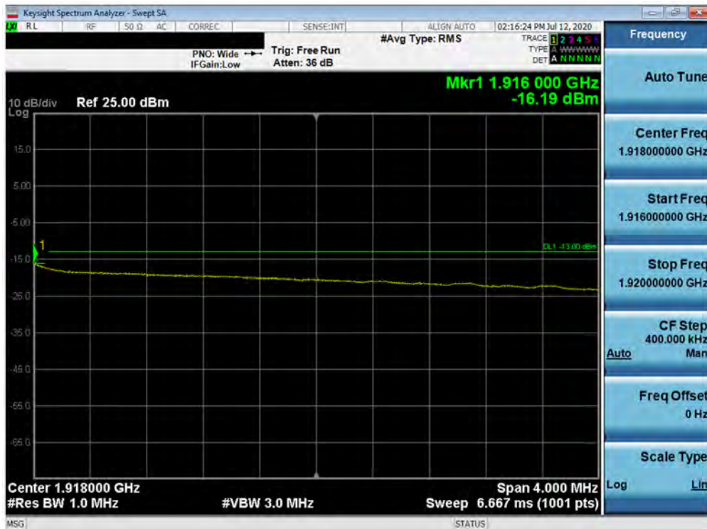
Plot 7-417. Upper Extended Band Edge Plot (Band 25 - 15.0MHz QPSK - Full RB Configuration)
