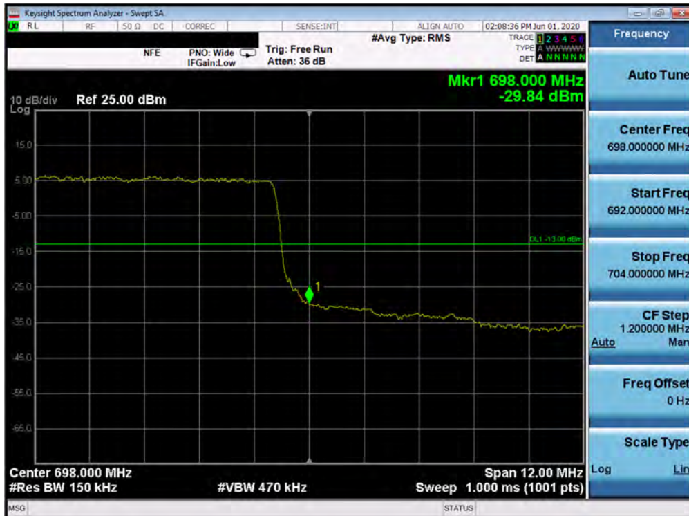
Plot 7-303. Upper Band Edge Plot (Band 71 - 15.0MHz QPSK - Full RB Configuration)
