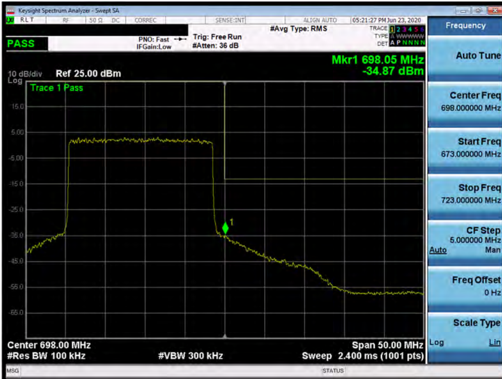
Plot 7-313. Upper Band Edge Plot (n71 - 20MHz DFT-s -OFDM-QPSK - Full RB Configuration)
