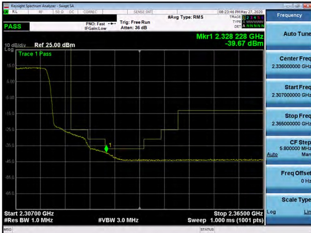
Plot 7-431. Upper Extended Band Edge Plot (Band 30 - 10.0MHz QPSK - Full RB Configuration)
