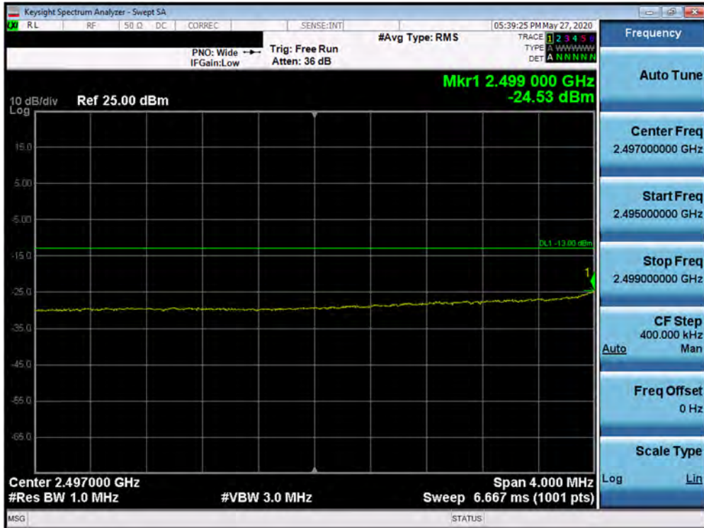
Plot 7-437. Lower Extended Band Edge Plot (Band 7 - 10.0MHz QPSK - Full RB Configuration)
