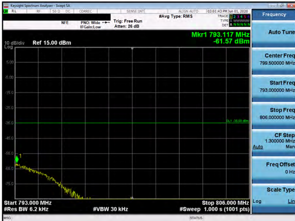
Plot 7-325. Upper Emission Mask Plot (Band 13 - 5.0MHz QPSK - Full RB Configuration)
