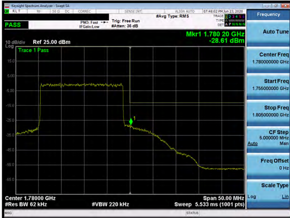
Plot 7-386. Upper Band Edge Plot (n66 - 20MHz DFT-s-OFDM-QPSK - Full RB Configuration)
