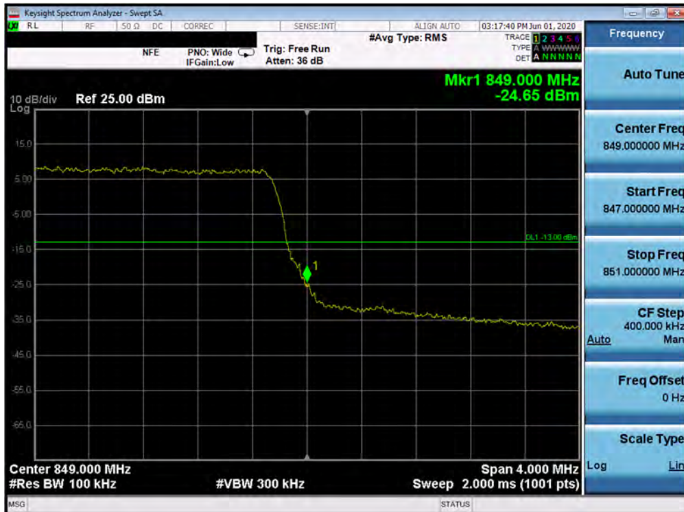
Plot 7-335. Upper Band Edge Plot (Band 5 - 5.0MHz QPSK - Full RB Configuration)
