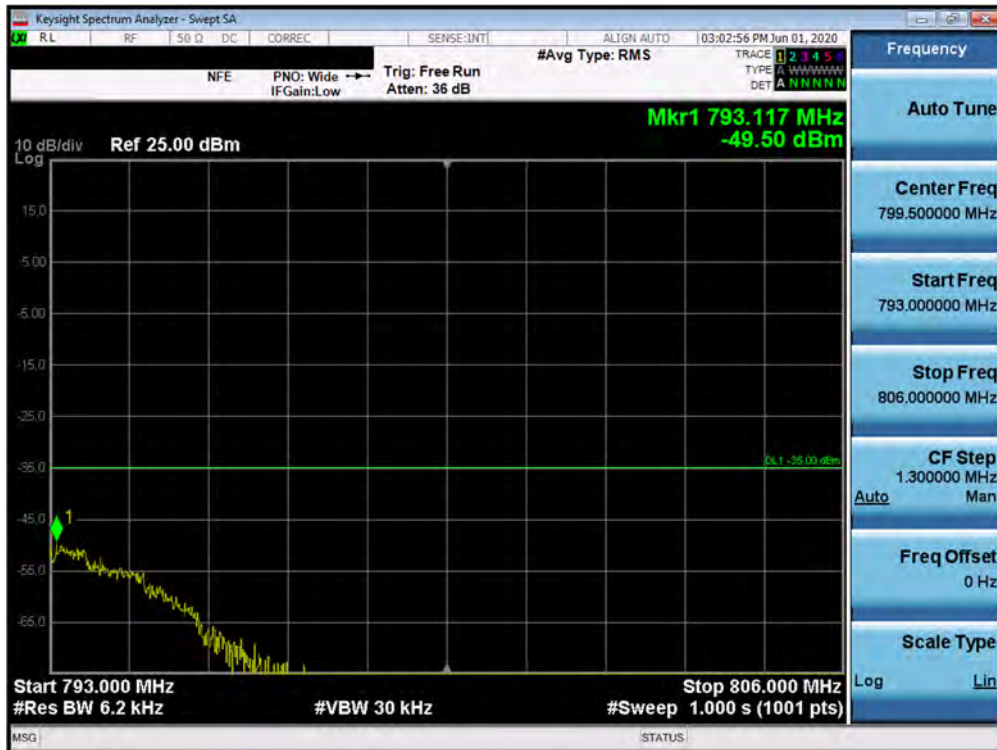
Plot 7-329. Upper Band Emission Mask Plot (Band 13 - 10.0MHz QPSK - Full RB Configuration)
