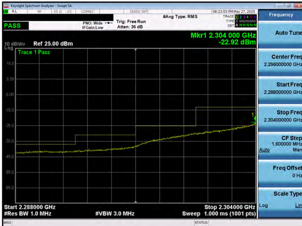
Plot 7-429. Lower Extended Band Edge Plot (Band 30 - 10.0MHz QPSK - Full RB Configuration)
