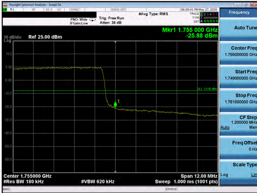
Plot 7-364. Upper Band Edge Plot (Band 4 - 15.0MHz QPSK - Full RB Configuration)
