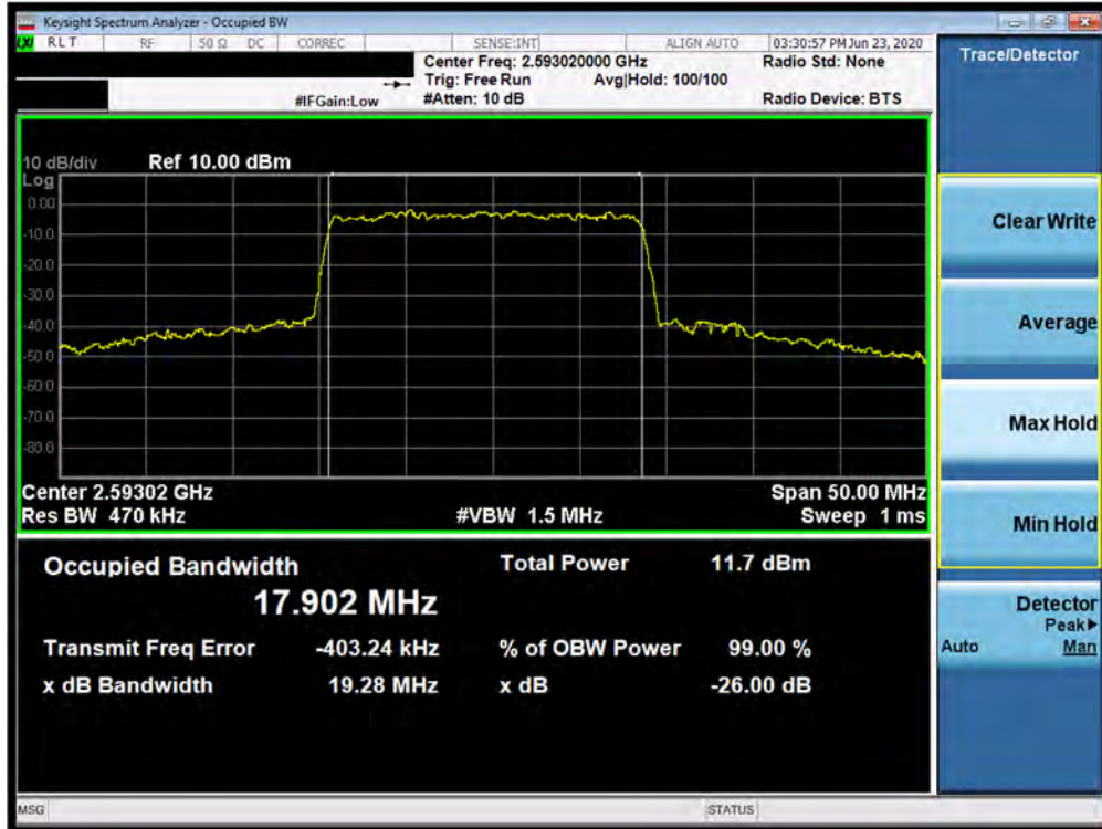
Plot 7-163. Occupied Bandwidth Plot (n41 20MHz 16QAM-CP-OFDM - Full RB Configuration)
