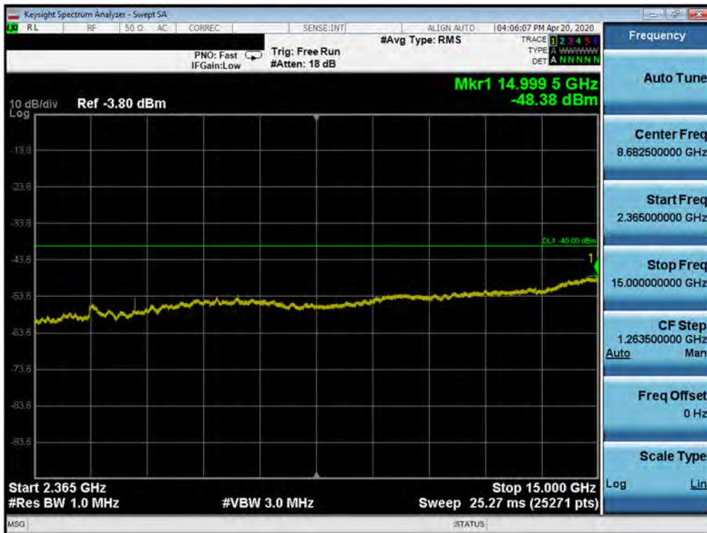
Plot 7-263. Conducted Spurious Plot (Band 30 - 10.0MHz QPSK - RB Size 1, RB Offset 0 - Mid Channel)
