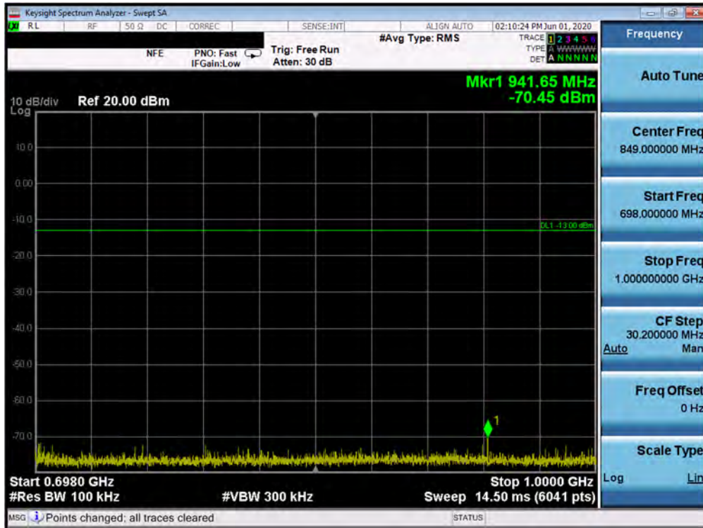
Plot 7-200. Conducted Spurious Plot (Band 71 - 20.0MHz QPSK - RB Size 1, RB Offset 0 - Mid Channel)
