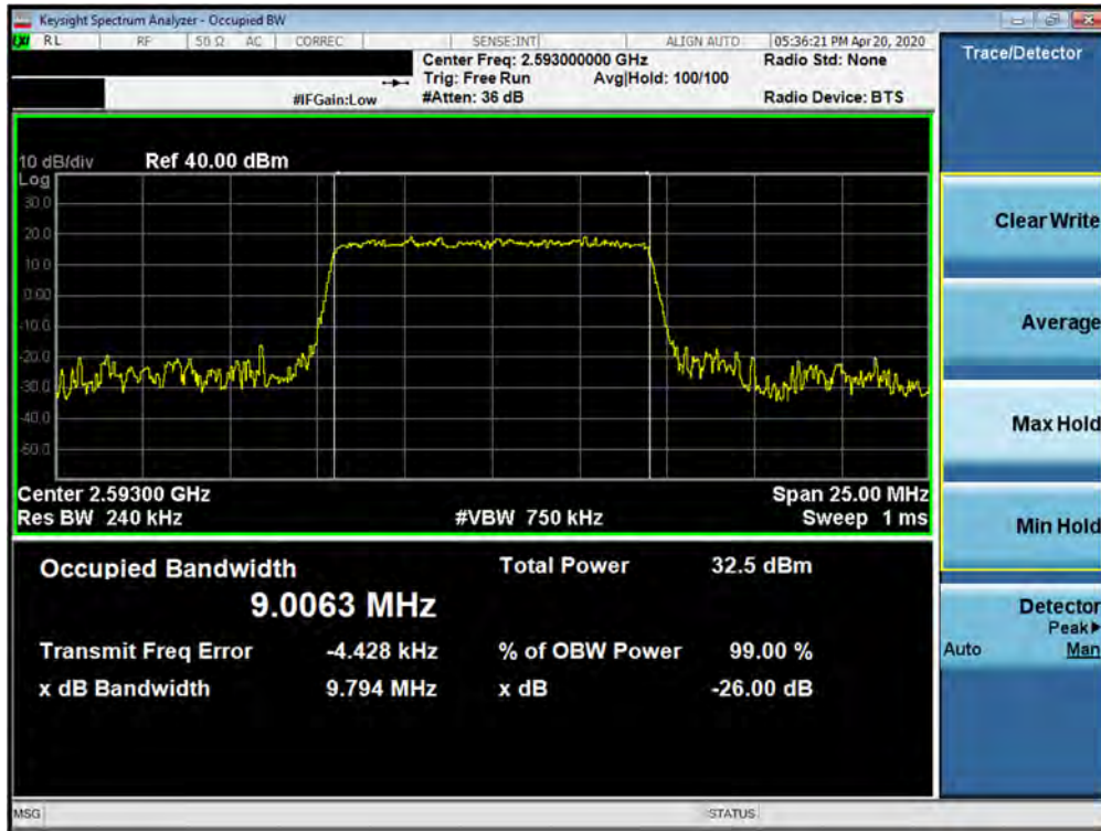
Plot 7-149. Occupied Bandwidth Plot (Band 41 - 10.0MHz QPSK - Full RB Configuration)
