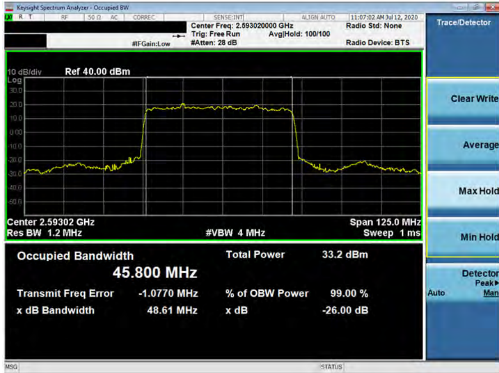
Plot 7-171. Occupied Bandwidth Plot (n41 50MHz BPSK-DFT-s-OFDM - Full RB Configuration)
