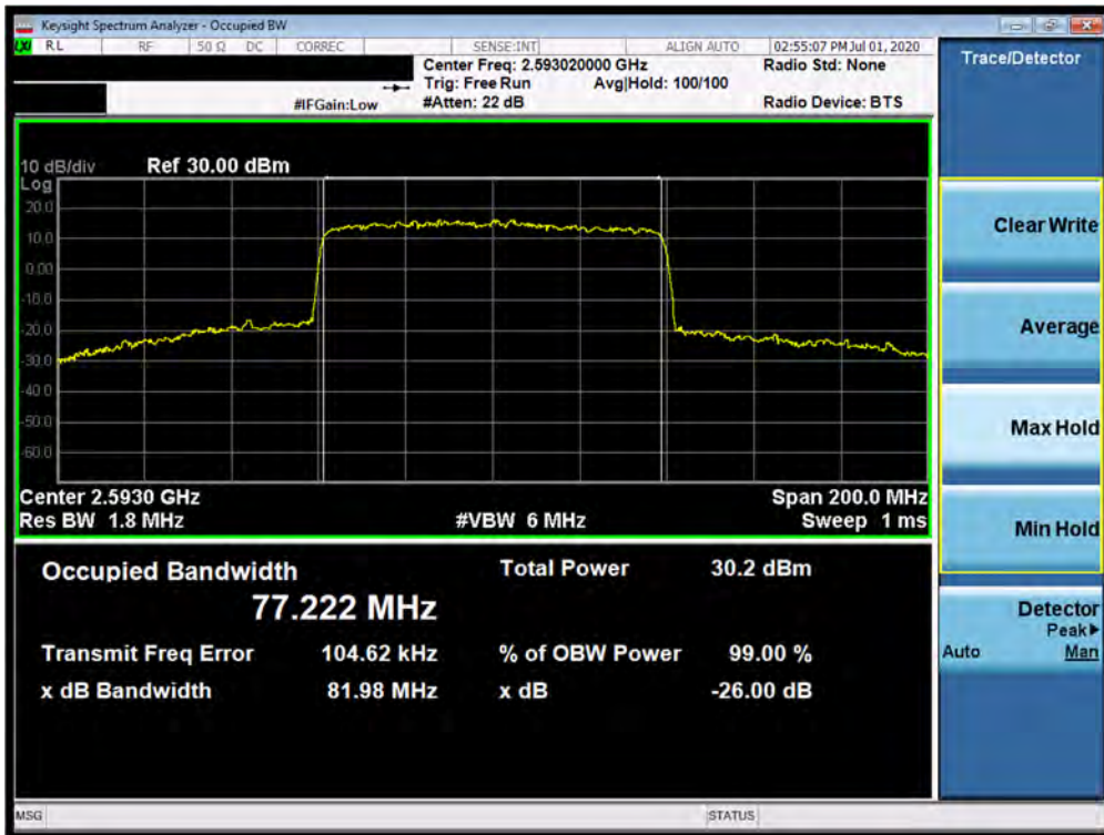
Plot 7-182. Occupied Bandwidth Plot (n41 80MHz QPSK-CP-OFDM - Full RB Configuration)
