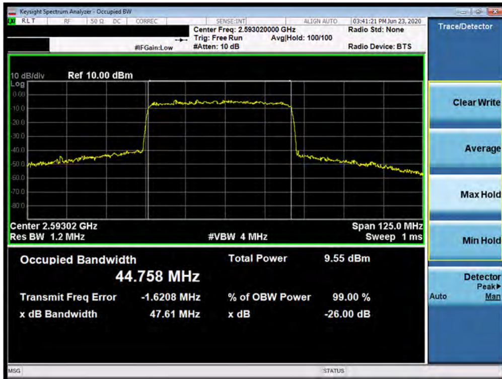
Plot 7-175. Occupied Bandwidth Plot (n41 50MHz 256QAM-CP-OFDM- Full RB Configuration)
