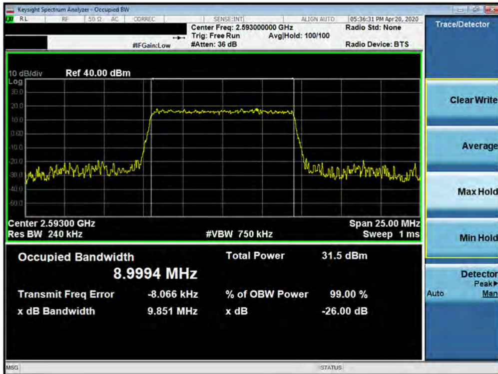
Plot 7-150. Occupied Bandwidth Plot (Band 41 - 10.0MHz 16-QAM - Full RB Configuration)
