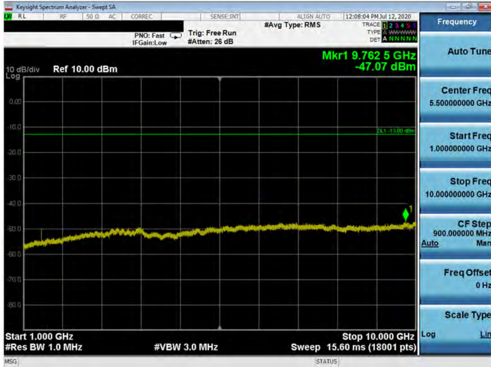
Plot 7-222. Conducted Spurious Plot (Band 12 - 10MHz QPSK - RB Size 1, RB Offset 0 - High Channel)
