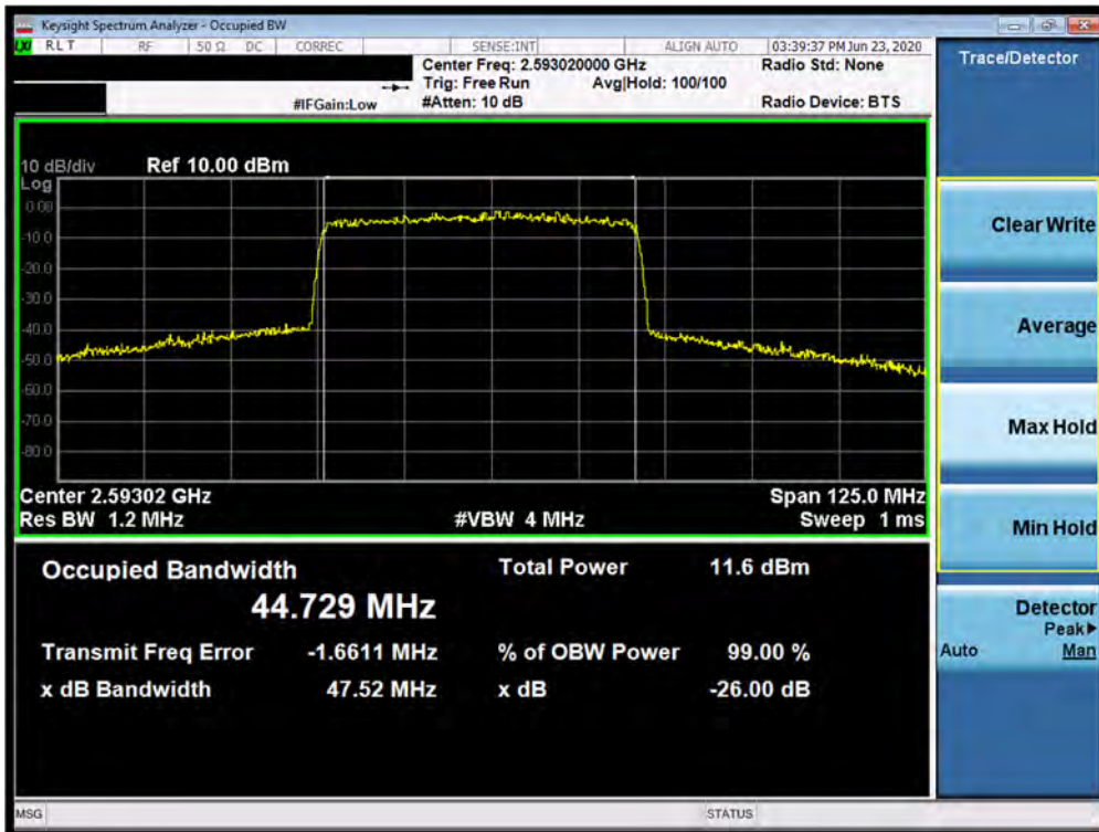
Plot 7-172. Occupied Bandwidth Plot (n41 50MHz QPSK-CP-OFDM - Full RB Configuration)
