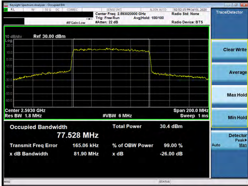
Plot 7-183. Occupied Bandwidth Plot (n41 80MHz 16QAM-CP-OFDM - Full RB Configuration)
