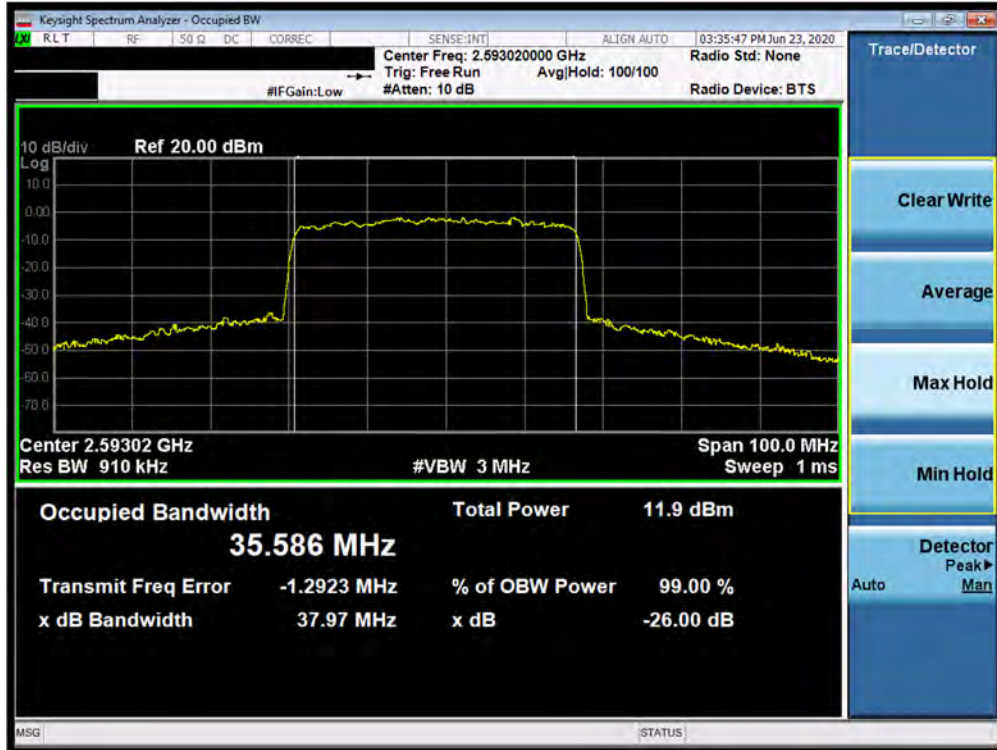
Plot 7-169. Occupied Bandwidth Plot (n41 40MHz 64QAM-CP-OFDM- Full RB Configuration)
