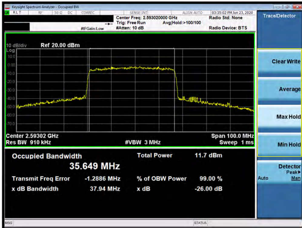
Plot 7-168. Occupied Bandwidth Plot (n41 40MHz 16QAM-CP-OFDM - Full RB Configuration)
