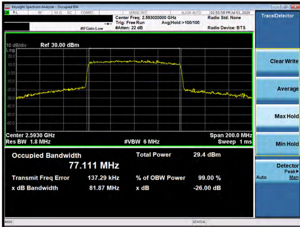
Plot 7-184. Occupied Bandwidth Plot (n41 80MHz 64QAM-CP-OFDM- Full RB Configuration)
