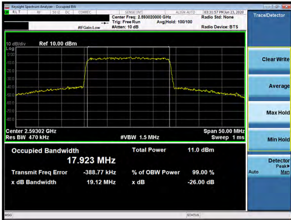
Plot 7-164. Occupied Bandwidth Plot (n41 20MHz 64QAM-CP-OFDM- Full RB Configuration)
