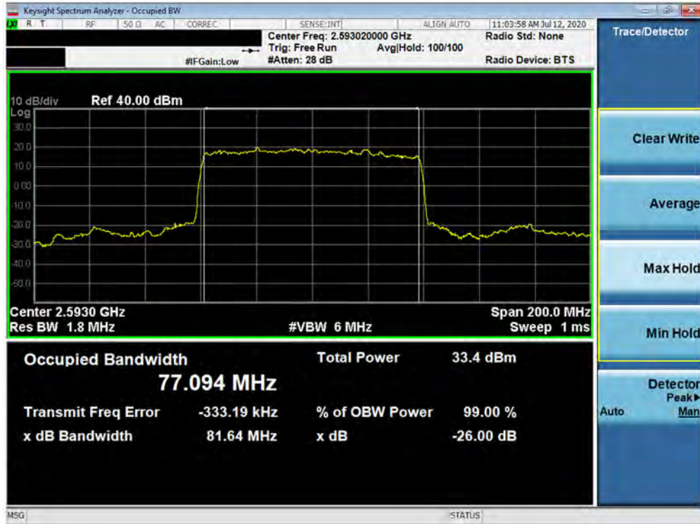
Plot 7-181. Occupied Bandwidth Plot (n41 80MHz BPSK-DFT-s-OFDM - Full RB Configuration)
