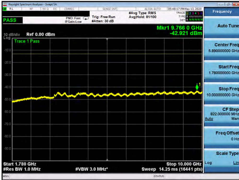
Plot 7-248. Conducted Spurious Plot (n66 - 20MHz DFT-s-OFDM-QPSK - RB Size 1, RB Offset 1 - Mid Channel)
