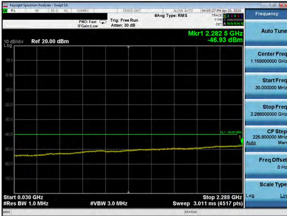
Plot 7-262. Conducted Spurious Plot (Band 30 - 10.0MHz QPSK - RB Size 1, RB Offset 0 - Mid Channel)
