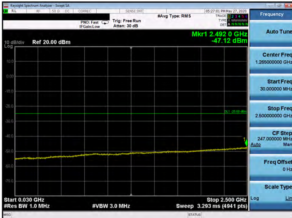
Plot 7-274. Conducted Spurious Plot (Band 7 - 20.0MHz QPSK - RB Size 1, RB Offset 0 - Mid Channel)
