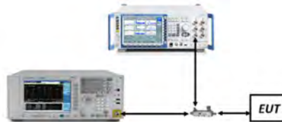
Figure 7-2. Test Instrument & Measurement Setup
