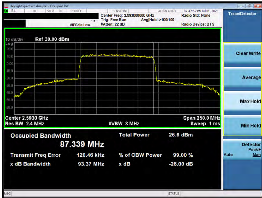
Plot 7-190. Occupied Bandwidth Plot (n41 90MHz 256QAM-CP-OFDM- Full RB Configuration)
