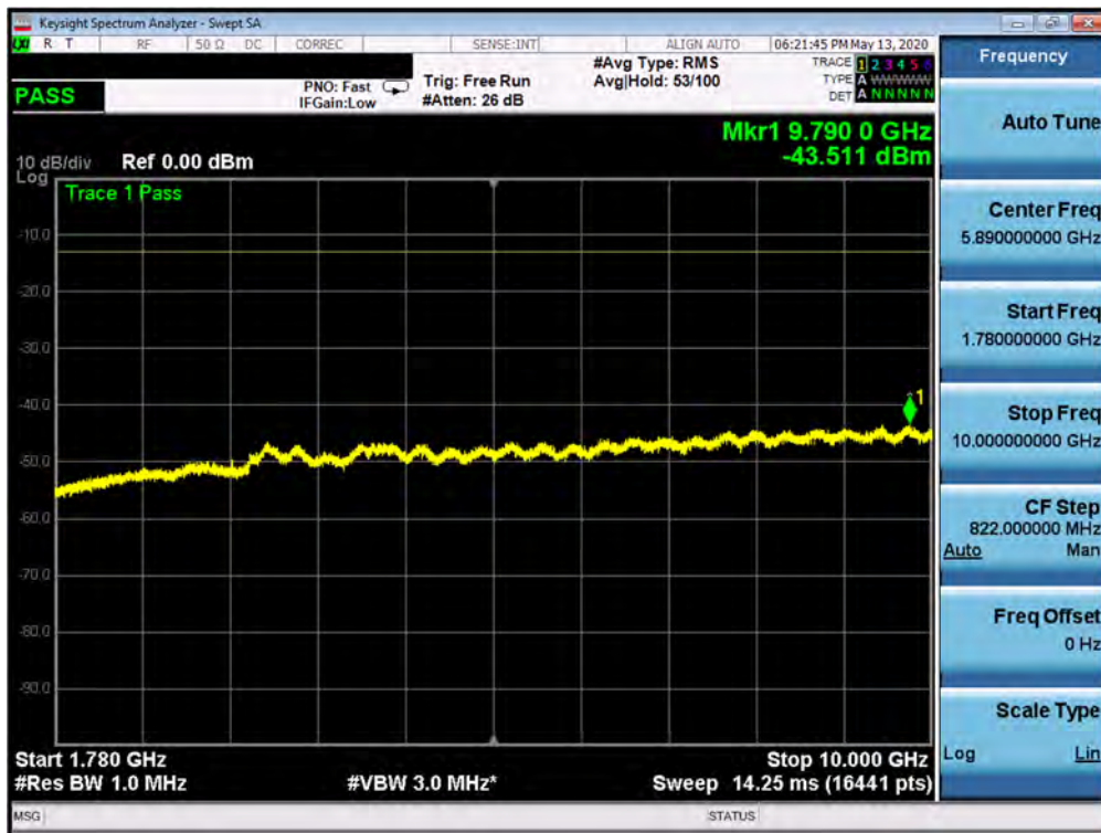
Plot 7-245. Conducted Spurious Plot (n66 - 20MHz DFT-s-OFDM-QPSK - RB Size 1, RB Offset 1 - Low Channel)
