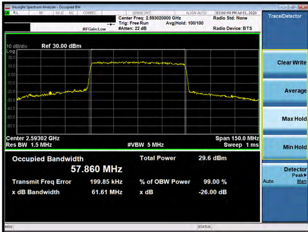
Plot 7-178. Occupied Bandwidth Plot (n41 60MHz 16QAM-CP-OFDM - Full RB Configuration)
