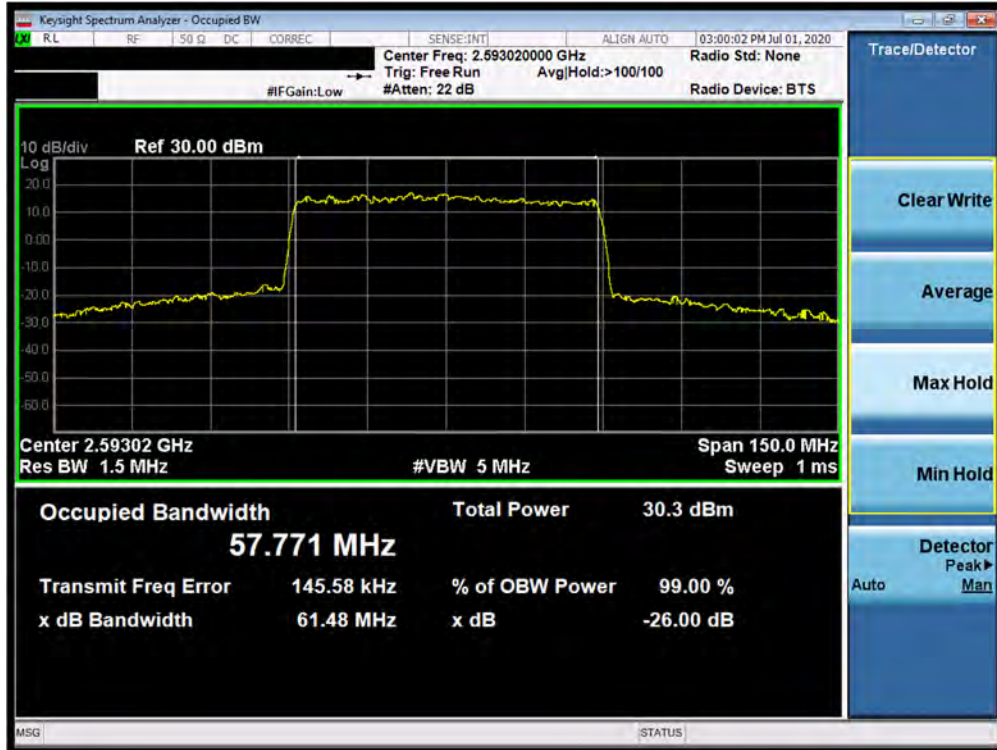
Plot 7-177. Occupied Bandwidth Plot (n41 60MHz QPSK-CP-OFDM - Full RB Configuration)
