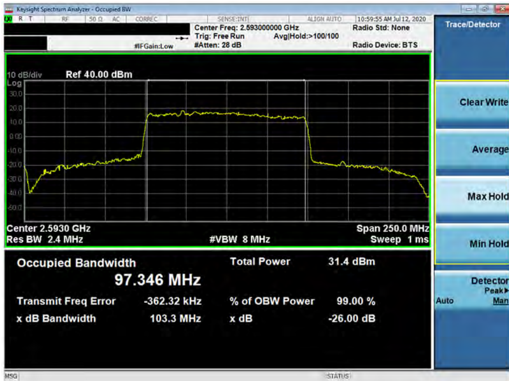
Plot 7-194. Occupied Bandwidth Plot (n41 100MHz 64QAM-CP-OFDM- Full RB Configuration)
