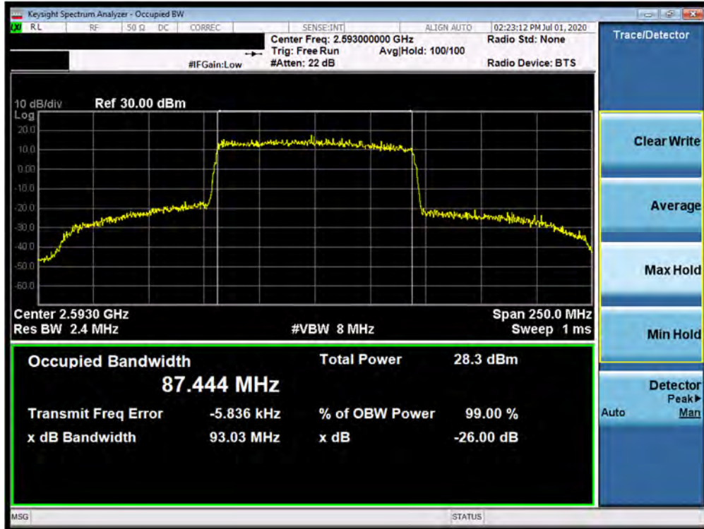
Plot 7-187. Occupied Bandwidth Plot (n41 90MHz QPSK-CP-OFDM - Full RB Configuration)
