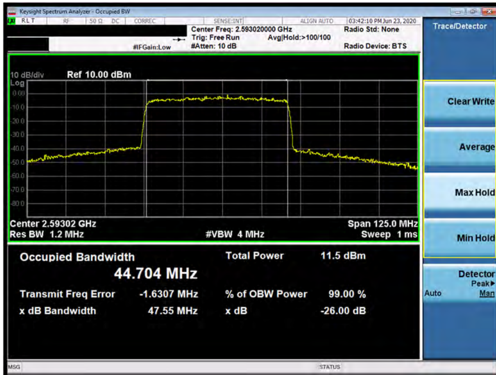
Plot 7-174. Occupied Bandwidth Plot (n41 50MHz 64QAM-CP-OFDM- Full RB Configuration)
