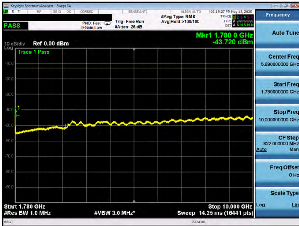
Plot 7-251. Conducted Spurious Plot (n66 - 20MHz DFT-s-OFDM-QPSK - RB Size 1, RB Offset 1 - High Channel)
