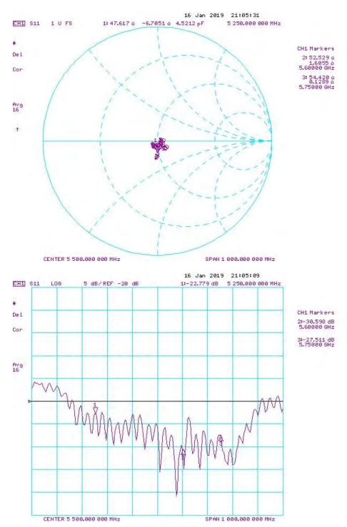
Impedance & Return-Loss Measurement Plot for Head TSL
