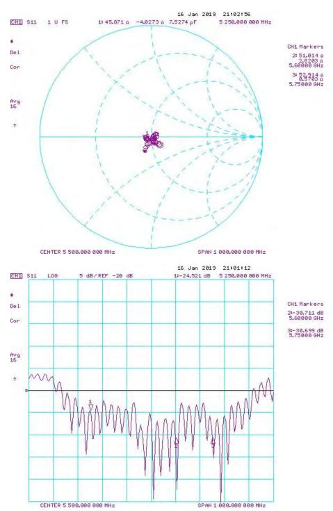
Impedance & Return-Loss Measurement Plot for Body TSL
