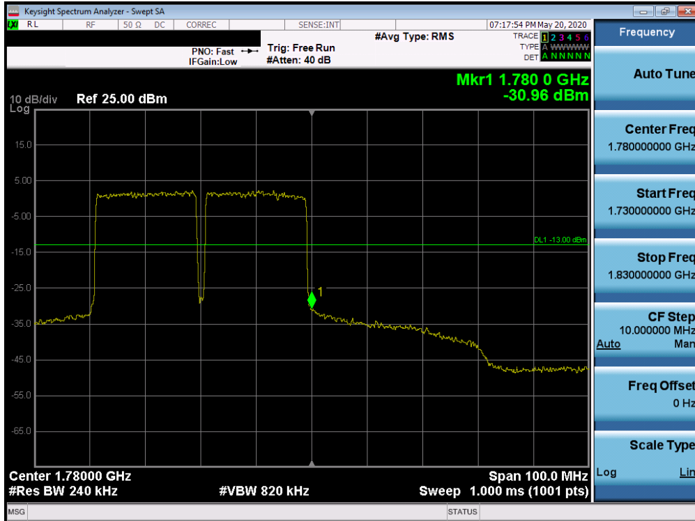
Plot 7-730. Upper Band Edge Plot (Band 66 QPSK – PCC:20 MHz SCC:20 MHz – Full RB)
