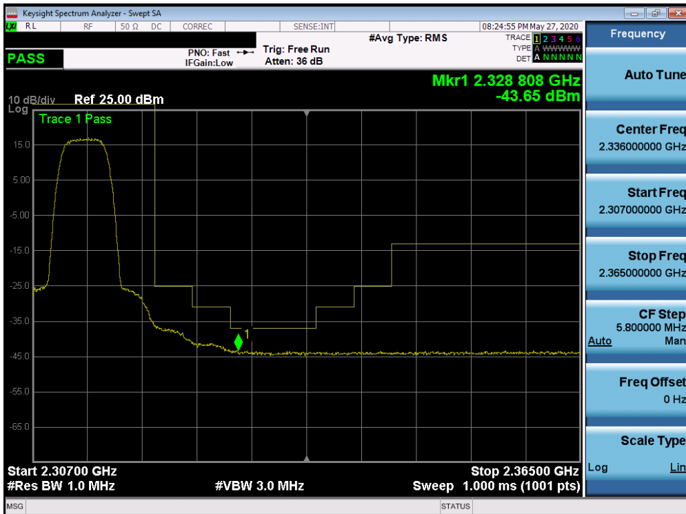
Plot 7-579. Upper Extended Band Edge Plot (Band 30 - 5.0MHz QPSK - Full RB Configuration)
