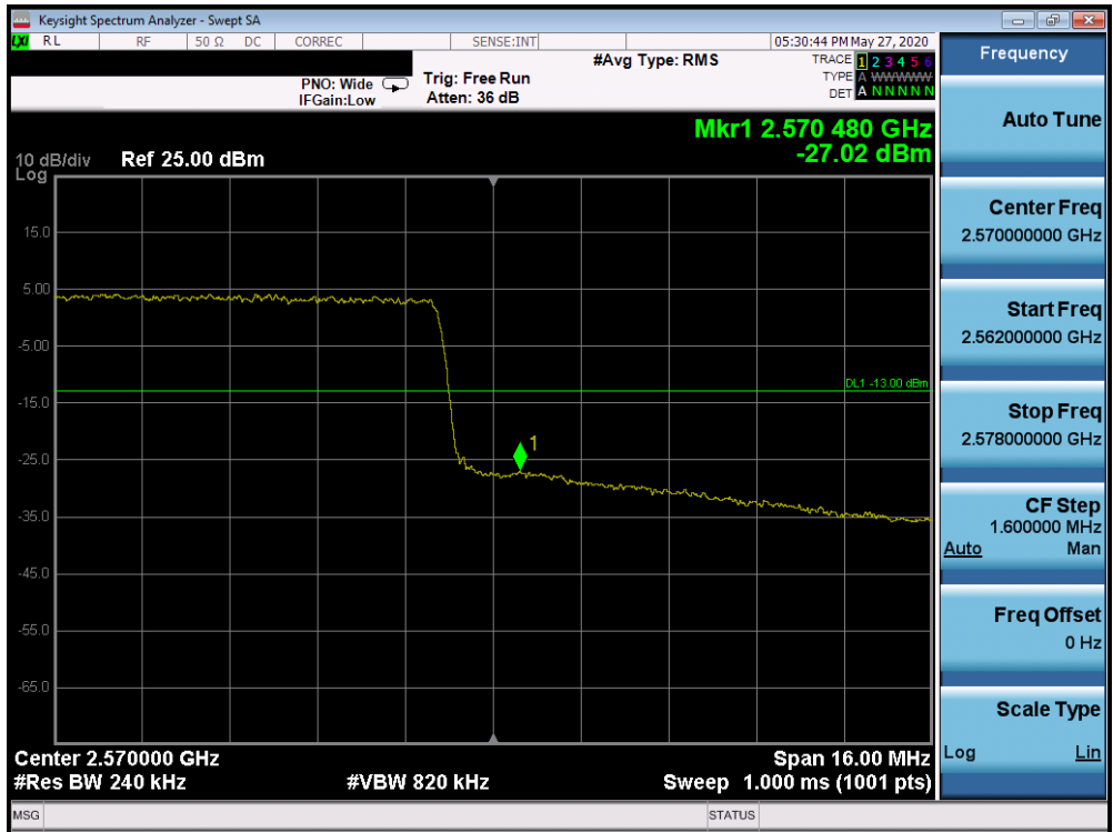
Plot 7-598. Upper Band Edge Plot (Band 7 - 20.0MHz QPSK - Full RB Configuration)
