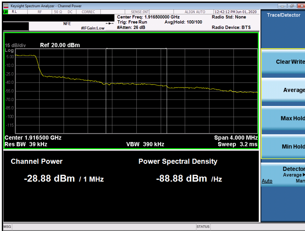
Plot 7-519. Upper Extended Band Edge Plot (Band 25 - 1.4MHz QPSK - Full RB Configuration)
