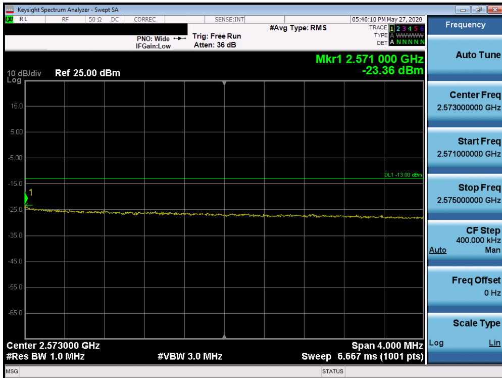
Plot 7-591. Upper Extended Band Edge Plot (Band 7 - 10.0MHz QPSK - Full RB Configuration)
