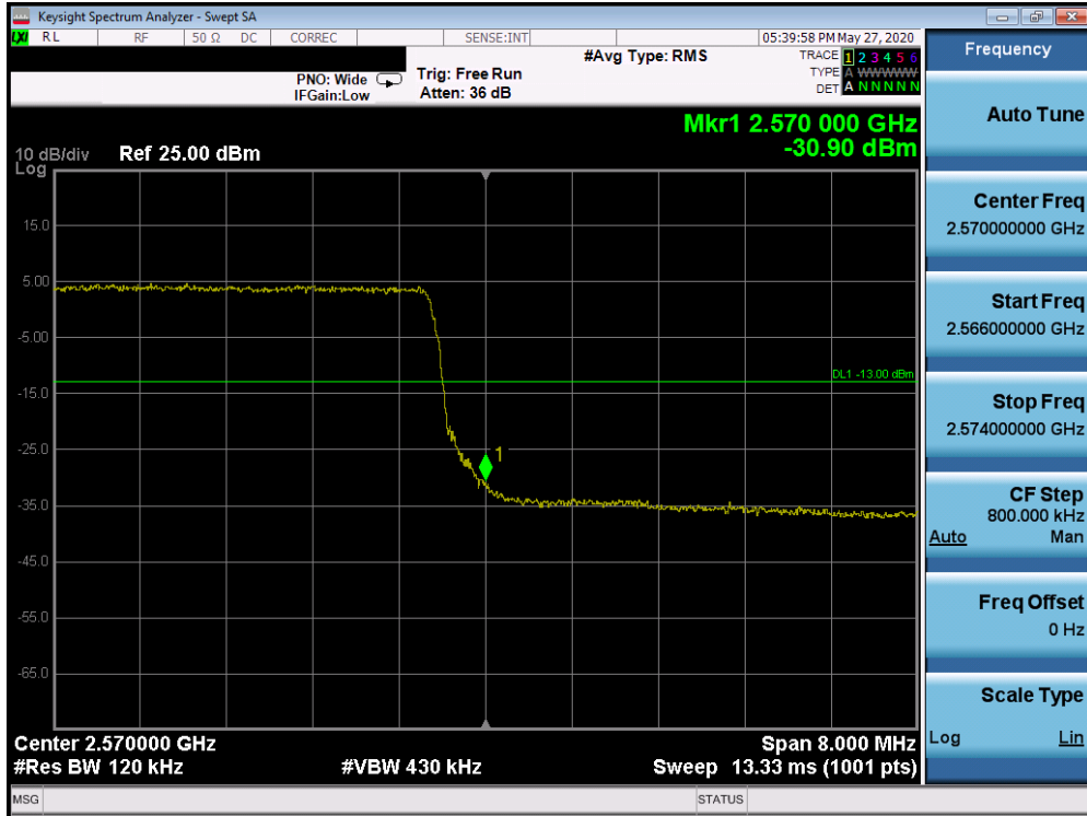
Plot 7-590. Upper Band Edge Plot (Band 7 - 10.0MHz QPSK - Full RB Configuration)
