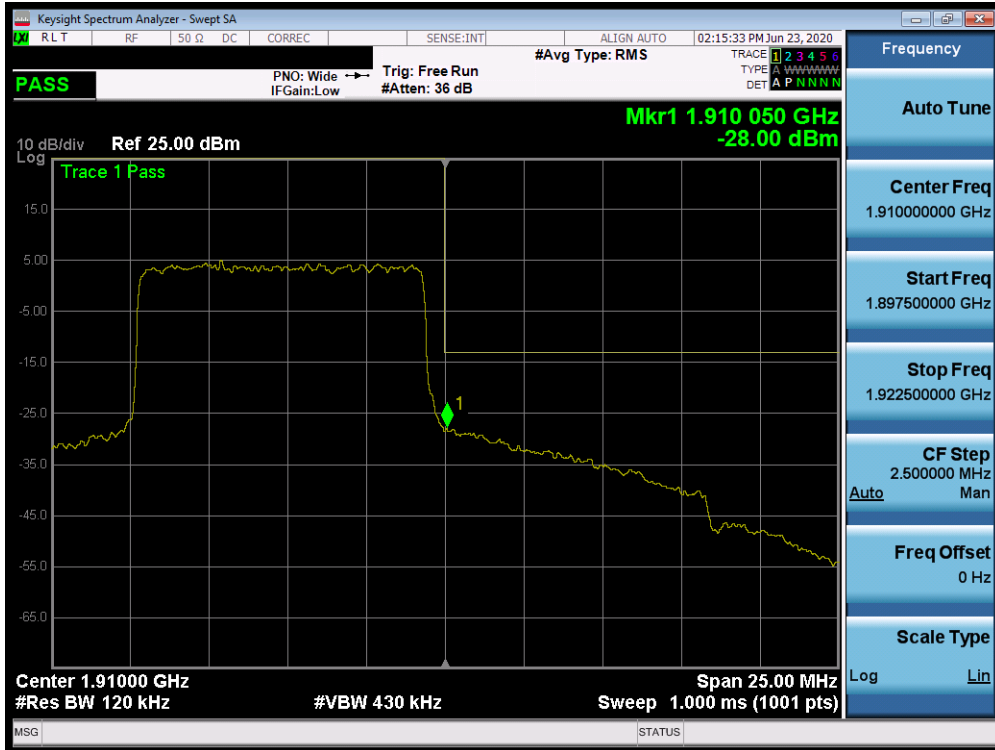
Plot 7-558. Upper Band Edge Plot (n2 - 10MHz DFT-s-OFDM-QPSK - Full RB Configuration)
