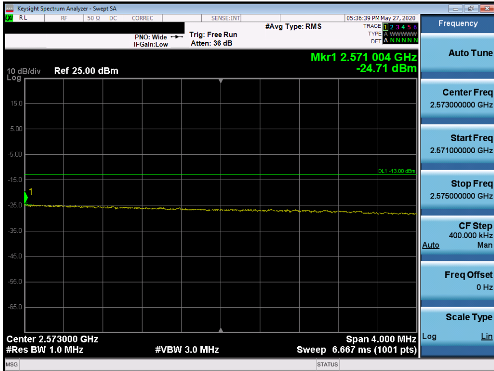
Plot 7-595. Upper Extended Band Edge Plot (Band 7 - 15.0MHz QPSK - Full RB Configuration)
