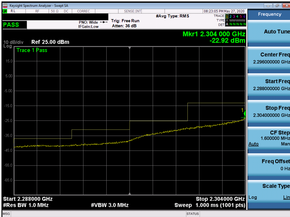
Plot 7-581. Lower Extended Band Edge Plot (Band 30 - 10.0MHz QPSK - Full RB Configuration)
