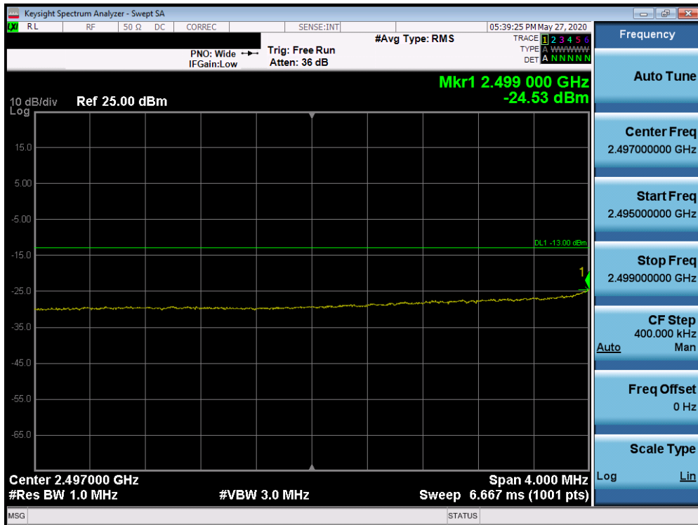
Plot 7-589. Lower Extended Band Edge Plot (Band 7 - 10.0MHz QPSK - Full RB Configuration)
