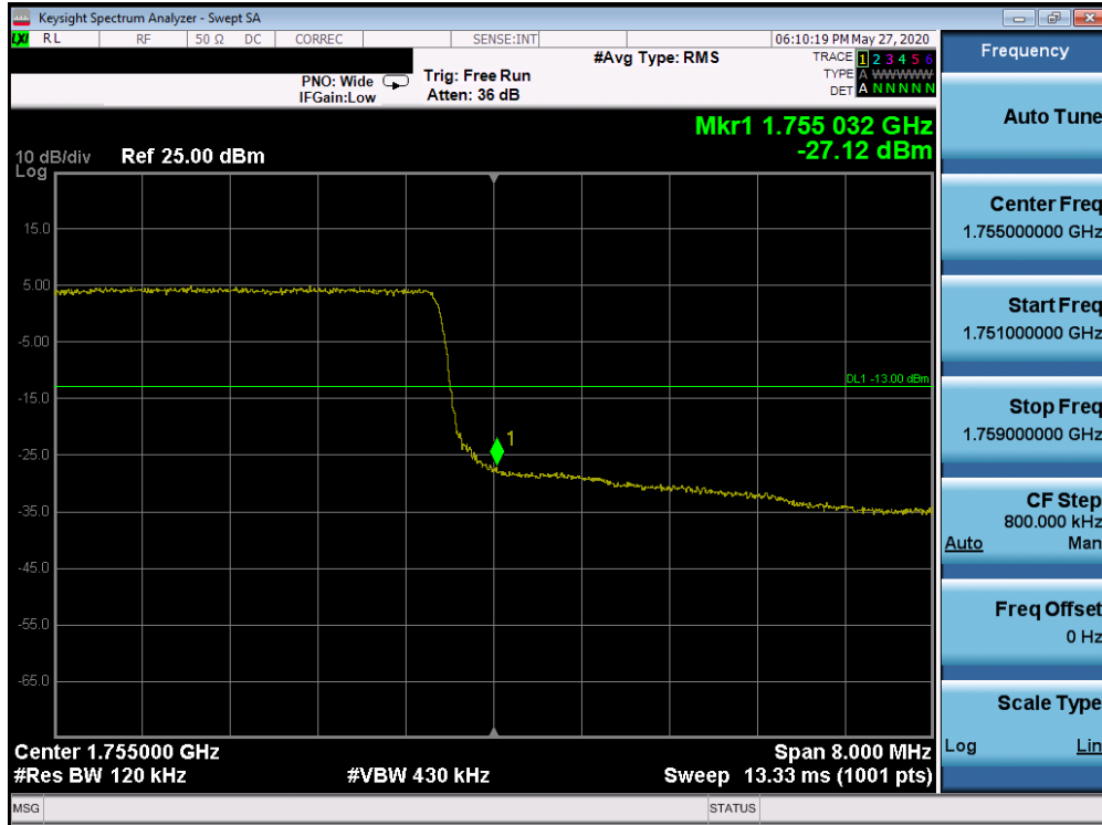
Plot 7-484. Upper Band Edge Plot (Band 4 - 10.0MHz QPSK - Full RB Configuration)
