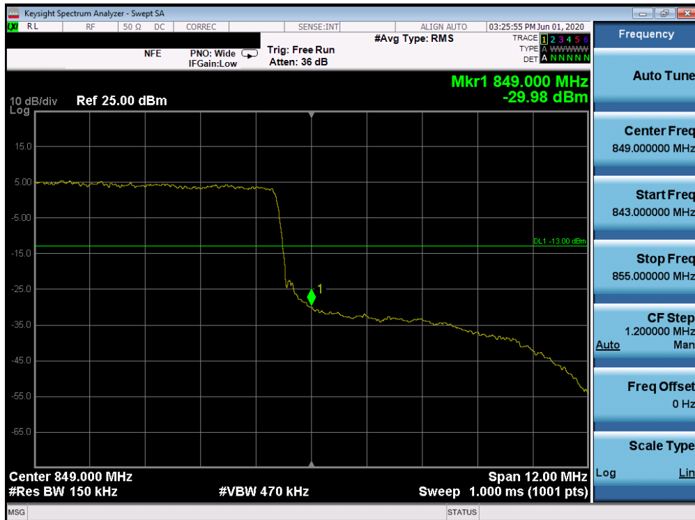
Plot 7-455. Upper Band Edge Plot (Band 26 - 15.0MHz QPSK - Full RB Configuration)
