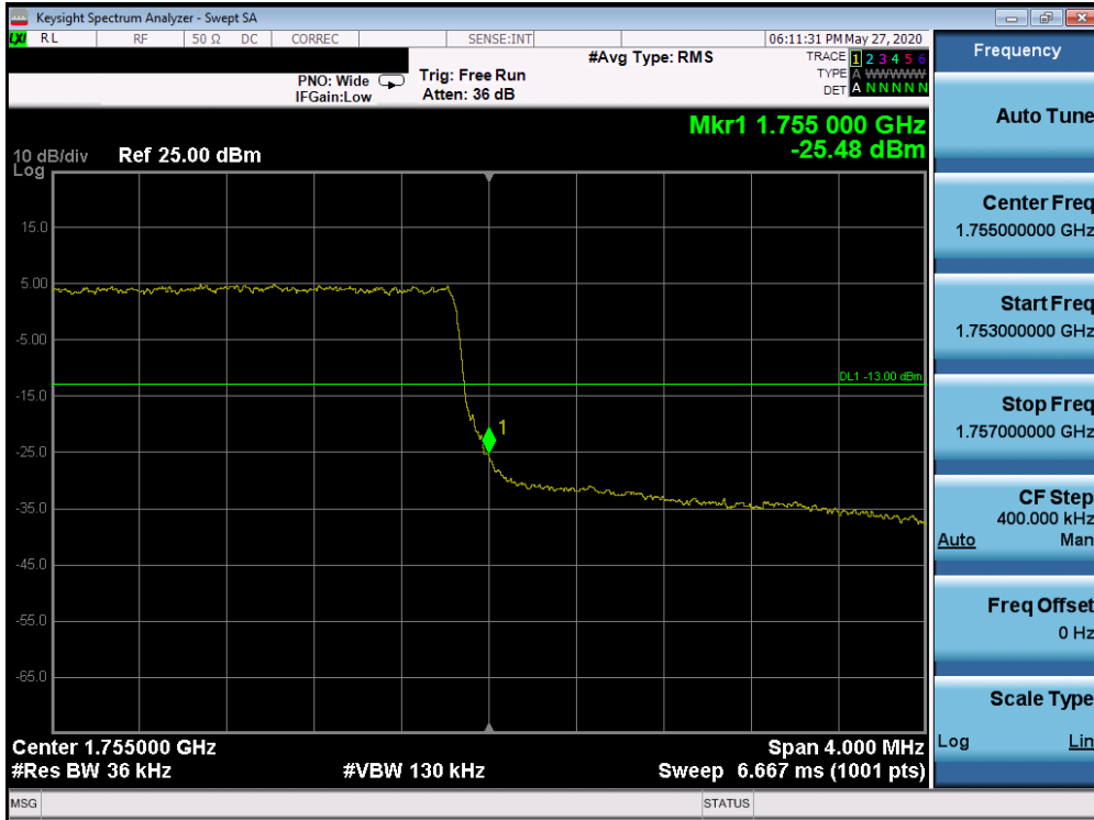
Plot 7-472. Upper Band Edge Plot (Band 4 - 3.0MHz QPSK - Full RB Configuration)
