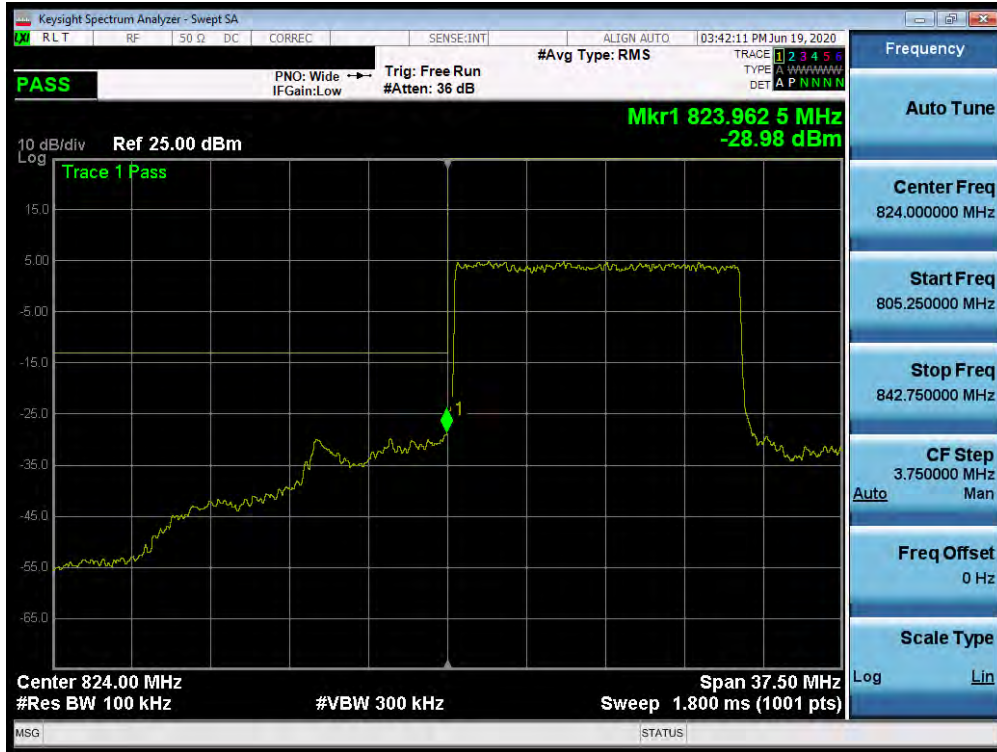
Plot 7-460. Lower Band Edge Plot (n5 – 15.0MHz DFT-s-OFDM BPSK - Full RB Configuration)
