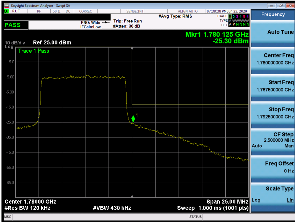
Plot 7-504. Upper Band Edge Plot (n66 - 10MHz DFT-s-OFDM-QPSK - Full RB Configuration)
