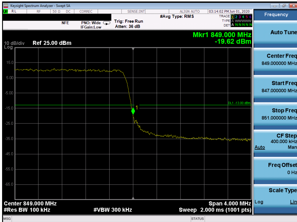
Plot 7-449. Upper Band Edge Plot (Band 26/5 - 3.0MHz QPSK - Full RB Configuration)
