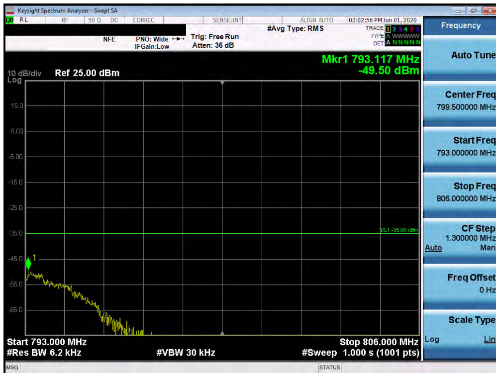
Plot 7-445. Upper Band Emission Mask Plot (Band 13 - 10.0MHz QPSK - Full RB Configuration)
