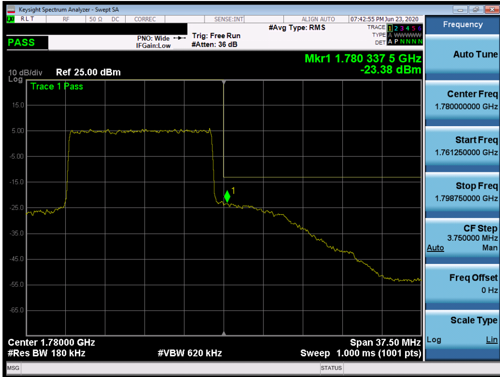
Plot 7-508. Upper Band Edge Plot (n66 - 15MHz DFT-s-OFDM-QPSK - Full RB Configuration)
