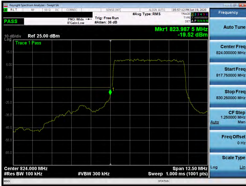
Plot 7-456. Lower Band Edge Plot (n5 – 5.0MHz DFT-s-OFDM BPSK - Full RB Configuration)
