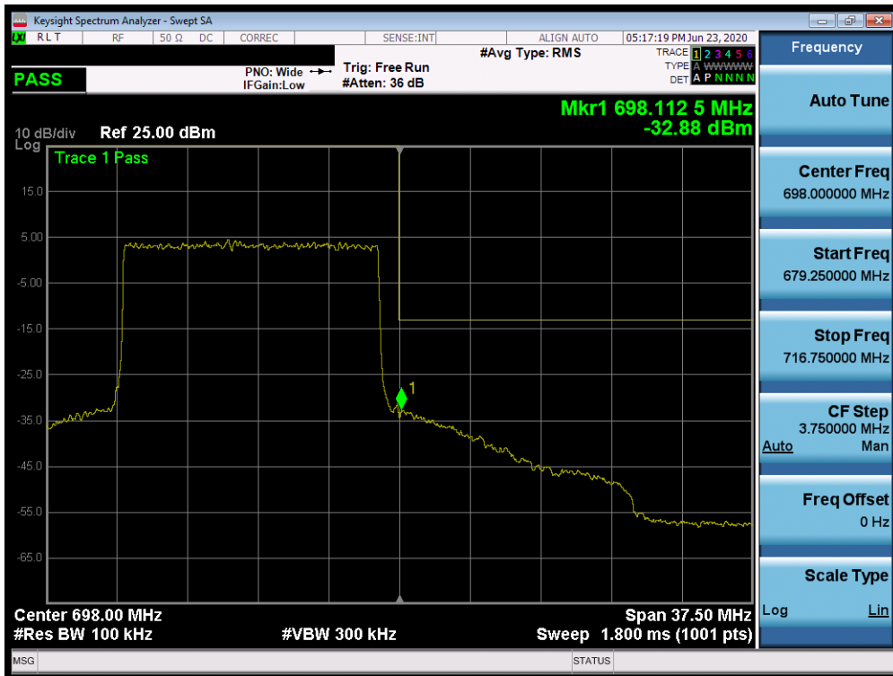
Plot 7-421. Upper Band Edge Plot (n71 - 15MHz DFT-s-OFDM-QPSK - Full RB Configuration)
