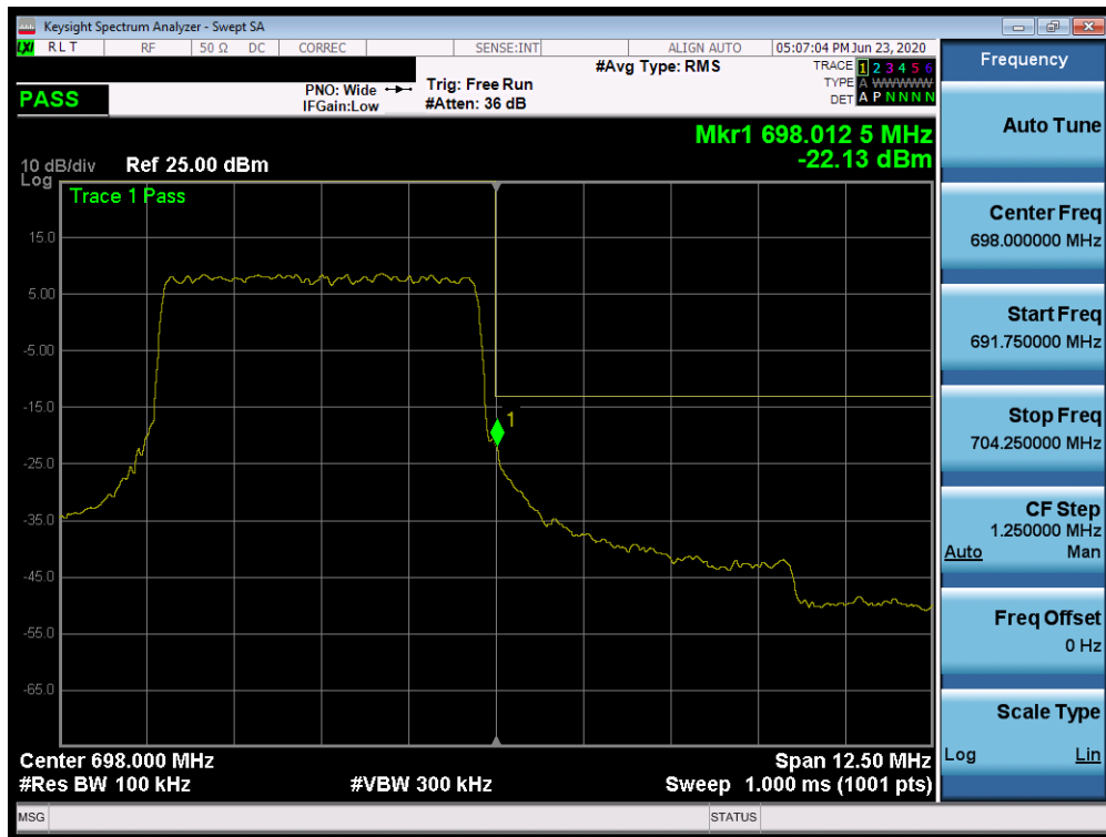
Plot 7-417. Upper Band Edge Plot (n71 - 5MHz DFT-s-OFDM-QPSK - Full RB Configuration)
