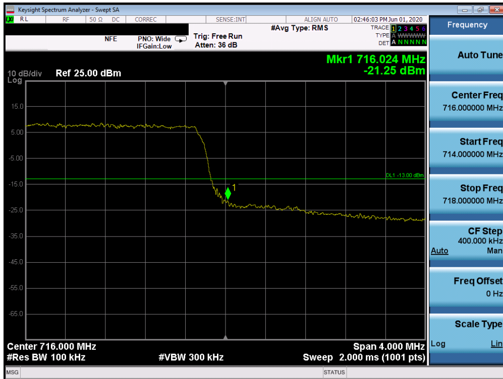
Plot 7-429. Upper Band Edge Plot (Band 12 - 5.0MHz QPSK - Full RB Configuration)
