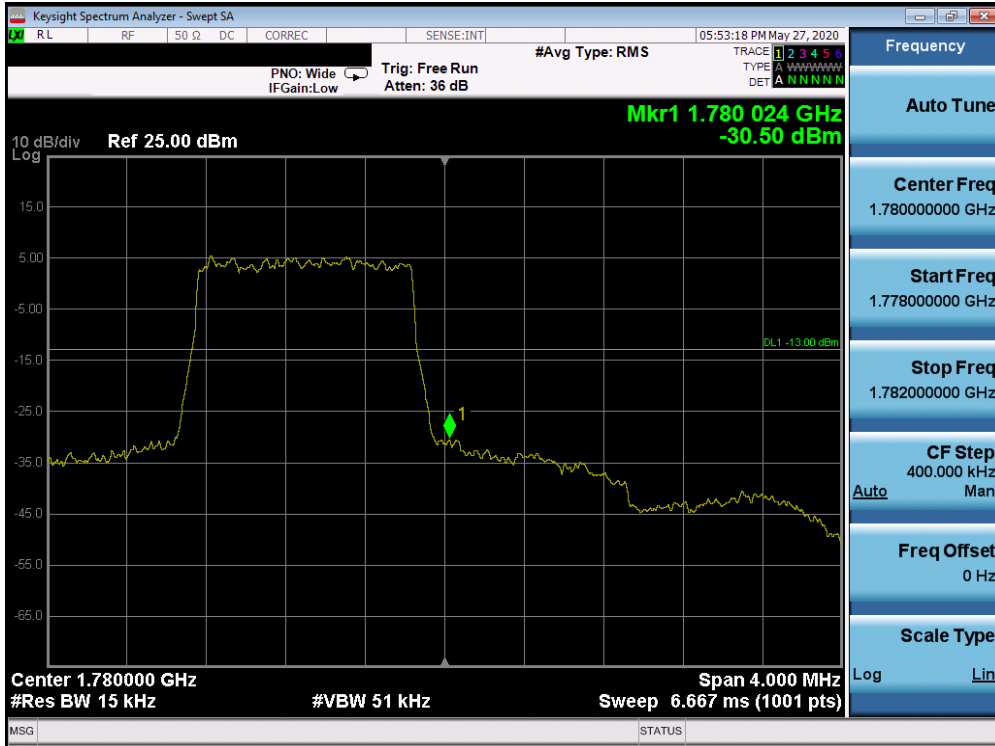
Plot 7-468. Upper Band Edge Plot (Band 66 - 1.4MHz QPSK - Full RB Configuration)
