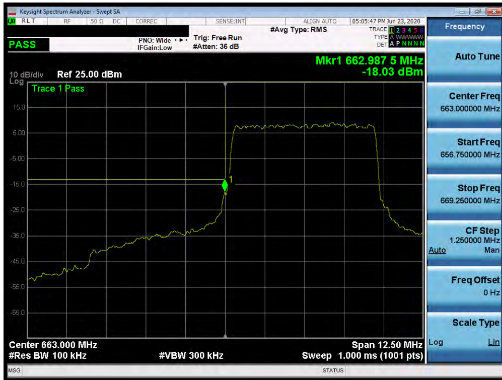
Plot 7-416. Lower Band Edge Plot (n71 - 5MHz DFT-s-OFDM-QPSK - Full RB Configuration)
