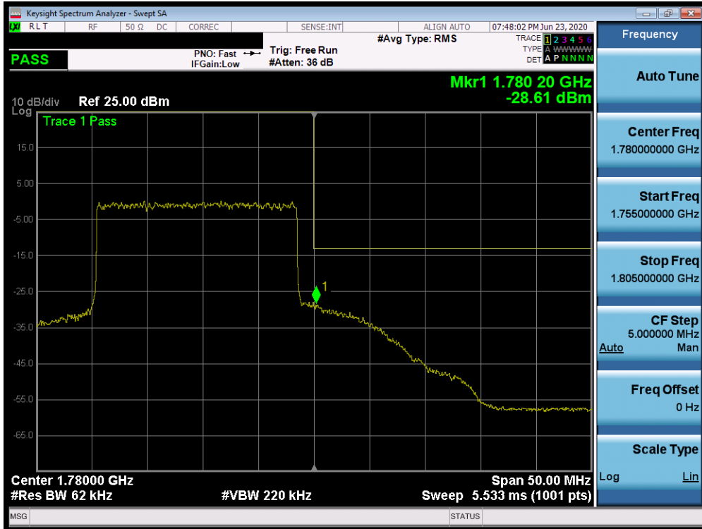
Plot 7-512. Upper Band Edge Plot (n66 - 20MHz DFT-s-OFDM-QPSK - Full RB Configuration)
