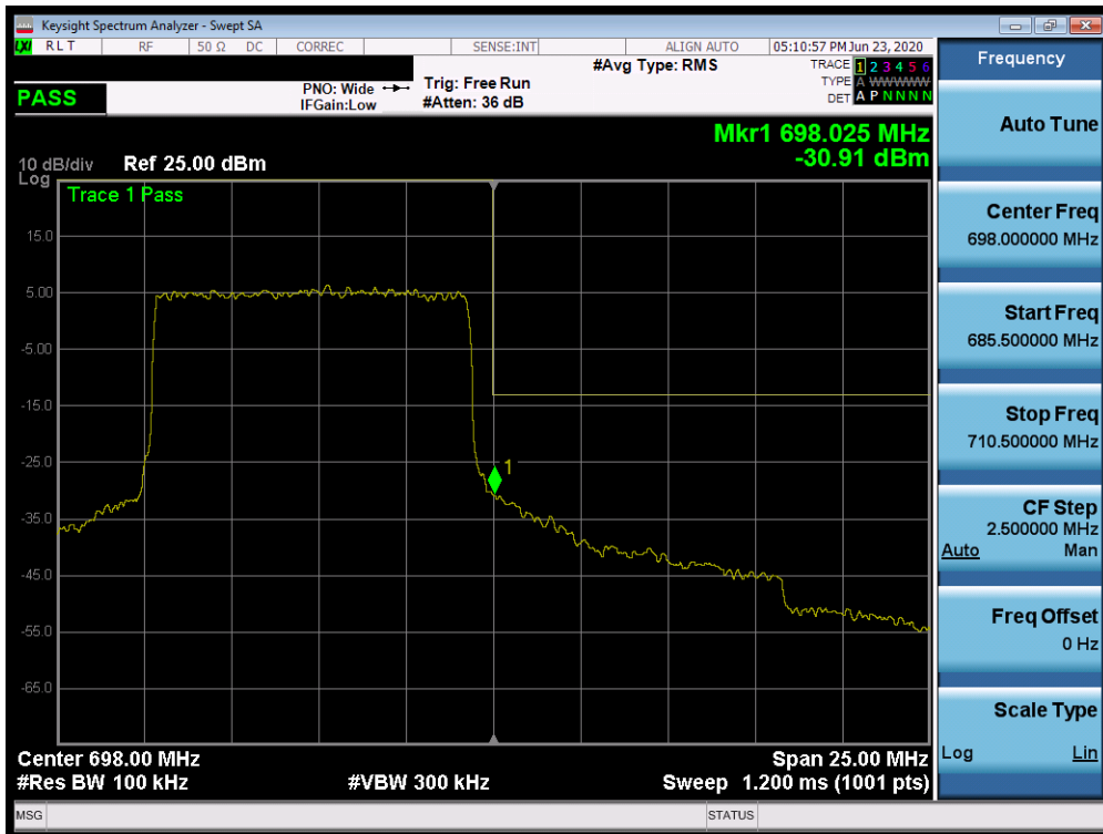
Plot 7-419. Upper Band Edge Plot (n71 - 10MHz DFT-s-OFDM-QPSK - Full RB Configuration)
