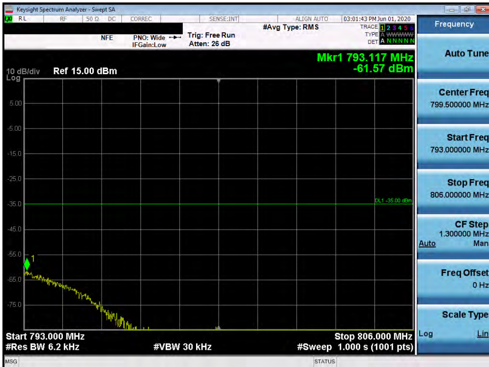
Plot 7-441. Upper Emission Mask Plot (Band 13 - 5.0MHz QPSK - Full RB Configuration)
