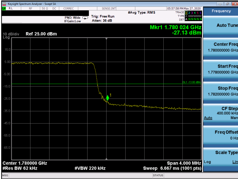
Plot 7-480. Upper Band Edge Plot (Band 66 - 5.0MHz QPSK - Full RB Configuration)
