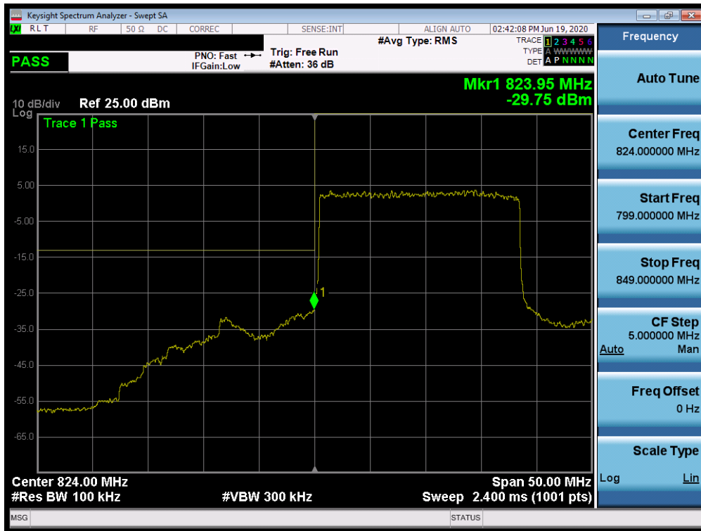
Plot 7-462. Lower Band Edge Plot (n5 – 20.0MHz DFT-s-OFDM BPSK - Full RB Configuration)
