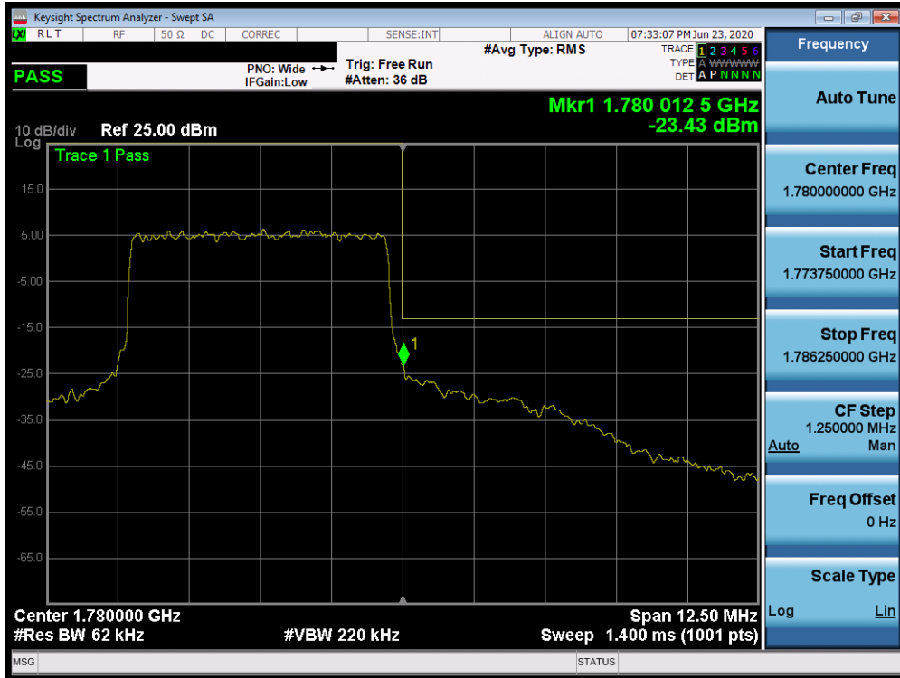
Plot 7-500. Upper Band Edge Plot (n66 - 5MHz DFT-s-OFDM-QPSK - Full RB Configuration)
