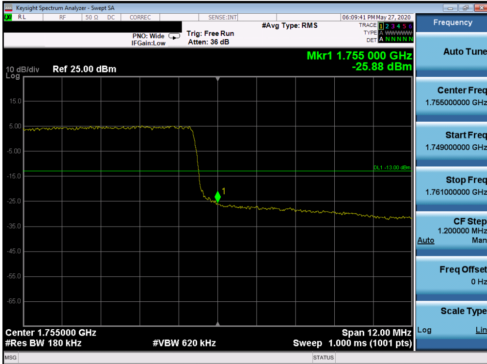
Plot 7-490. Upper Band Edge Plot (Band 4 - 15.0MHz QPSK - Full RB Configuration)
