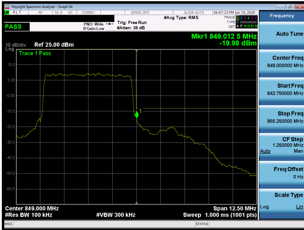
Plot 7-457. Upper Band Edge Plot (n5 – 5.0MHz DFT-s-OFDM BPSK - Full RB Configuration)
