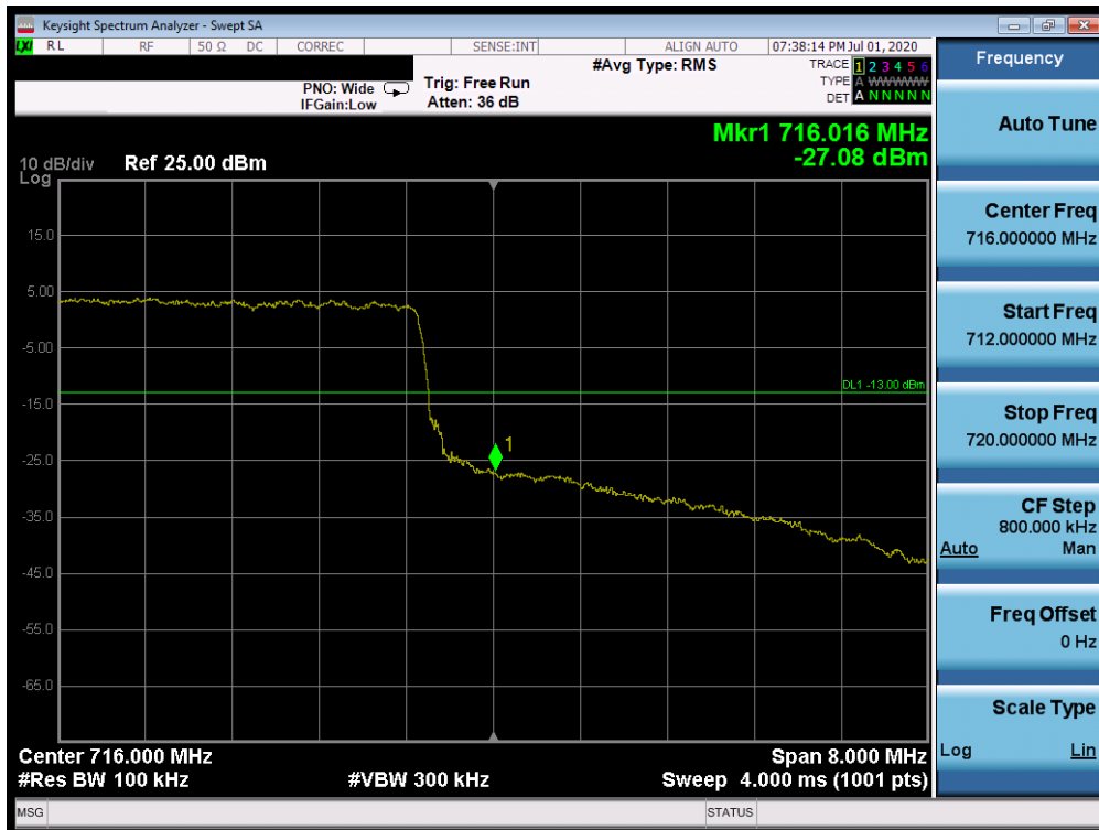
Plot 7-435. Upper Band Edge Plot (n12 - 10MHz DFT-s-OFDM-QPSK - Full RB Configuration)
