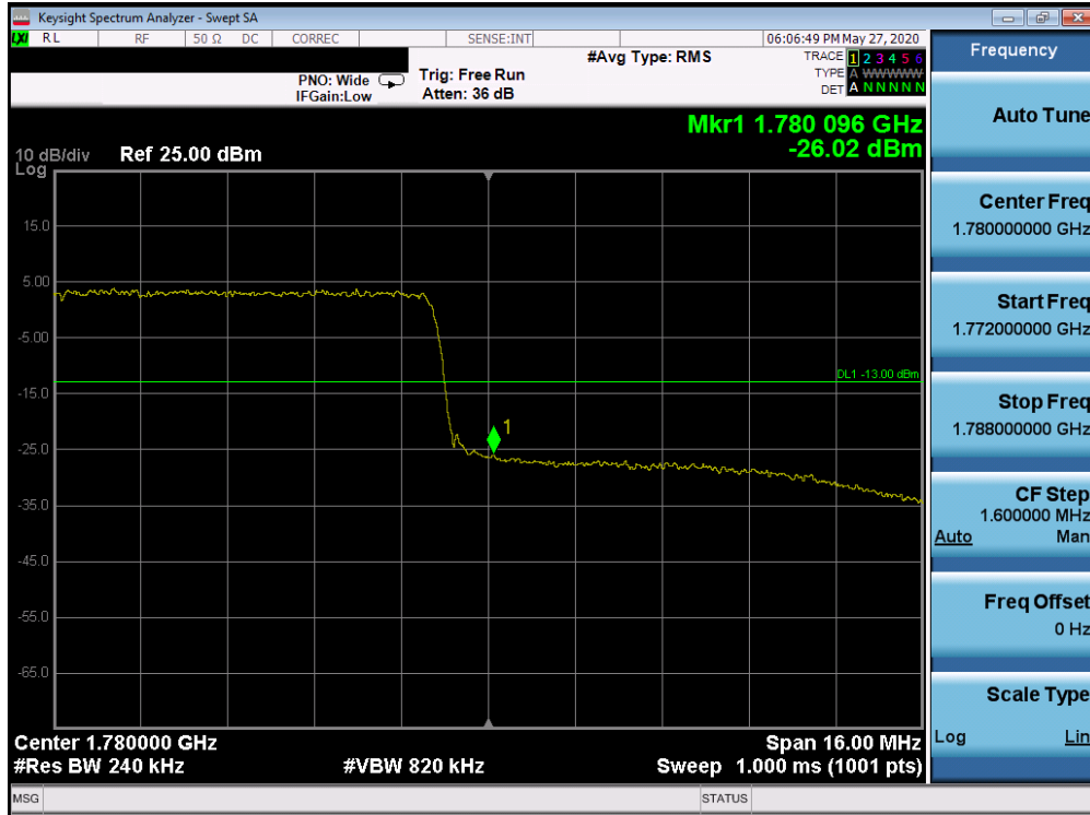
Plot 7-496. Upper Band Edge Plot (Band 66 - 20.0MHz QPSK - Full RB Configuration)
