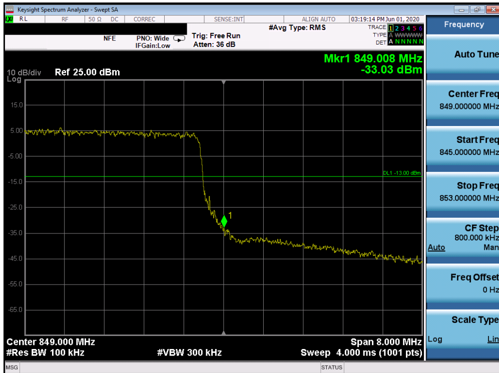
Plot 7-453. Upper Band Edge Plot (Band 26/5 - 10.0MHz QPSK - Full RB Configuration)
