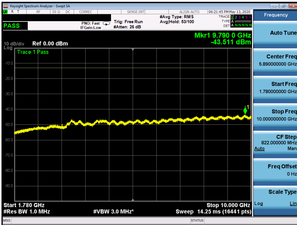
Plot 7-346. Conducted Spurious Plot (n66 - 20MHz DFT-s-OFDM-QPSK - RB Size 1, RB Offset 1 - Low Channel)
