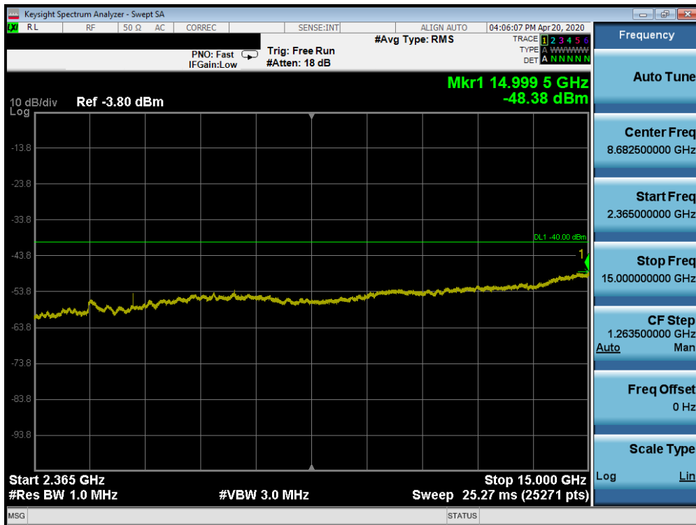
Plot 7-373. Conducted Spurious Plot (Band 30 - 10.0MHz QPSK - RB Size 1, RB Offset 0 - Mid Channel)
