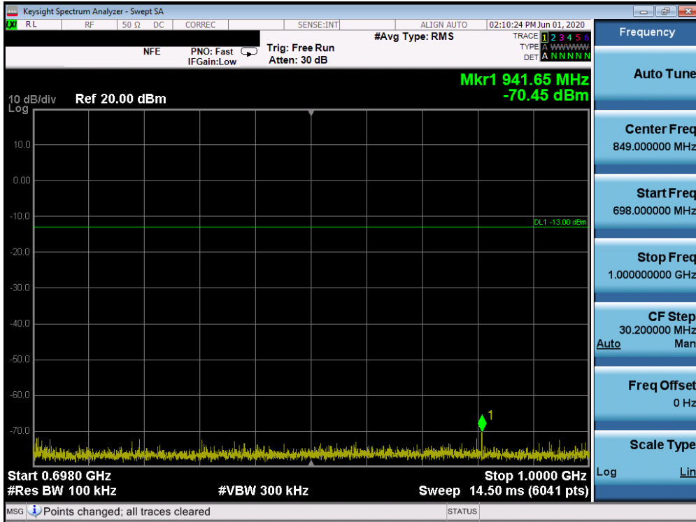
Plot 7-283. Conducted Spurious Plot (Band 71 - 20.0MHz QPSK - RB Size 1, RB Offset 0 - Mid Channel)
