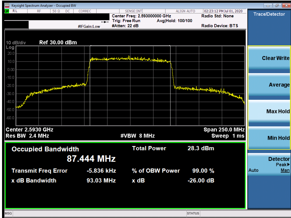
Plot 7-270. Occupied Bandwidth Plot (n41 90MHz QPSK-CP-OFDM - Full RB Configuration)
