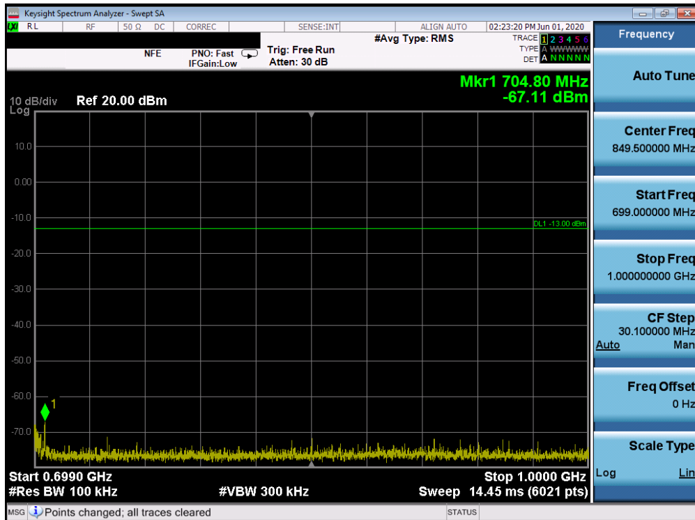
Plot 7-286. Conducted Spurious Plot (Band 71 - 20.0MHz QPSK - RB Size 1, RB Offset 0 - High Channel)
