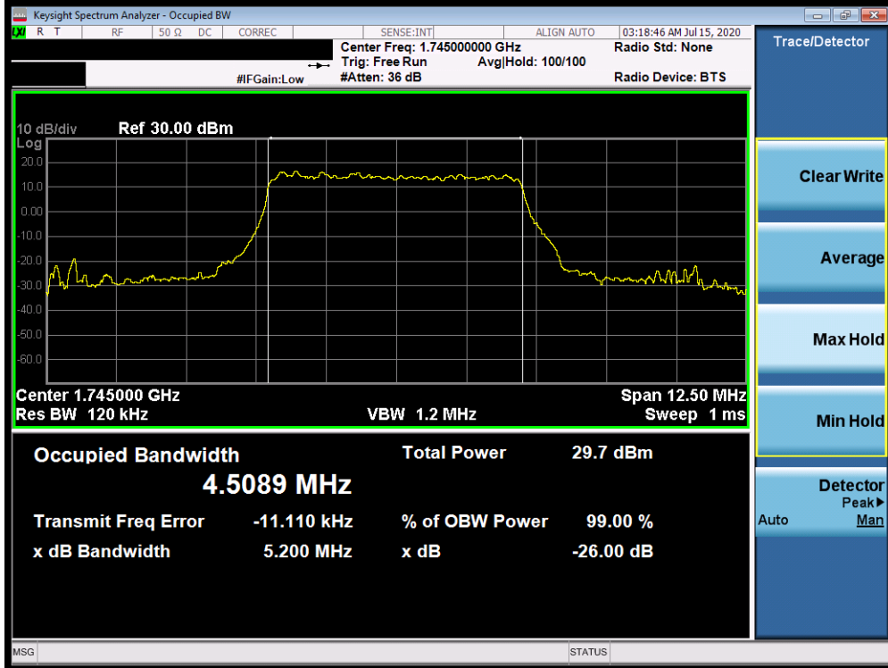
Plot 7-142. Occupied Bandwidth Plot (n66 5MHz 16QAM-CP-OFDM - Full RB Configuration)
