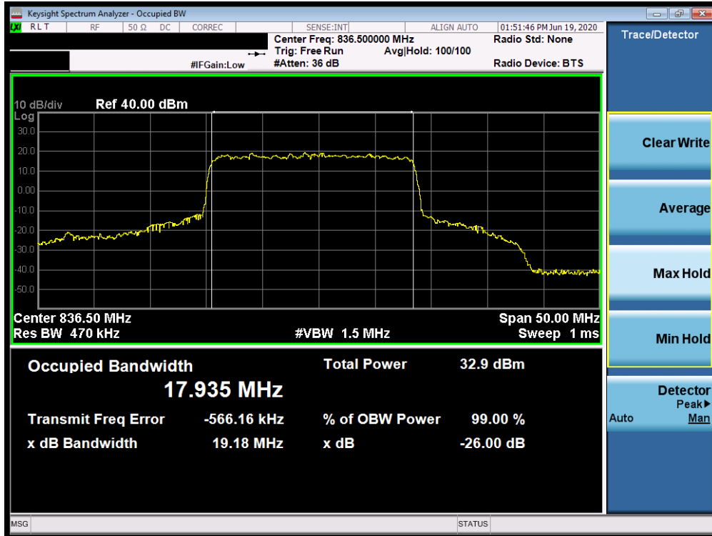
Plot 7-112. Occupied Bandwidth Plot (n5 20MHz QPSK-CP-OFDM - Full RB Configuration)
