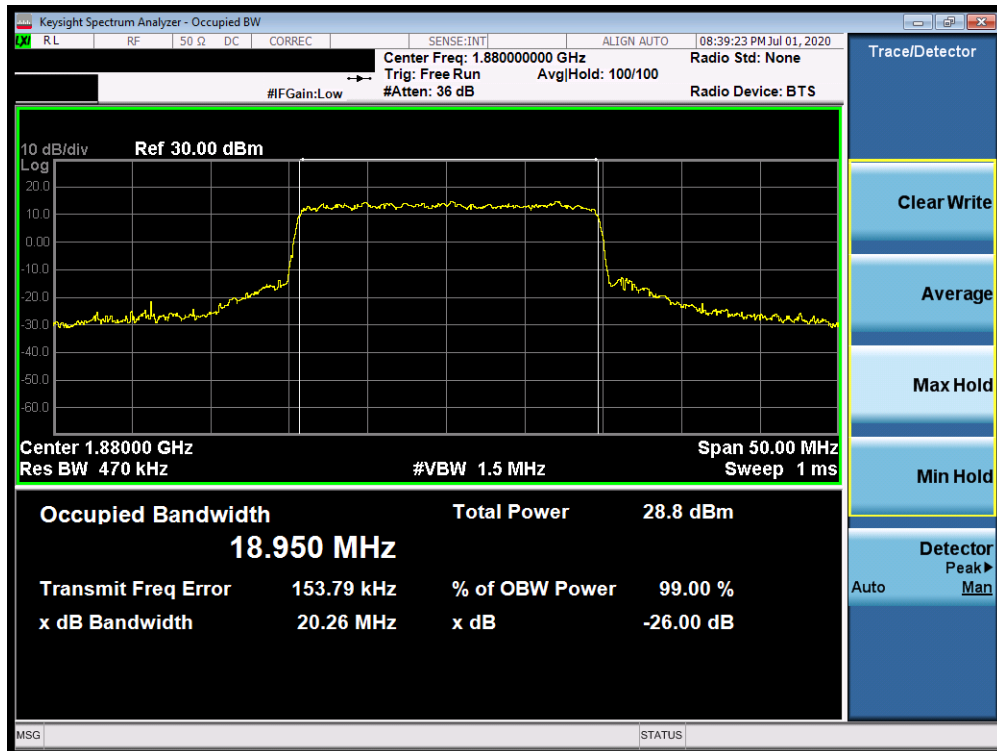
Plot 7-200. Occupied Bandwidth Plot (n25/2 20MHz QPSK-CP-OFDM - Full RB Configuration)
