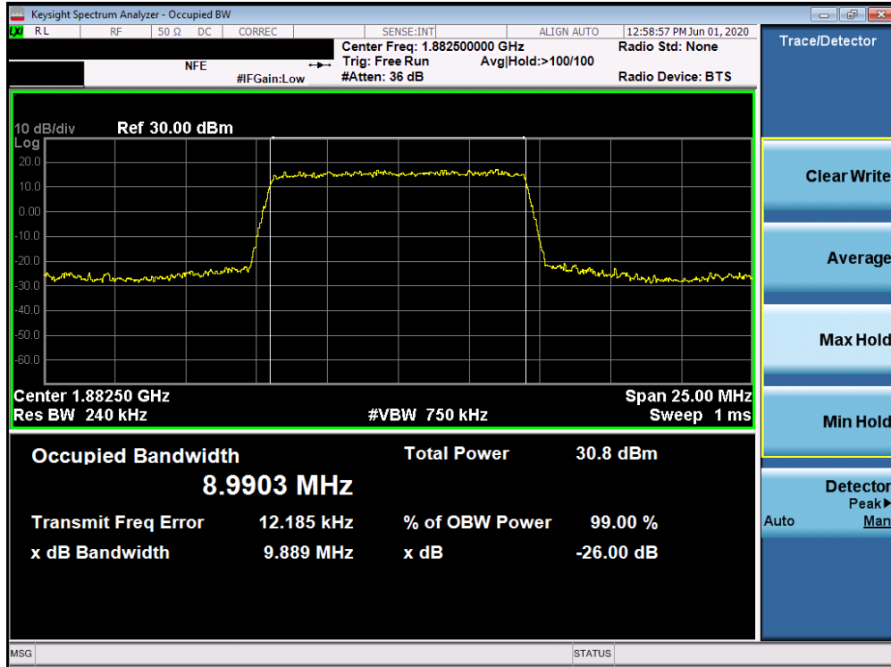
Plot 7-172. Occupied Bandwidth Plot (Band 25/2 - 10.0MHz QPSK - Full RB Configuration)
