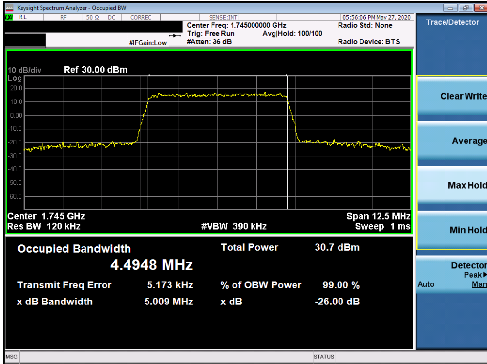
Plot 7-124. Occupied Bandwidth Plot (Band 66/4 - 5.0MHz QPSK - Full RB Configuration)
