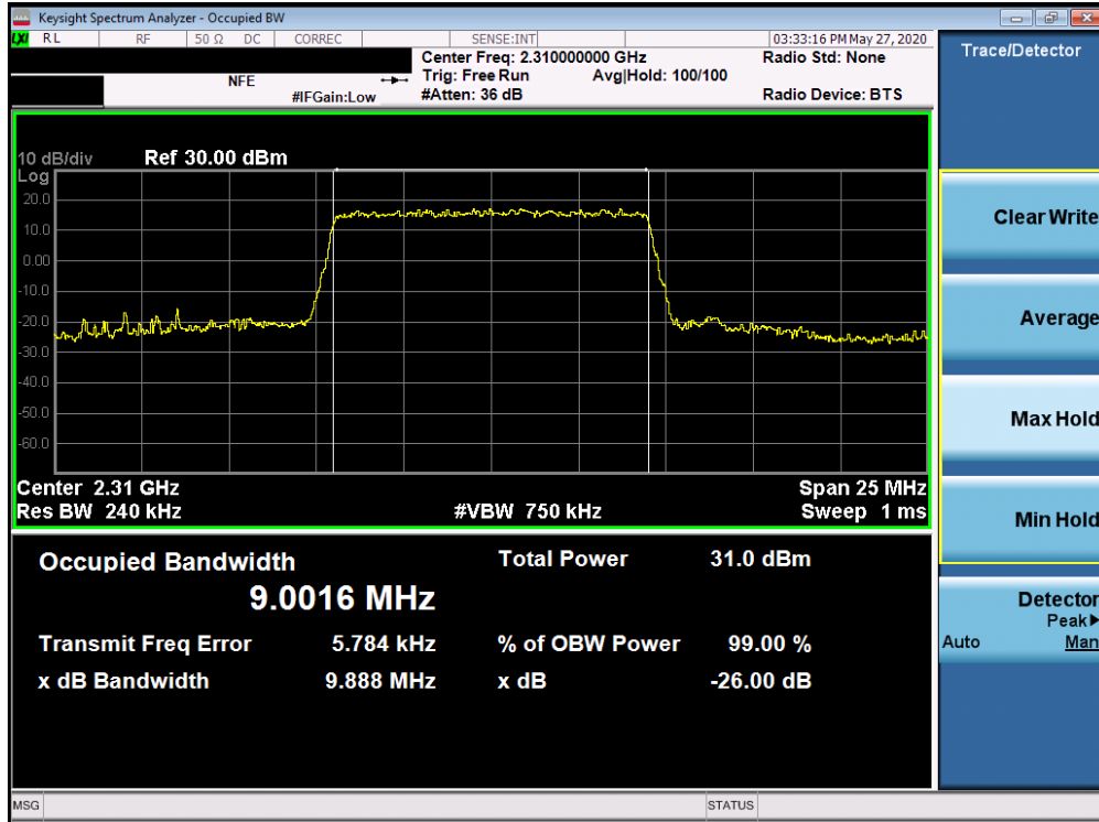
Plot 7-208. Occupied Bandwidth Plot (Band 30 - 10.0MHz QPSK - Full RB Configuration)
