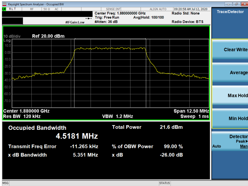
Plot 7-185. Occupied Bandwidth Plot (n25/2 5MHz QPSK-CP-OFDM - Full RB Configuration)
