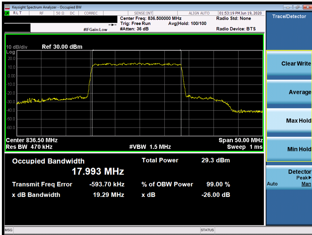
Plot 7-115. Occupied Bandwidth Plot (n5 20MHz 256QAM-CP-OFDM- Full RB Configuration)
