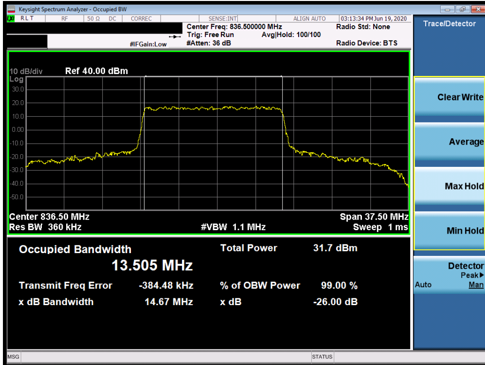
Plot 7-108. Occupied Bandwidth Plot (n5 15MHz 16QAM-CP-OFDM - Full RB Configuration)
