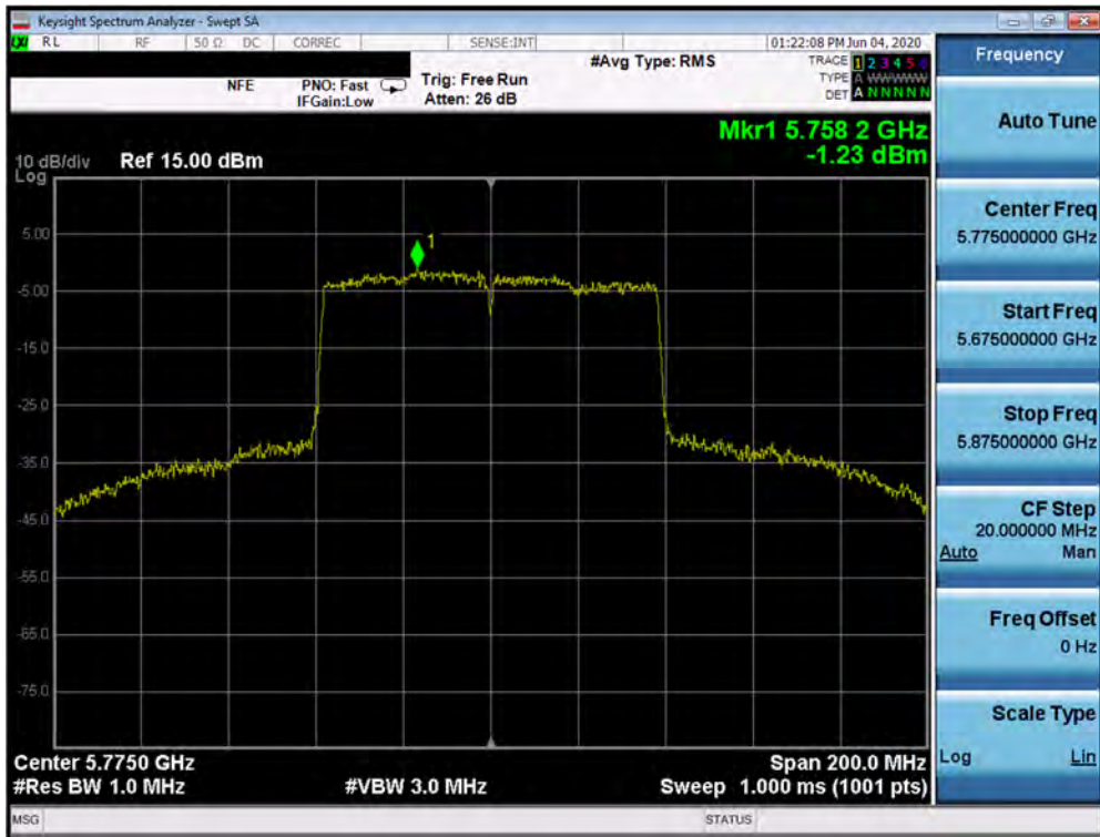
Plot 7-257. Power Spectral Density Plot SISO ANT2 (80MHz BW 802.11ac (UNII Band 3) – Ch. 155)
