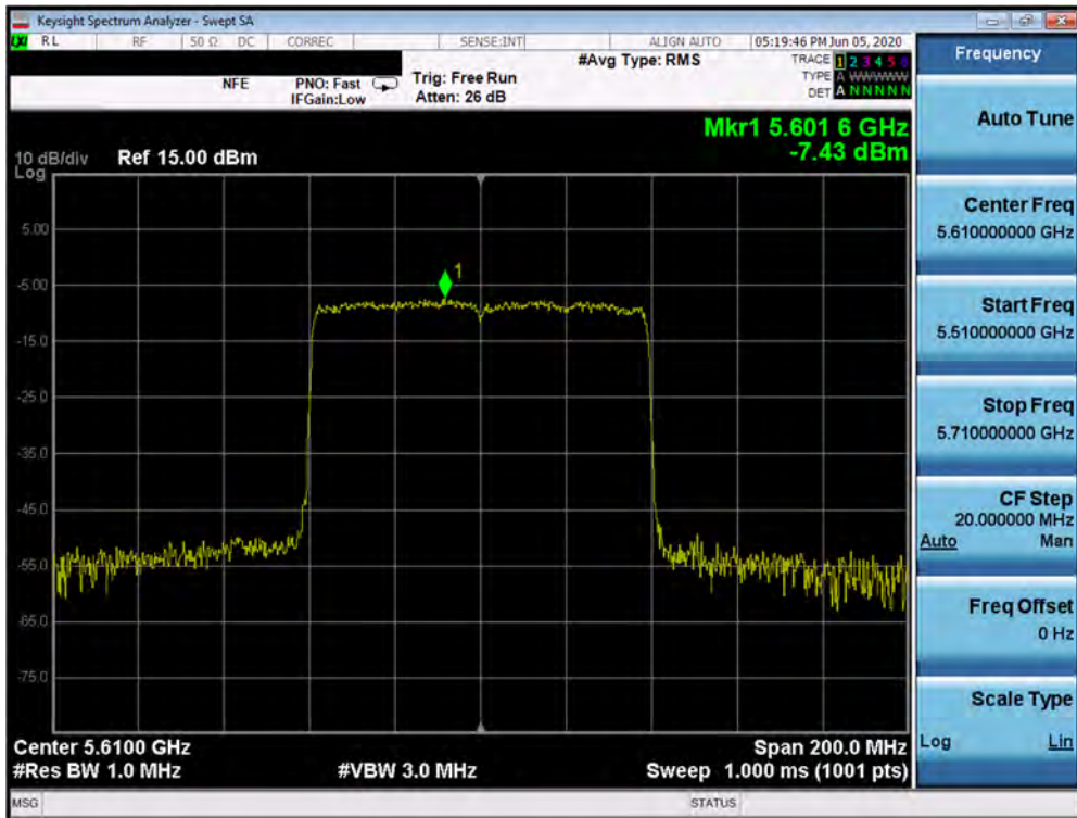
Plot 7-176. Power Spectral Density Plot SISO ANT1 (80MHz BW 802.11ax (UNII Band 2C) – Ch. 122)
