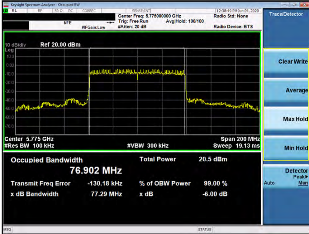
Plot 7-126. 6dB Bandwidth Plot SISO ANT2 (80MHz BW 802.11ax (UNII Band 3) – Ch. 155)
