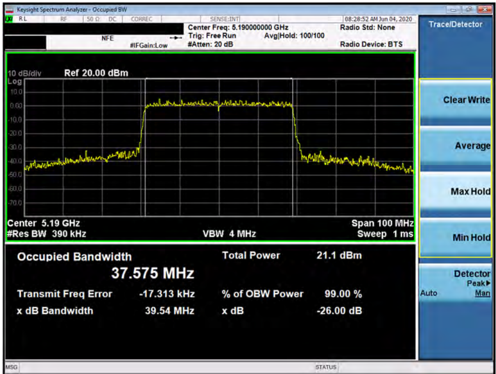
Plot 7-57. 26dB Bandwidth Plot SISO ANT2 (40MHz BW 802.11ax (UNII Band 1) – Ch. 38)
