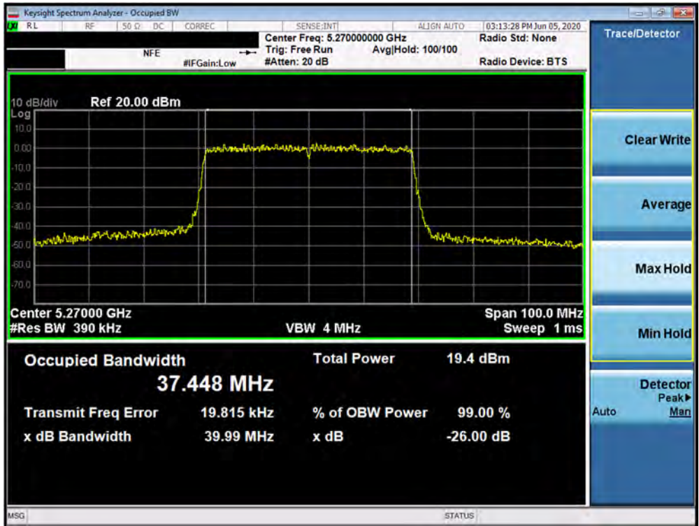
Plot 7-21. 26dB Bandwidth Plot SISO ANT1 (40MHz BW 802.11ax (UNII Band 2A) – Ch. 54)
