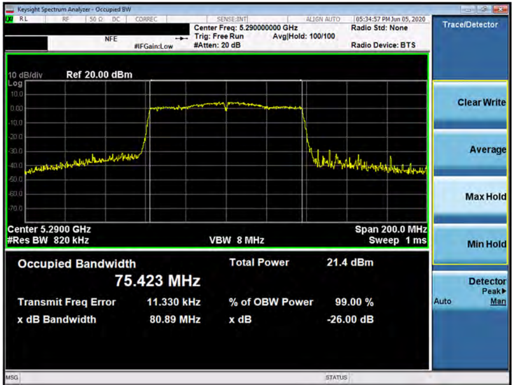
Plot 7-23. 26dB Bandwidth Plot SISO ANT1 (80MHz BW 802.11ac (UNII Band 2A) – Ch. 58)
