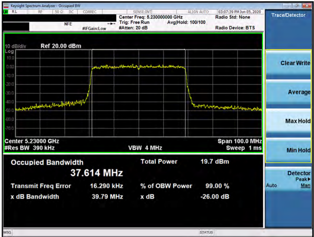
Plot 7-10. 26dB Bandwidth Plot SISO ANT1 (40MHz BW 802.11ax (UNII Band 1) – Ch. 46)
