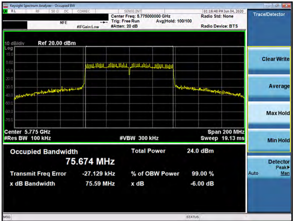
Plot 7-125. 6dB Bandwidth Plot SISO ANT2 (80MHz BW 802.11ac (UNII Band 3) – Ch. 155)
