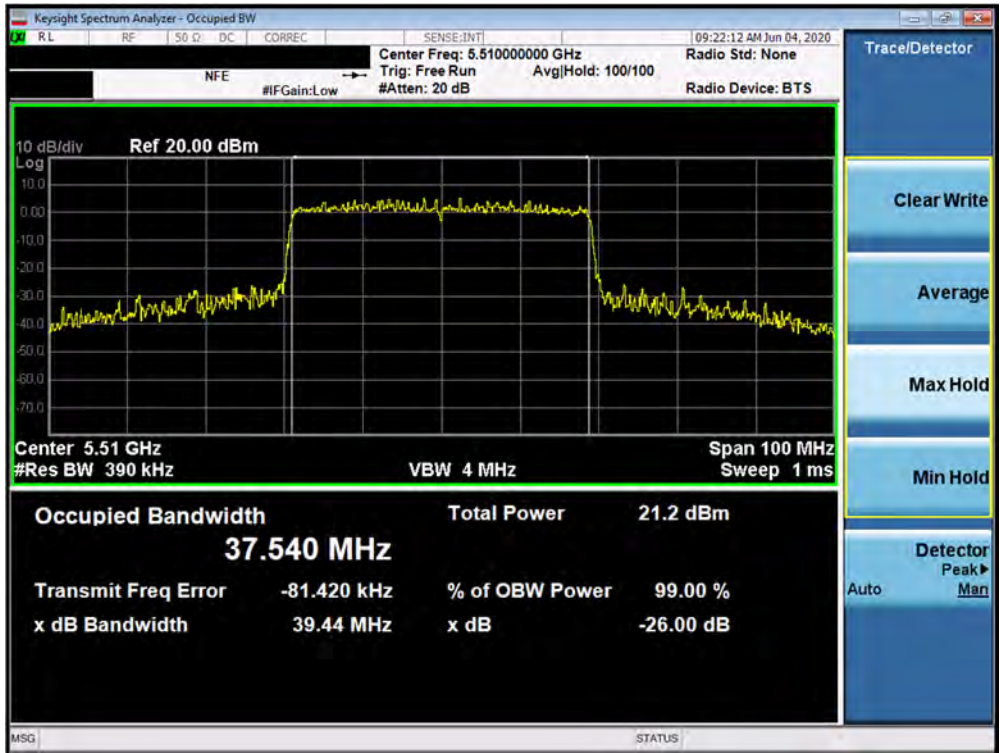
Plot 7-88. 26dB Bandwidth Plot SISO ANT2 (40MHz BW 802.11ax (UNII Band 2C) – Ch. 102)
