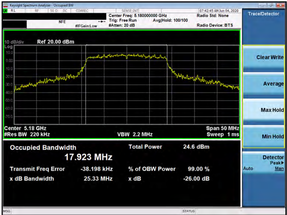
Plot 7-49. 26dB Bandwidth Plot SISO ANT2 (20MHz BW 802.11n (UNII Band 1) – Ch. 36)
