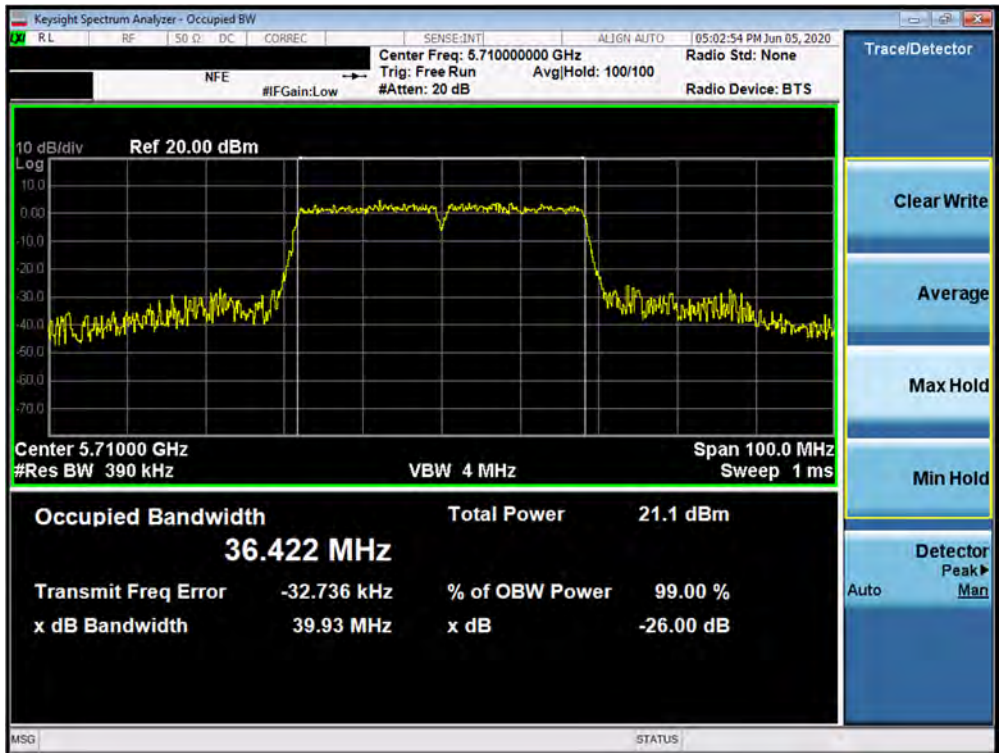
Plot 7-36. 26dB Bandwidth Plot SISO ANT1 (40MHz BW 802.11n (UNII Band 2C) – Ch. 142)
