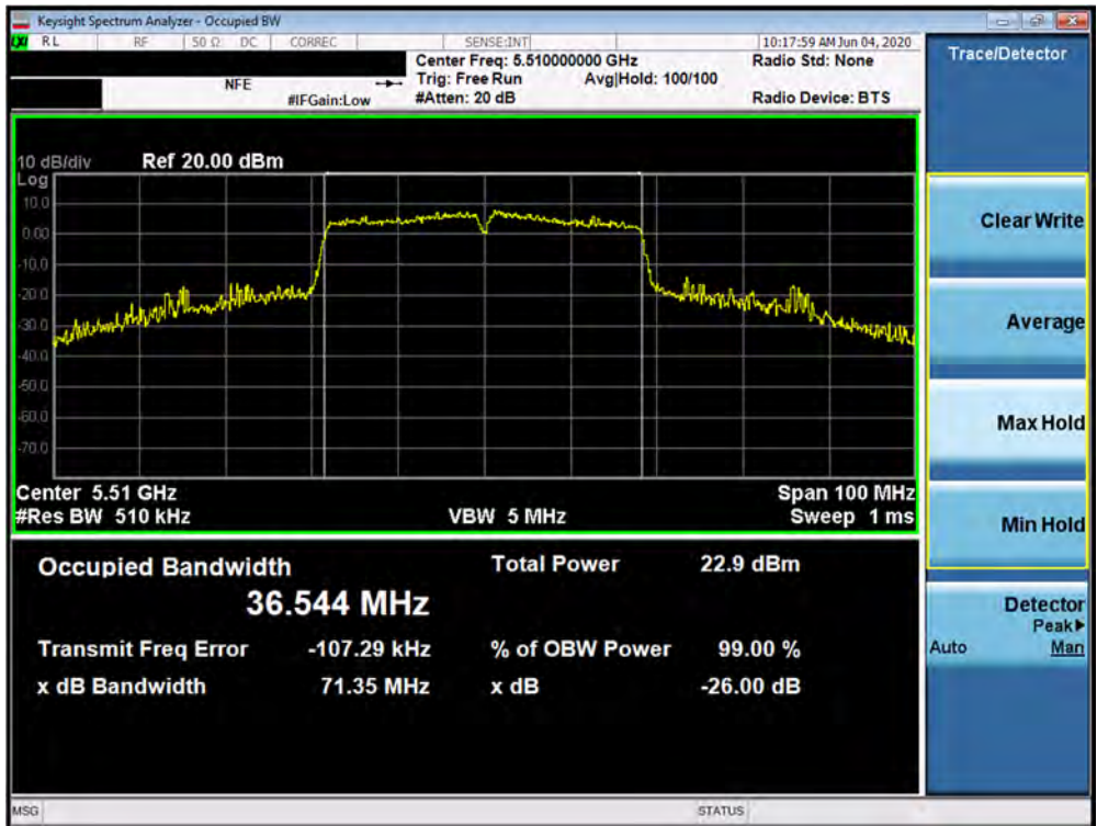
Plot 7-85. 26dB Bandwidth Plot SISO ANT2 (40MHz BW 802.11n (UNII Band 2C) – Ch. 102)
