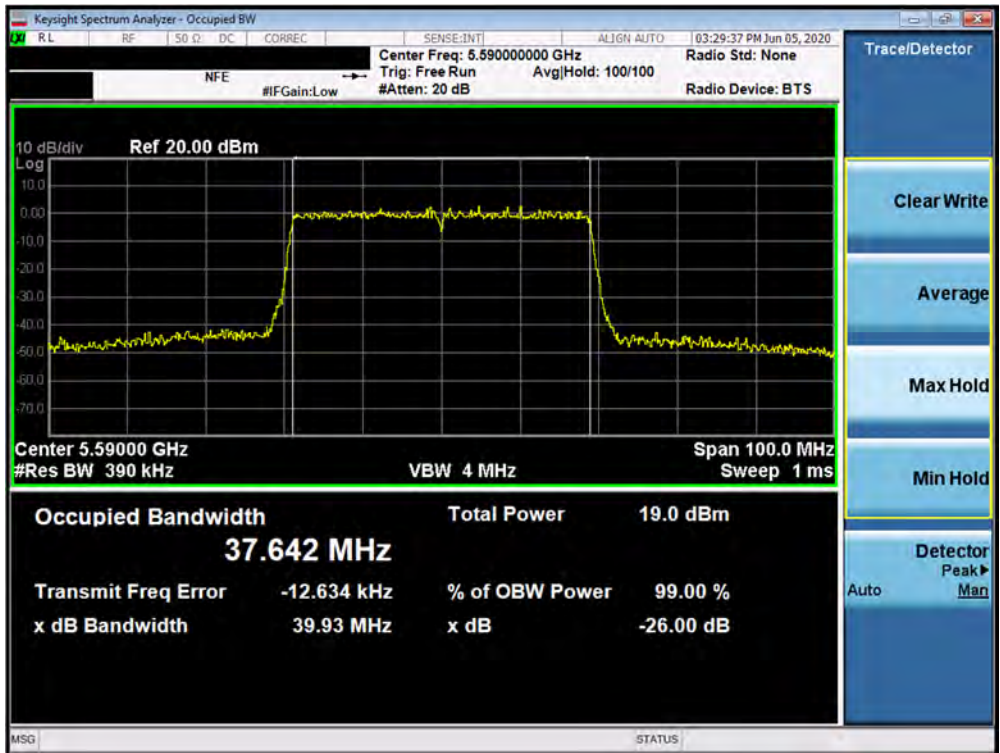
Plot 7-38. 26dB Bandwidth Plot SISO ANT1 (40MHz BW 802.11ax (UNII Band 2C) – Ch. 118)
