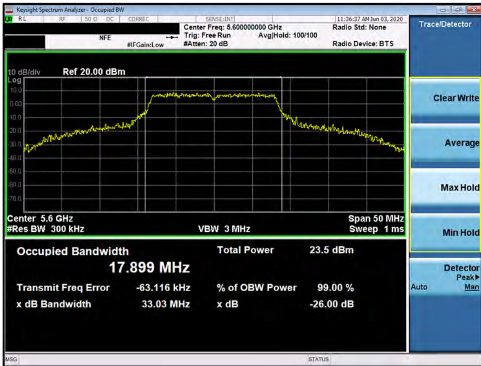
Plot 7-77. 26dB Bandwidth Plot SISO ANT2 (802.11a (UNII Band 2C) – Ch. 120)
