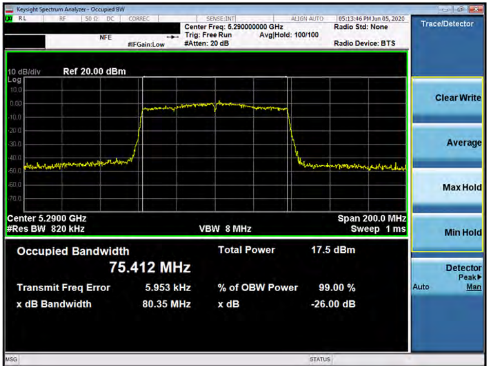
Plot 7-24. 26dB Bandwidth Plot SISO ANT1 (80MHz BW 802.11ax (UNII Band 2A) – Ch. 58)
