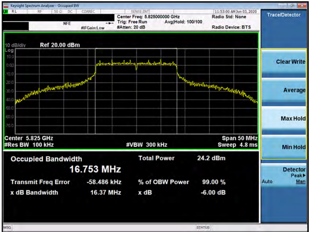
Plot 7-114. 6dB Bandwidth Plot SISO ANT2 (802.11a (UNII Band 3) – Ch. 165)
