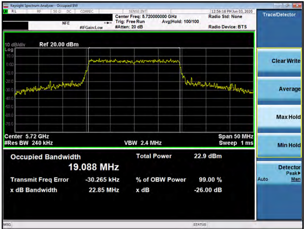
Plot 7-84. 26dB Bandwidth Plot SISO ANT2 (20MHz BW 802.11ax (UNII Band 2C) – Ch. 144)
