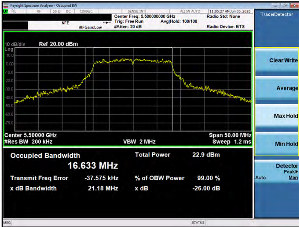
Plot 7-25. 26dB Bandwidth Plot SISO ANT1 (802.11a (UNII Band 2C) – Ch. 100)
