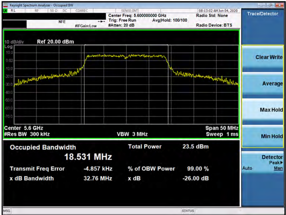
Plot 7-80. 26dB Bandwidth Plot SISO ANT2 (20MHz BW 802.11n (UNII Band 2C) – Ch. 120)
