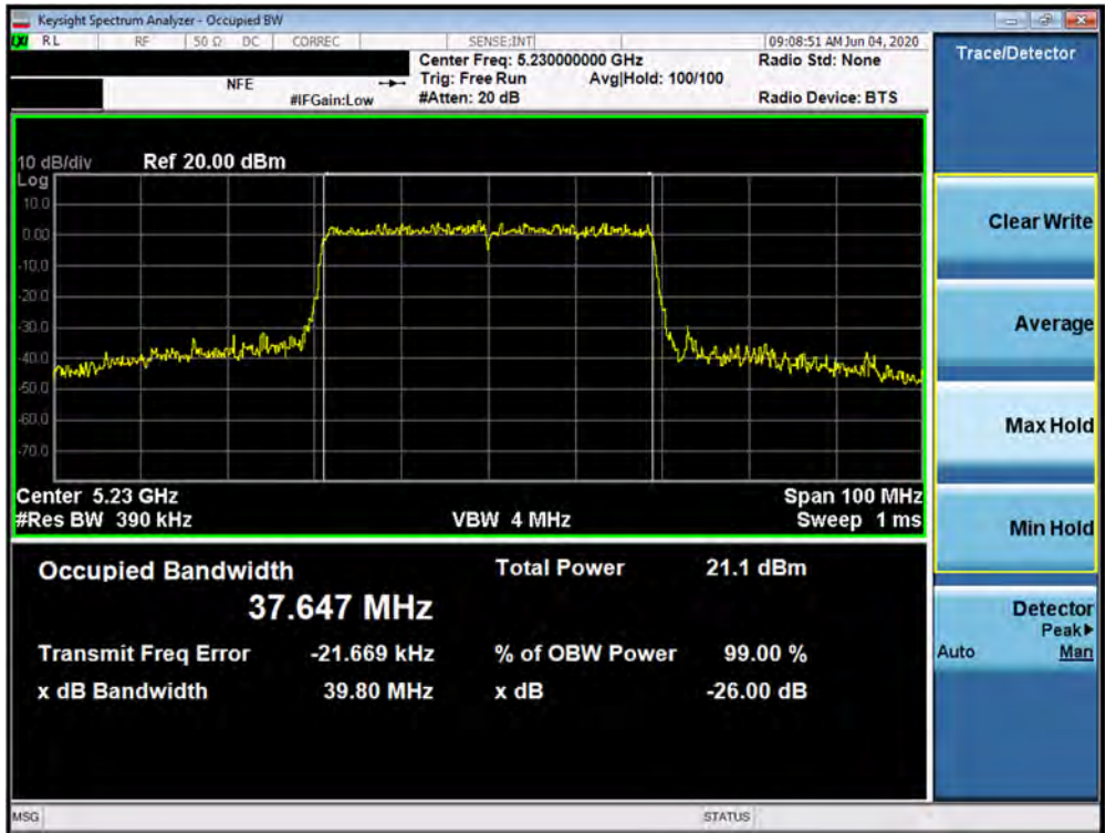
Plot 7-58. 26dB Bandwidth Plot SISO ANT2 (40MHz BW 802.11ax (UNII Band 1) – Ch. 46)
