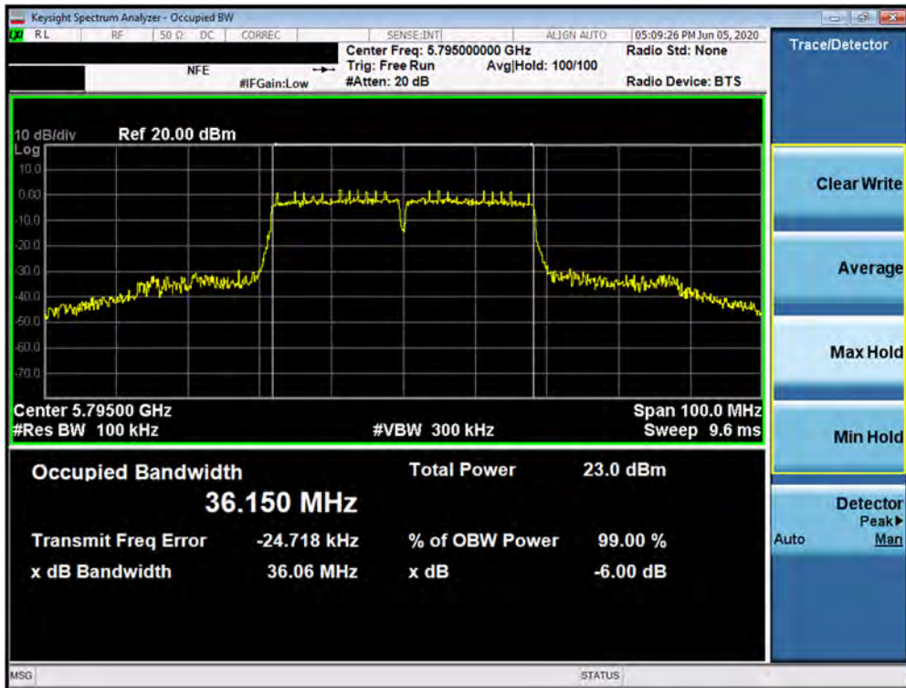
Plot 7-107. 6dB Bandwidth Plot SISO ANT1 (40MHz BW 802.11n (UNII Band 3) – Ch. 159)
