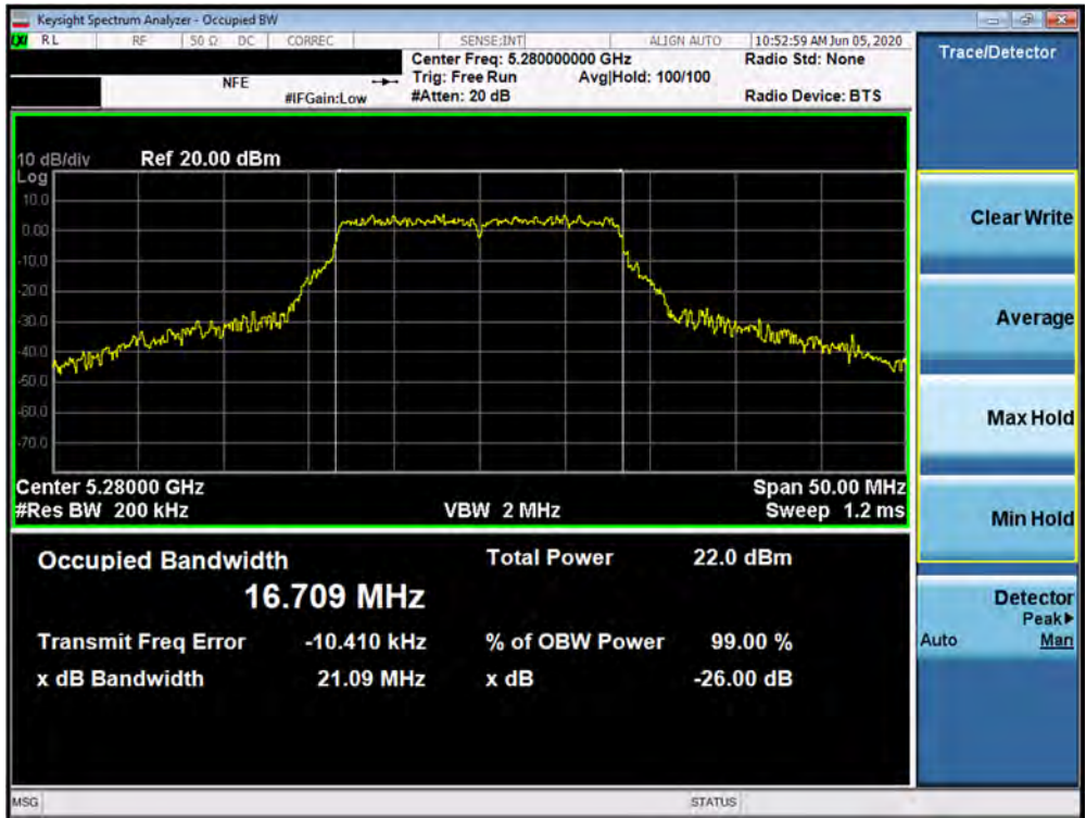
Plot 7-14. 26dB Bandwidth Plot SISO ANT1 (802.11a (UNII Band 2A) – Ch. 56)
