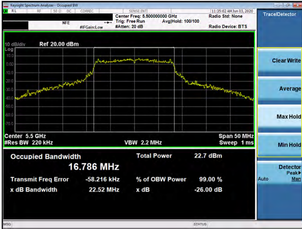
Plot 7-76. 26dB Bandwidth Plot SISO ANT2 (802.11a (UNII Band 2C) – Ch. 100)
