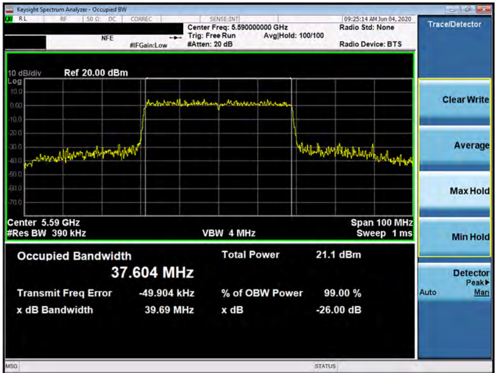
Plot 7-89. 26dB Bandwidth Plot SISO ANT2 (40MHz BW 802.11ax (UNII Band 2C) – Ch. 118)
