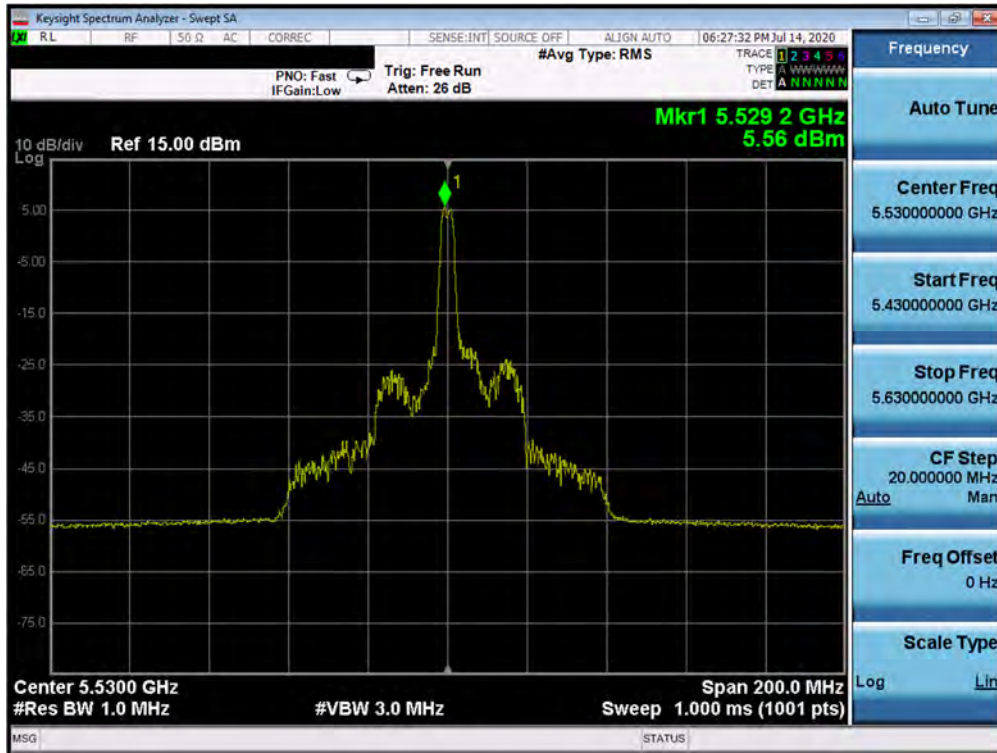
Plot 7-289. Power Spectral Density Plot MIMO ANT2 (80MHz BW 802.11ax – 26 Tones (UNII Band 2C) – Ch. 106)
