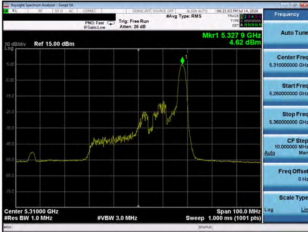
Plot 7-281. Power Spectral Density Plot MIMO ANT2 (40MHz BW 802.11ax – 26 Tones (UNII Band 2A) – Ch. 62)
