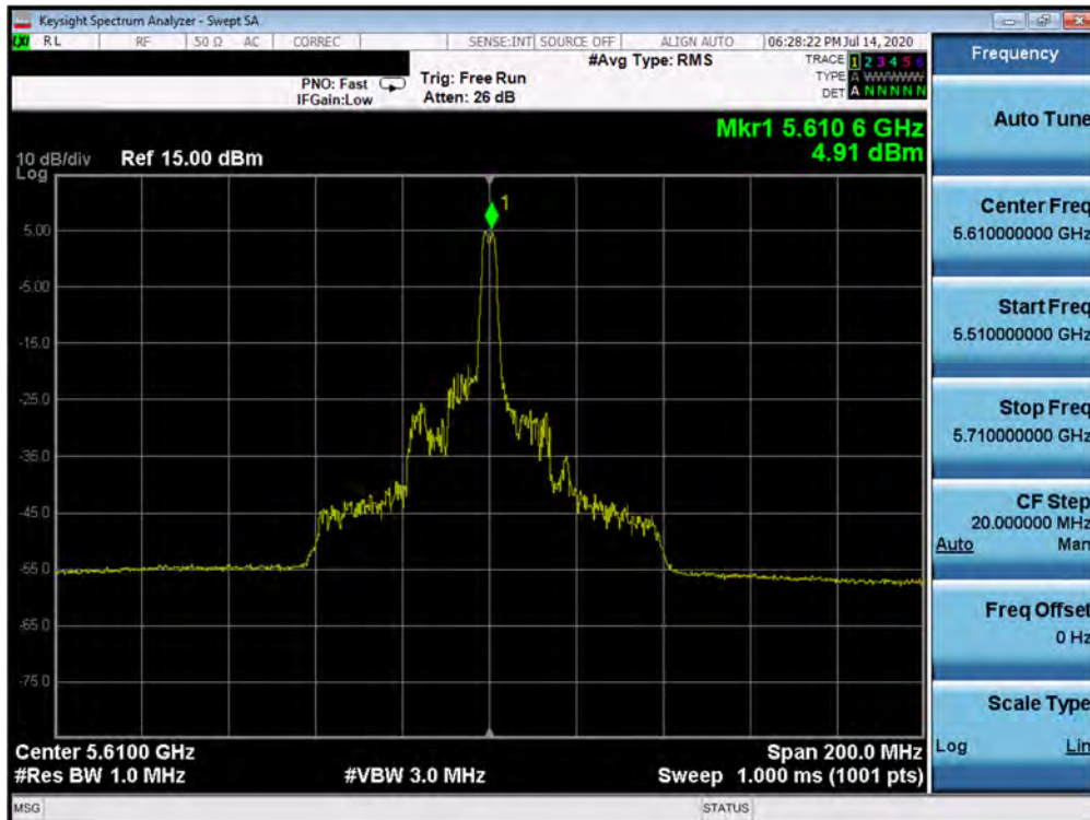
Plot 7-290. Power Spectral Density Plot MIMO ANT2 (80MHz BW 802.11ax – 26 Tones (UNII Band 2C) – Ch. 122)
