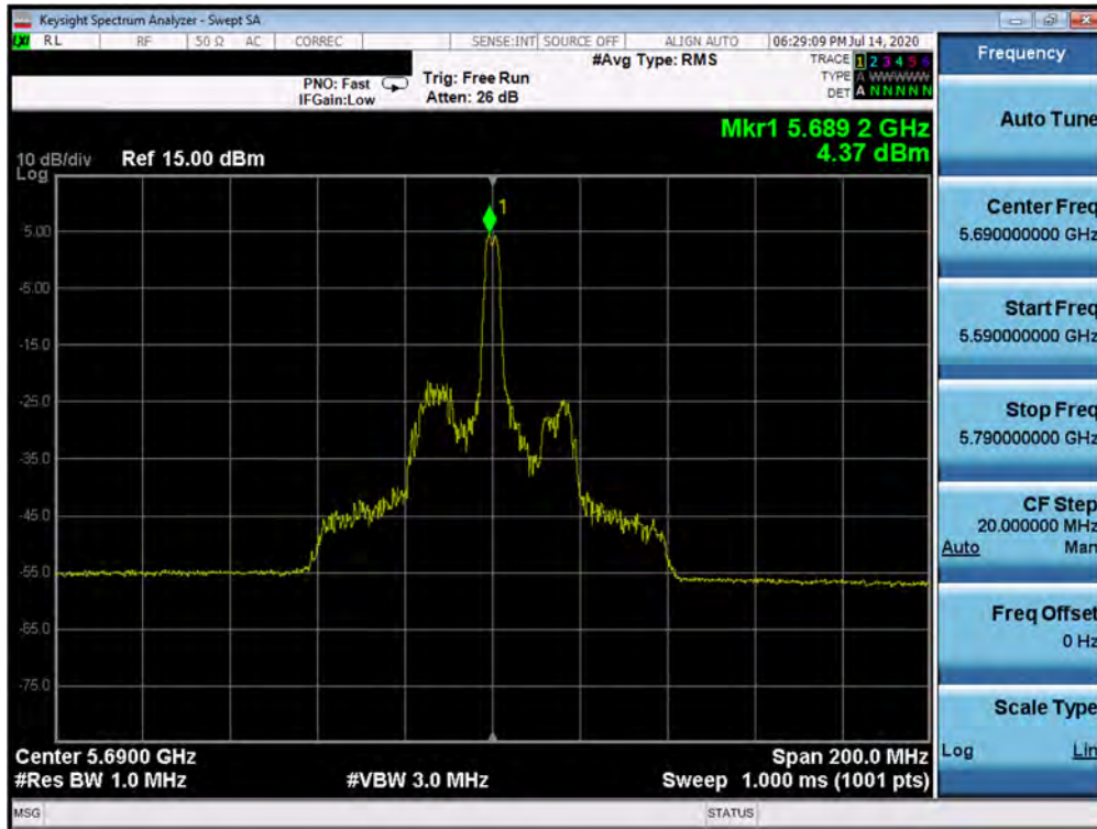
Plot 7-291. Power Spectral Density Plot MIMO ANT2 (80MHz BW 802.11ax – 26 Tones (UNII Band 2C) – Ch. 138)
