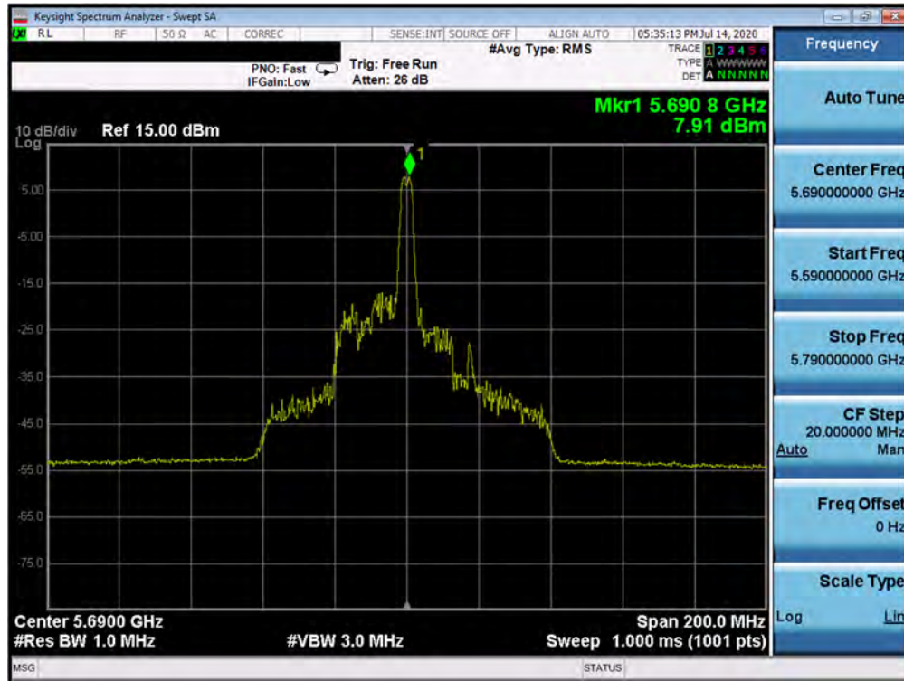
Plot 7-129. Power Spectral Density Plot SISO ANT1 (80MHz BW 802.11ax – 26 Tones (UNII Band 2C) – Ch. 138)
