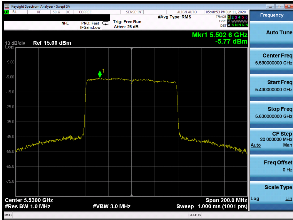
Plot 7-208. Power Spectral Density Plot SISO ANT2 (80MHz BW 802.11ax – Full Tones (UNII Band 2C) – Ch. 106)
