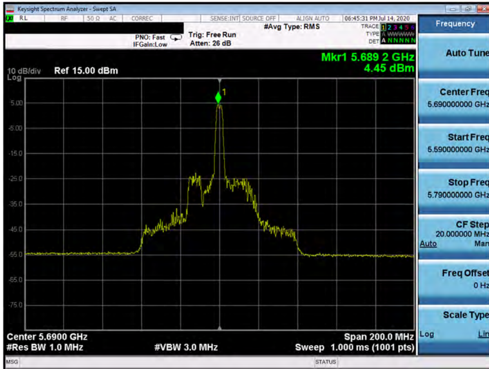
Plot 7-237. Power Spectral Density Plot MIMO ANT1 (80MHz BW 802.11ax – 26 Tones (UNII Band 2C) – Ch. 138)
