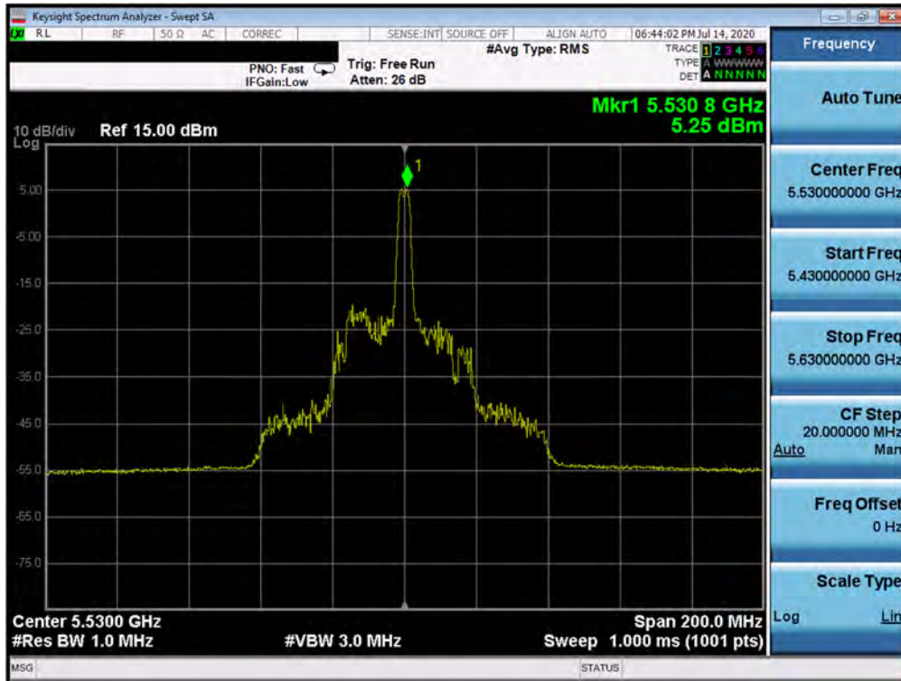
Plot 7-235. Power Spectral Density Plot MIMO ANT1 (80MHz BW 802.11ax – 26 Tones (UNII Band 2C) – Ch. 106)
