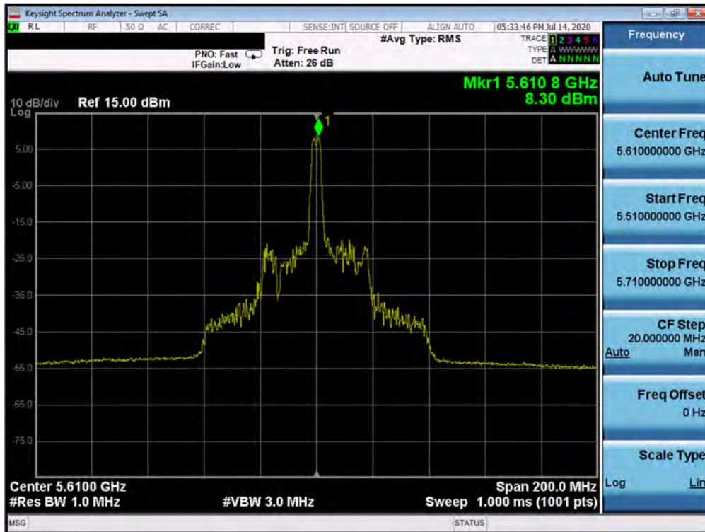
Plot 7-128. Power Spectral Density Plot SISO ANT1 (80MHz BW 802.11ax – 26 Tones (UNII Band 2C) – Ch. 122)
