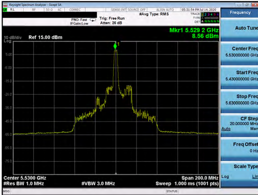
Plot 7-127. Power Spectral Density Plot SISO ANT1 (80MHz BW 802.11ax – 26 Tones (UNII Band 2C) – Ch. 106)
