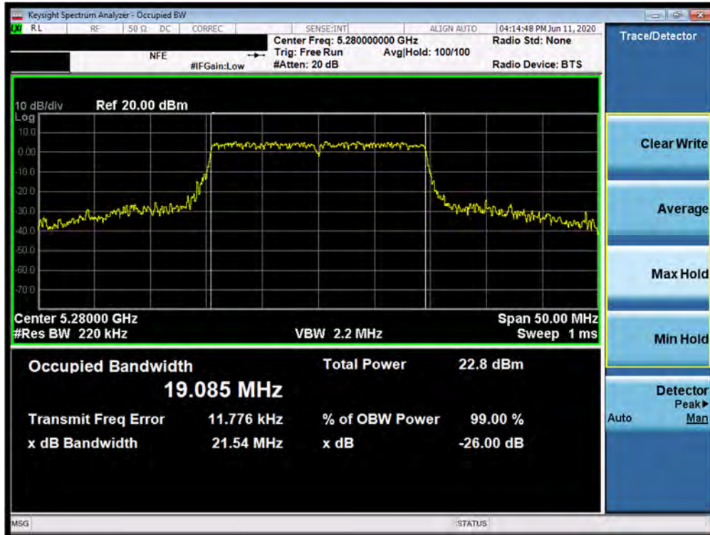
Plot 7-71. 26dB Bandwidth Plot SISO ANT2 (20MHz BW 802.11ax – 242 Tones (UNII Band 2A) – Ch. 56)
