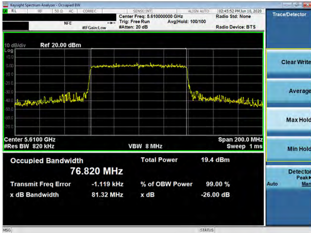
Plot 7-41. 26dB Bandwidth Plot SISO ANT1 (80MHz BW 802.11ax – 996 Tones (UNII Band 2C) – Ch. 122)
