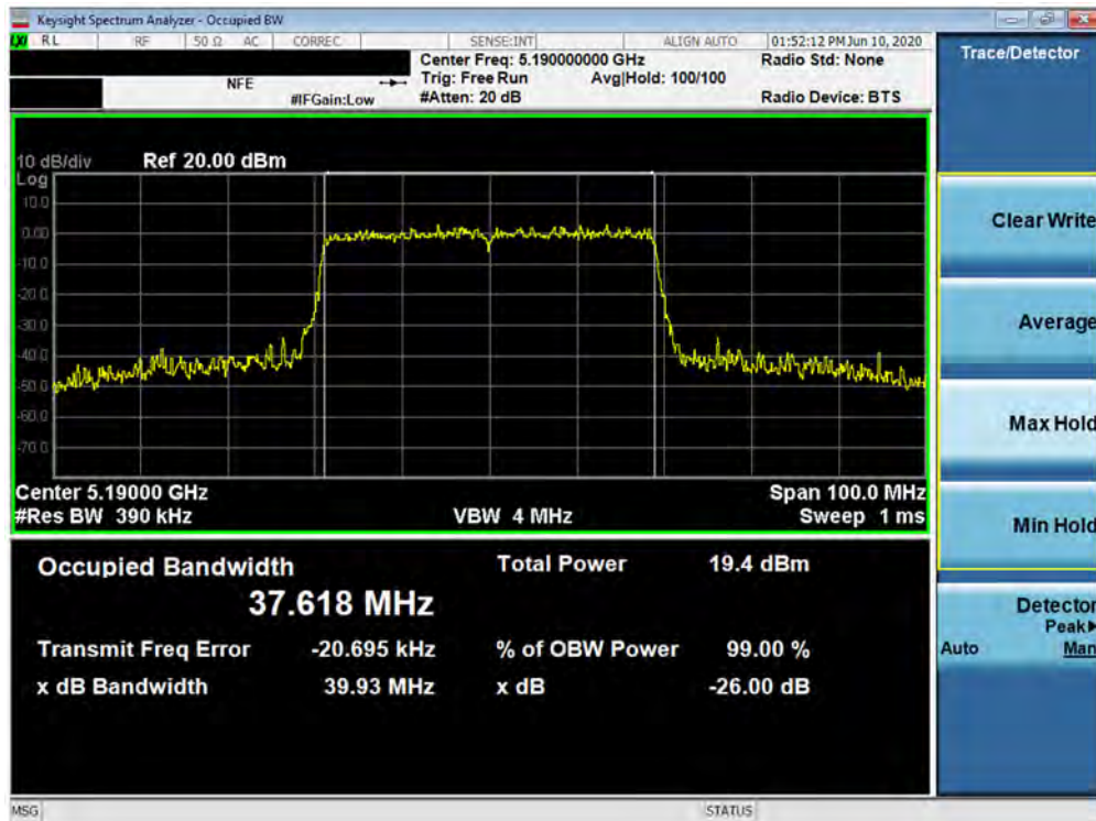
Plot 7-25. 26dB Bandwidth Plot SISO ANT1 (40MHz BW 802.11ax – 484 Tones (UNII Band 1) – Ch. 38)
