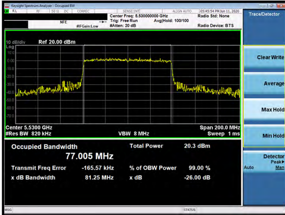
Plot 7-82. 26dB Bandwidth Plot SISO ANT2 (80MHz BW 802.11ax – 996 Tones (UNII Band 2C) – Ch. 106)
