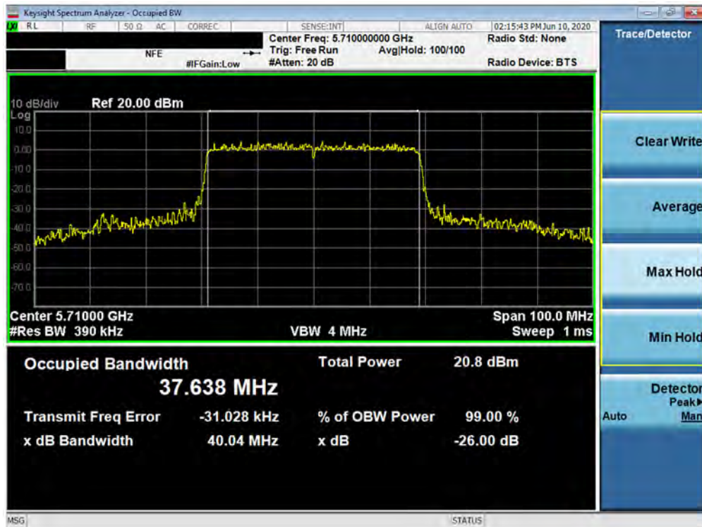
Plot 7-39. 26dB Bandwidth Plot SISO ANT1 (40MHz BW 802.11ax – 484 Tones (UNII Band 2C) – Ch. 142)
