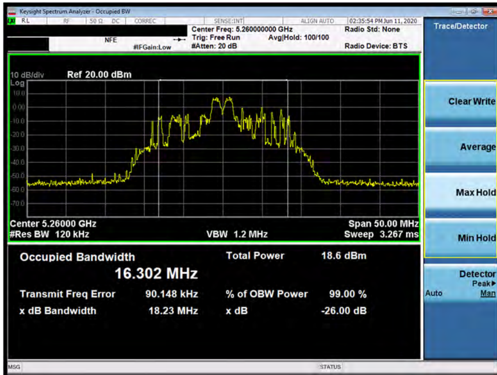
Plot 7-49. 26dB Bandwidth Plot SISO ANT2 (20MHz BW 802.11ax – 26 Tones (UNII Band 2A) – Ch. 52)
