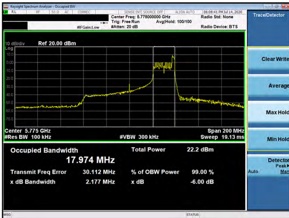
Plot 7-102. 6dB Bandwidth Plot SISO ANT2 (80MHz BW 802.11ax – 26 Tones (UNII Band 3) – Ch. 155)
