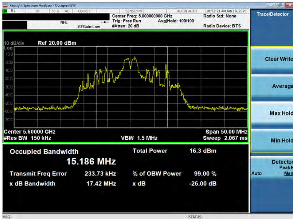
Plot 7-14. 26dB Bandwidth Plot SISO ANT1 (20MHz BW 802.11ax – 26 Tones (UNII Band 2C) – Ch. 120)
