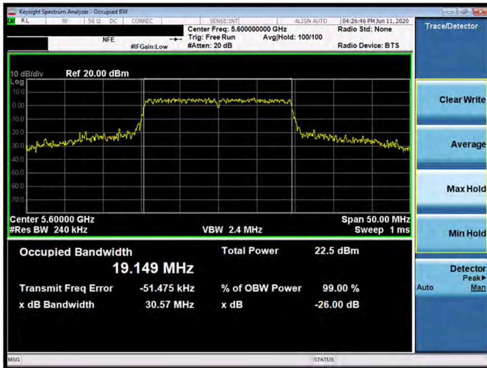
Plot 7-77. 26dB Bandwidth Plot SISO ANT2 (20MHz BW 802.11ax – 242 Tones (UNII Band 2C) – Ch. 120)
