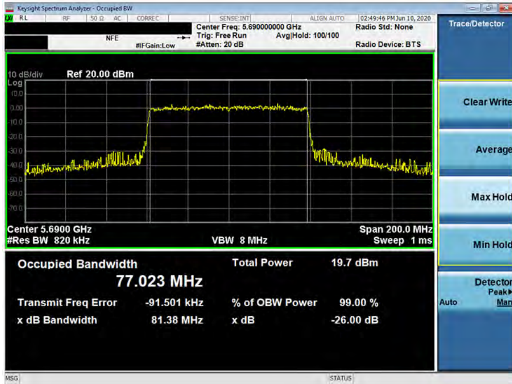
Plot 7-42. 26dB Bandwidth Plot SISO ANT1 (80MHz BW 802.11ax – 996 Tones (UNII Band 2C) – Ch. 138)
