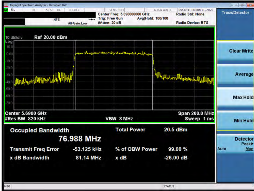
Plot 7-84. 26dB Bandwidth Plot SISO ANT2 (80MHz BW 802.11ax – 996 Tones (UNII Band 2C) – Ch. 138)
