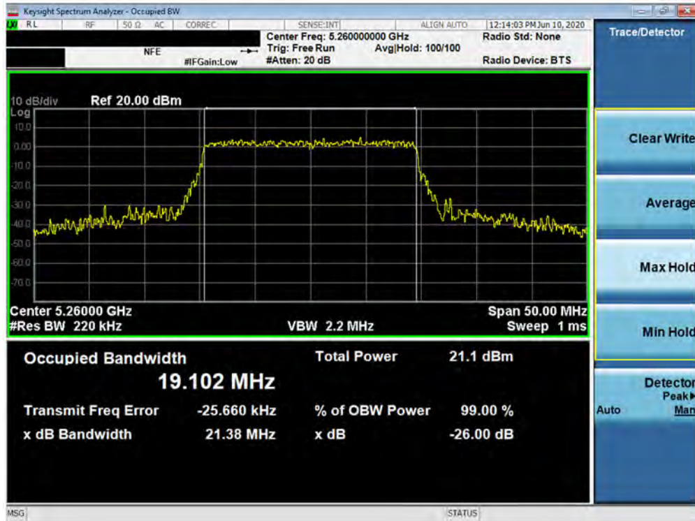
Plot 7-28. 26dB Bandwidth Plot SISO ANT1 (20MHz BW 802.11ax – 242 Tones (UNII Band 2A) – Ch. 52)
