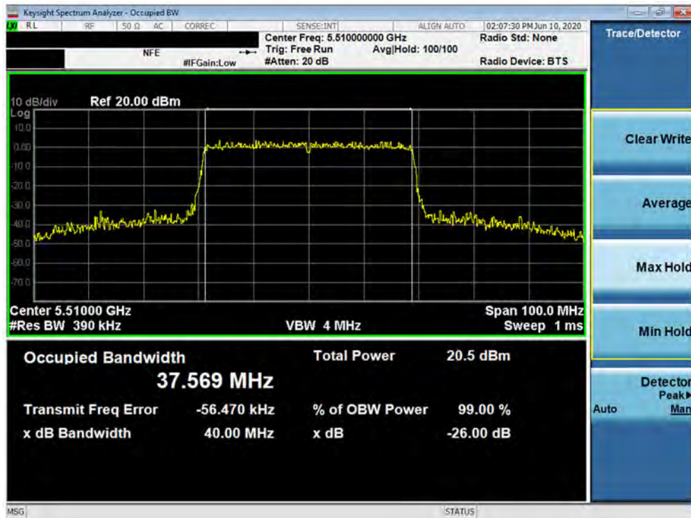
Plot 7-37. 26dB Bandwidth Plot SISO ANT1 (40MHz BW 802.11ax – 484 Tones (UNII Band 2C) – Ch. 102)
