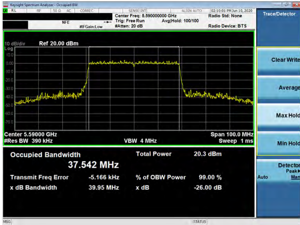
Plot 7-38. 26dB Bandwidth Plot SISO ANT1 (40MHz BW 802.11ax – 484 Tones (UNII Band 2C) – Ch. 118)
