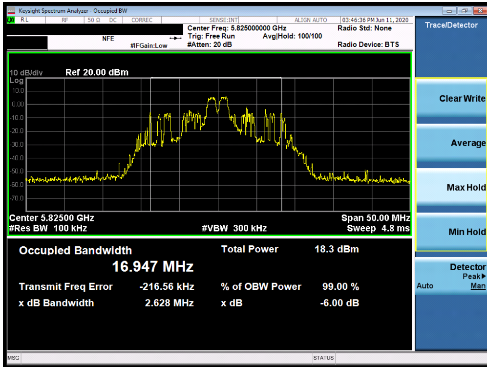
Plot 7-99. 6dB Bandwidth Plot SISO ANT2 (20MHz BW 802.11ax – 26 Tones (UNII Band 3) – Ch. 165)
