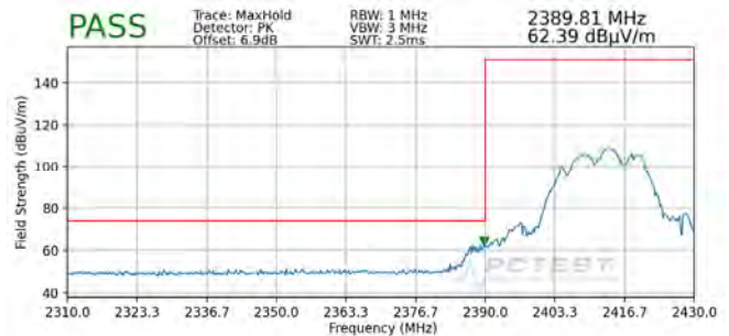
Plot 7-97. Radiated Restricted Lower Band Edge Measurement CDD (Peak)
