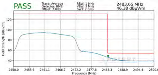
Plot 7-90. Radiated Restricted Upper Band Edge Measurement SISO ANT1 (Average)
