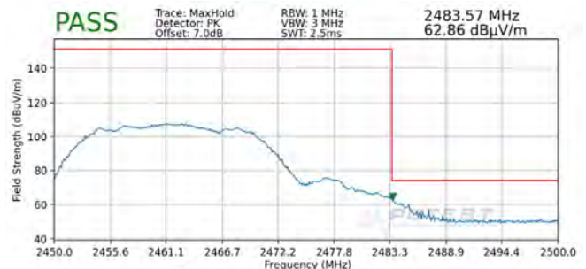
Plot 7-99. Radiated Restricted Upper Band Edge Measurement MIMO (Peak)
