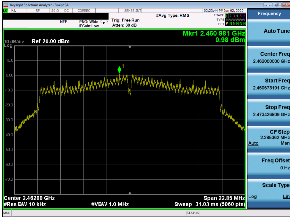
Plot 7-33. Power Spectral Density Plot SISO ANT1 (802.11n (2.4GHz) – Ch. 11)
