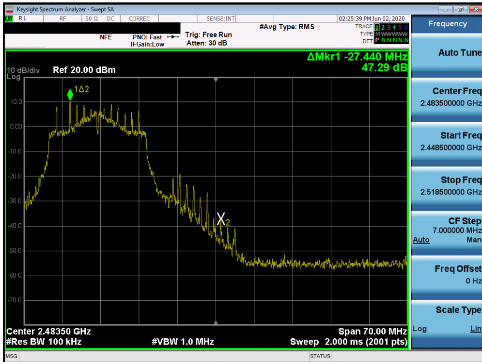
Plot 7-54. Band Edge Plot SISO ANT1 (802.11n (2.4GHz) – Ch. 11)
