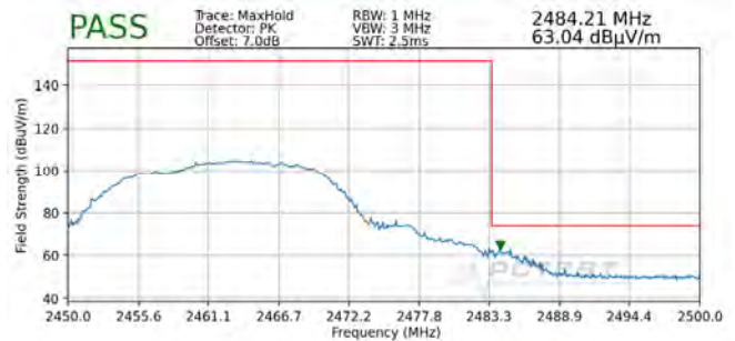
Plot 7-95. Radiated Restricted Upper Band Edge Measurement SISO ANT2 (Peak)
