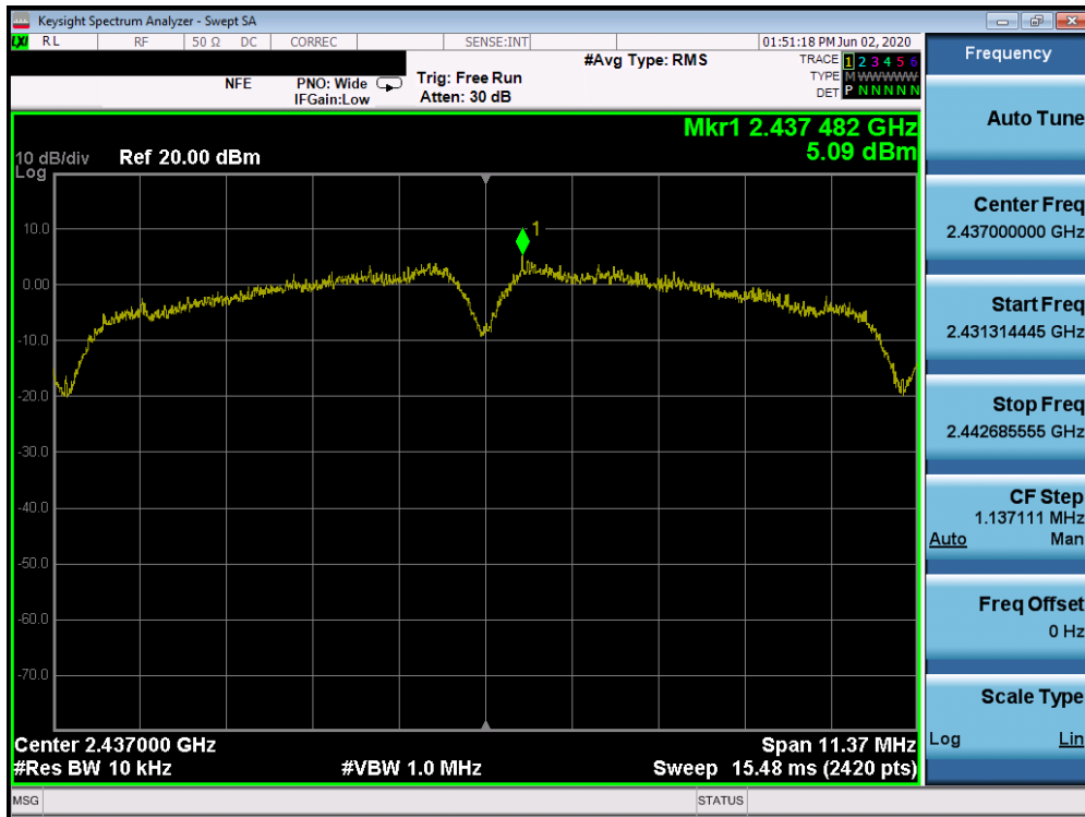
Plot 7-26. Power Spectral Density Plot SISO ANT1 (802.11b – Ch. 6)
