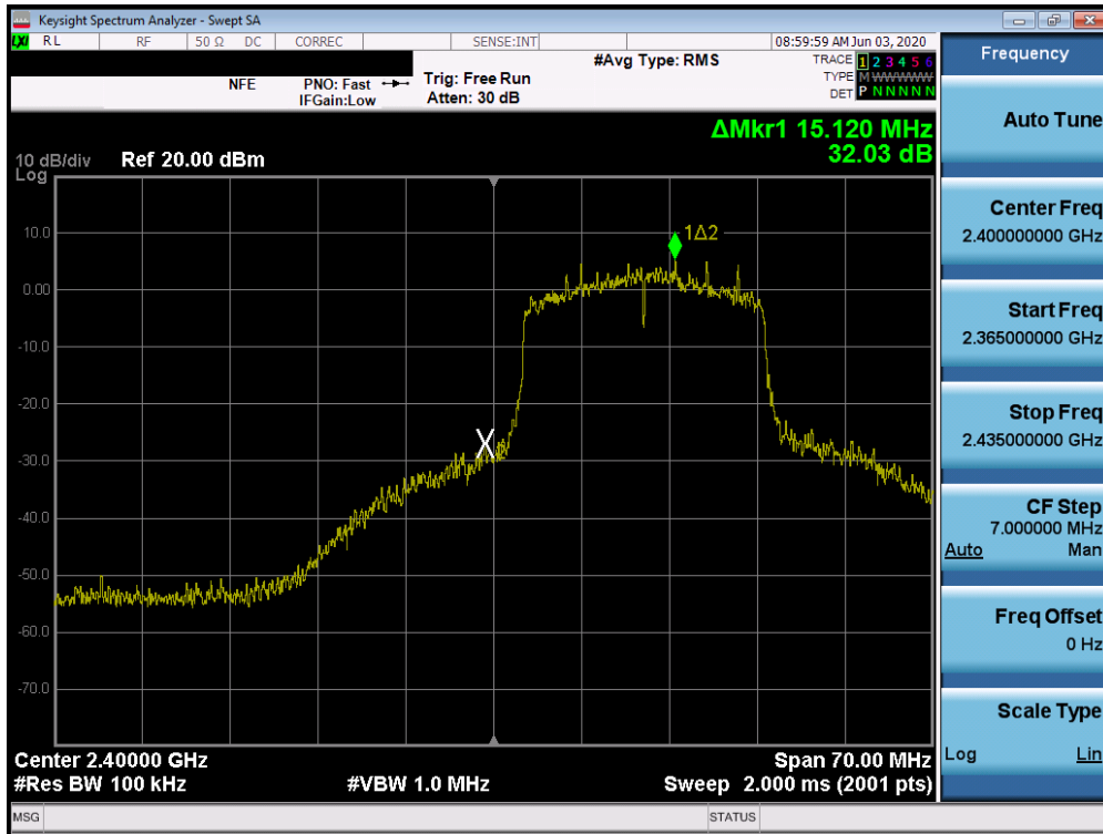
Plot 7-63. Band Edge Plot SISO ANT1 (802.11ax (2.4GHz) – Ch. 1)
