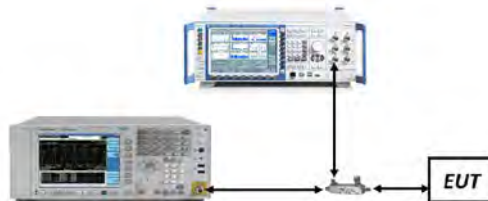
Figure 7-2. Test Instrument & Measurement Setup
