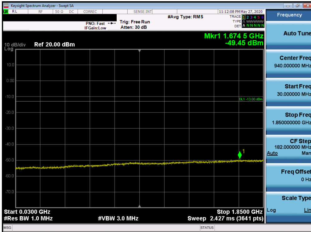
Plot 7-43. Conducted Spurious Plot (PCS CDMA Mode - High Channel)
