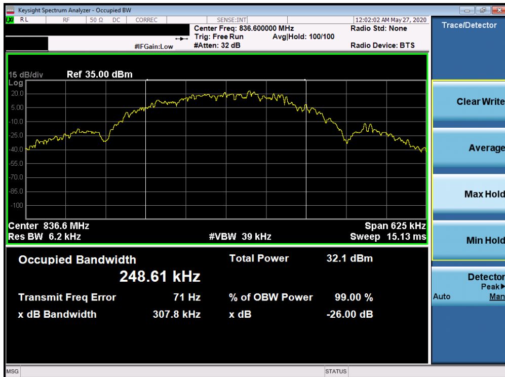
Plot 7-2. Occupied Bandwidth Plot (EDGE850 Mode)
