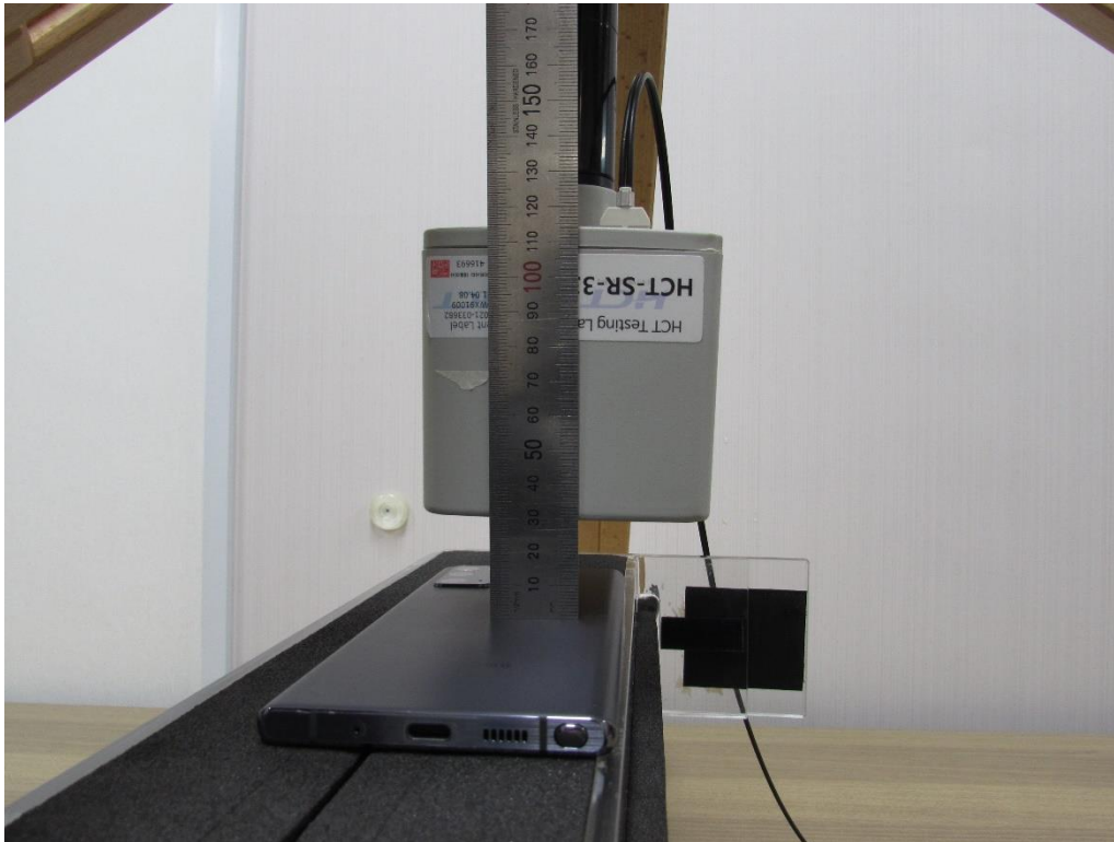
Distance from the rear side of the Device to the center of the Probe from 9.4 cm
