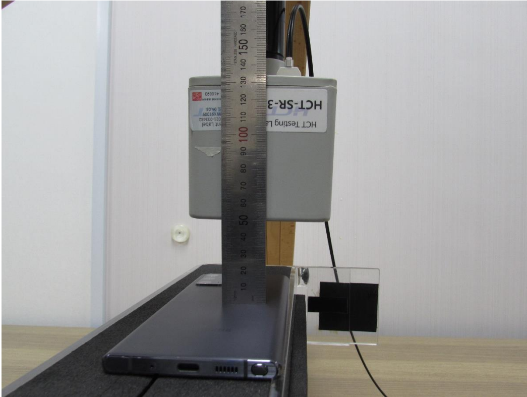
Distance from the rear side of the Device to the center of the Probe from 10.4 cm
