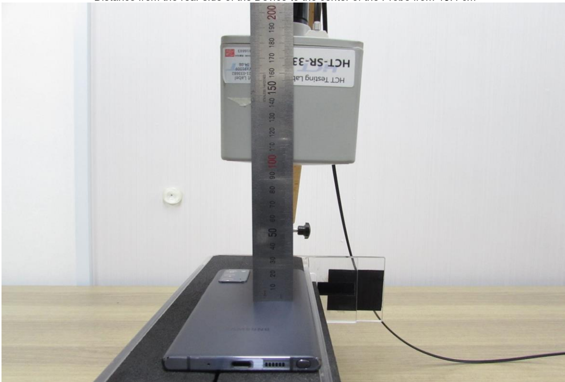
Distance from the rear side of the Device to the center of the Probe from 15.4 cm
