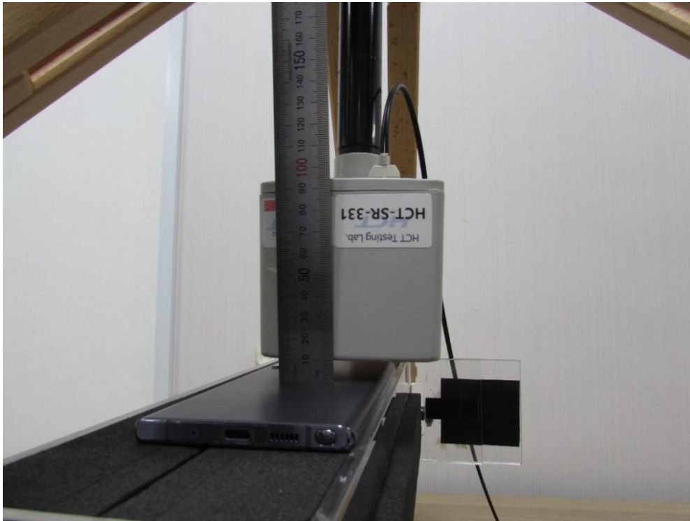
Distance from the rear side of the Device to the center of the Probe from 7.4 cm
