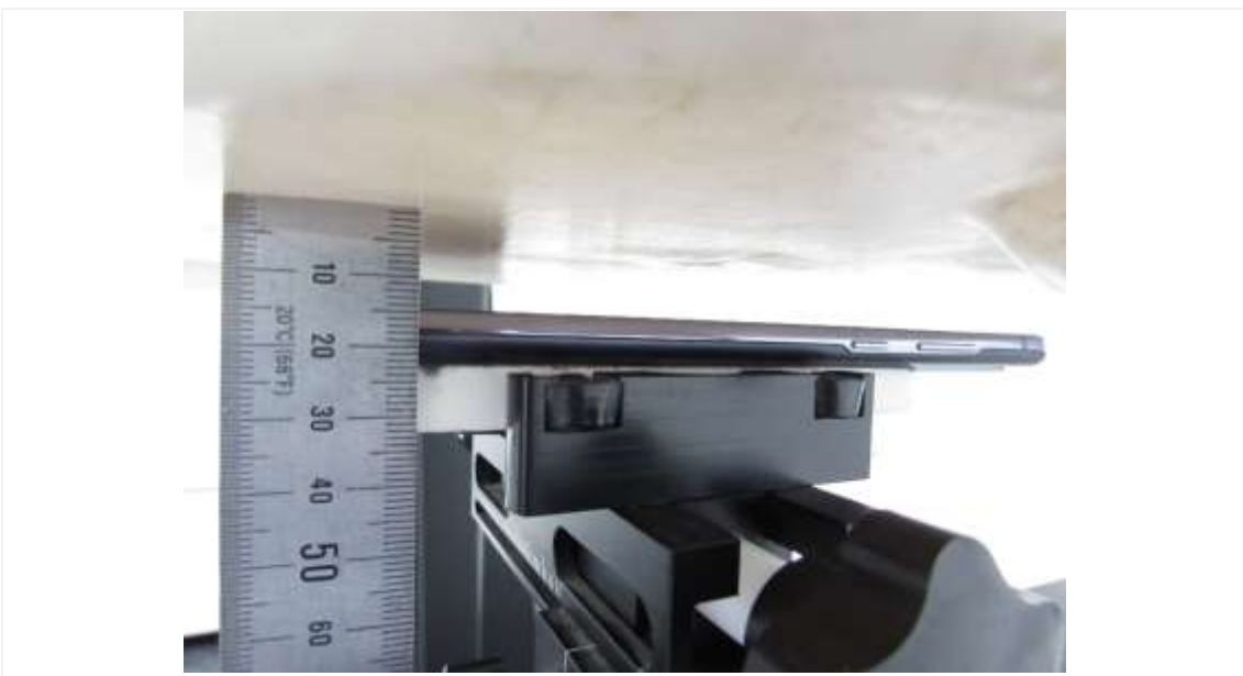
Distance of 15 mm from the EUT
