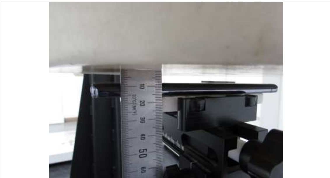
Distance of 8 mm from the EUT
