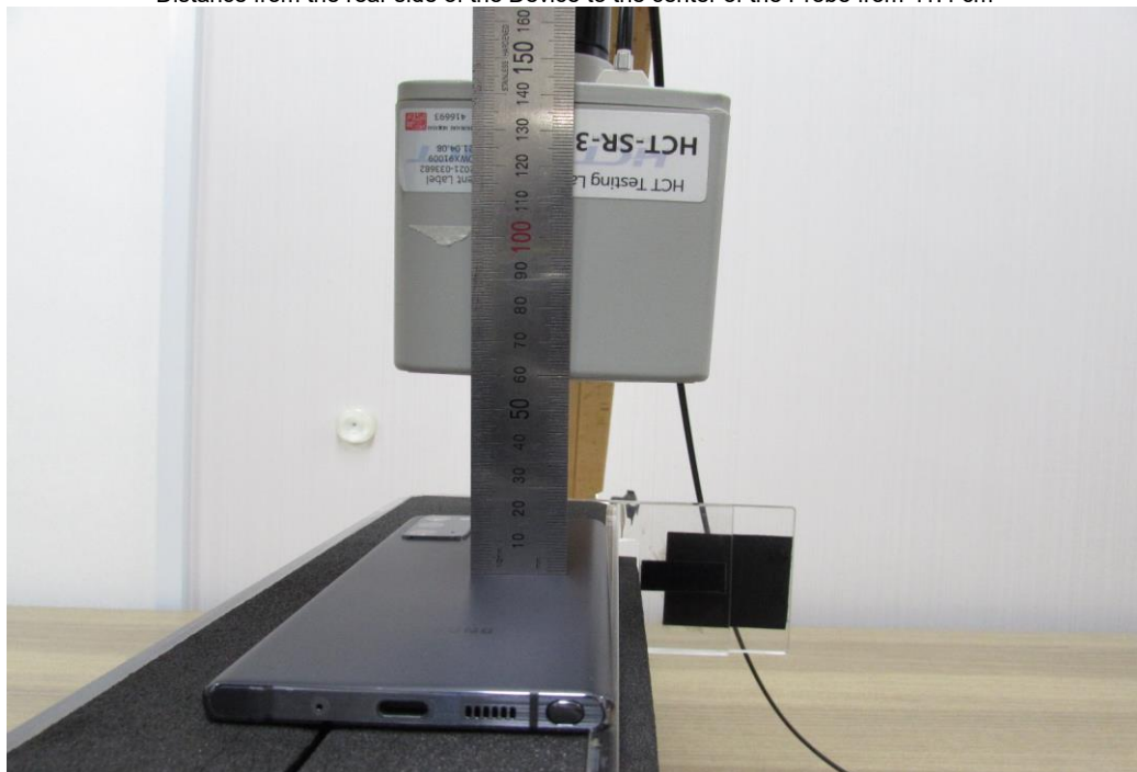
Distance from the rear side of the Device to the center of the Probe from 11.4 cm
