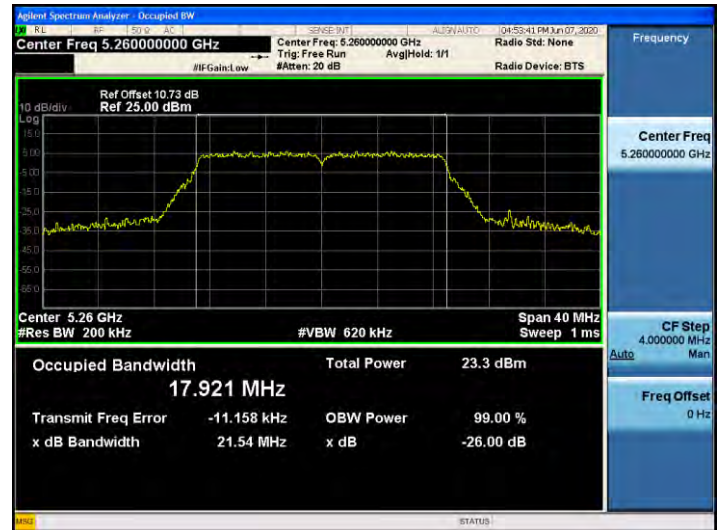
802.11ac_VHT20 UNII 3 BAND 26dB Bandwidth(CH 157)
