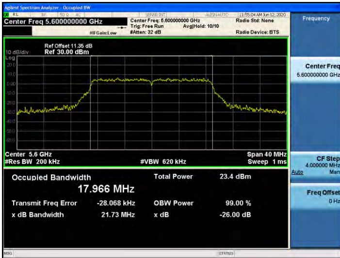
802.11ac_VHT20 UNII 2C BAND 26dB Bandwidth(CH 120)
