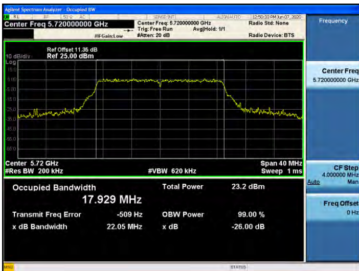
802.11n_HT20 UNII 2C BAND 26dB Bandwidth(CH 144)
