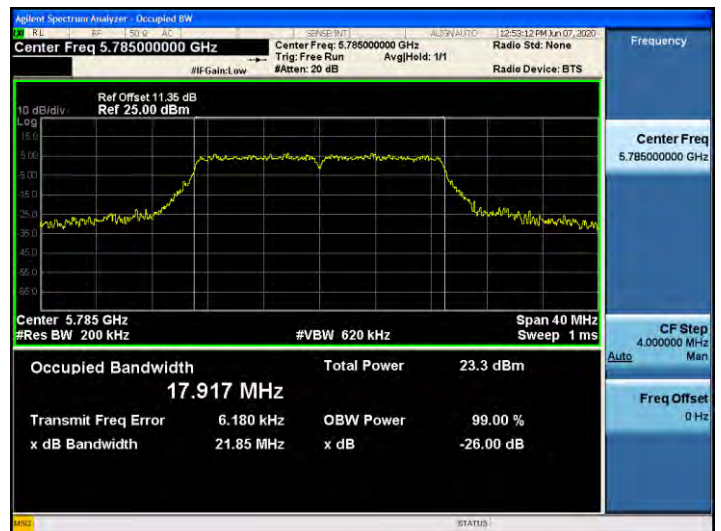
802.11n_HT20 UNII 3 BAND 26dB Bandwidth(CH 157)
