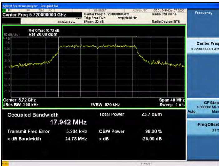
802.11ac_VHT20 UNII 2C BAND 26dB Bandwidth(CH 144)
