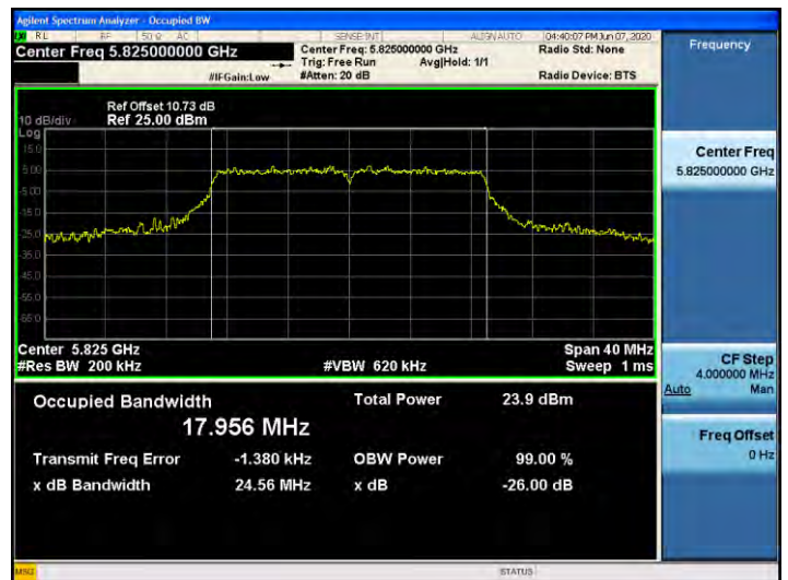
802.11n_HT20 UNII 3 BAND 26dB Bandwidth(CH 165)
