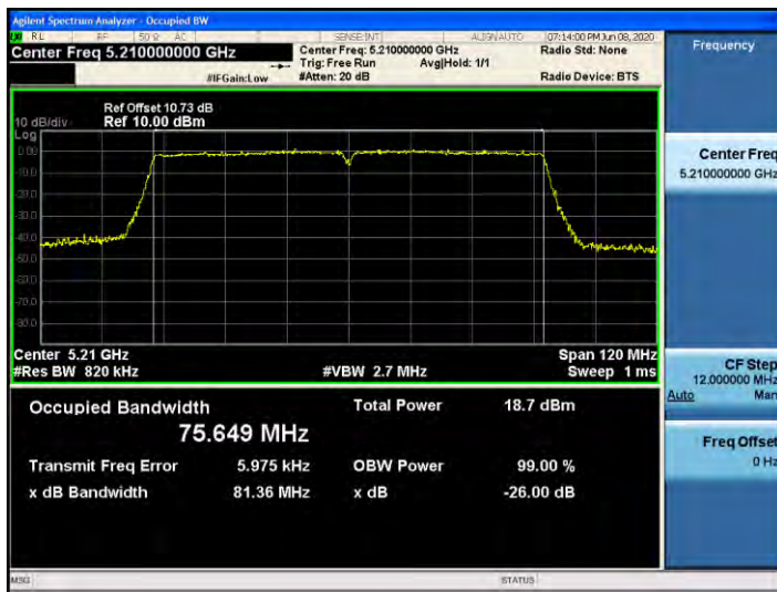
802.11ac_VHT80 UNII 2C BAND 26dB Bandwidth(CH 138)
