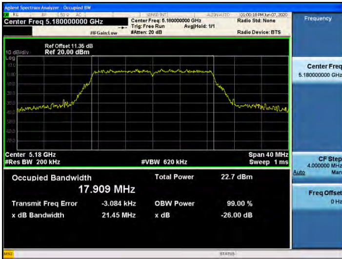
802.11ac_VHT20 UNII 2C BAND 26dB Bandwidth(CH 120)
