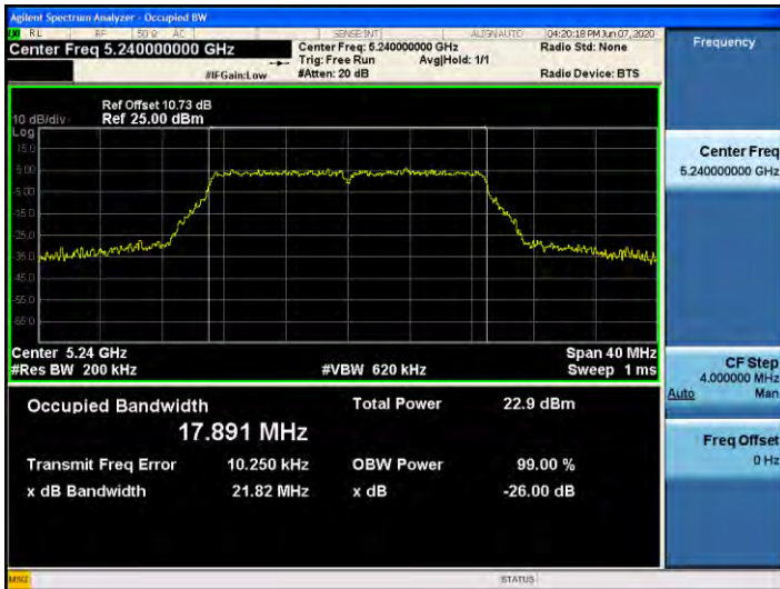
802.11n_HT20 UNII 2C BAND 26dB Bandwidth(CH 144)
