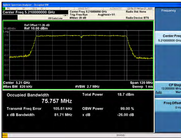
802.11ac_VHT80 UNII 2C BAND 26dB Bandwidth(CH 122)
