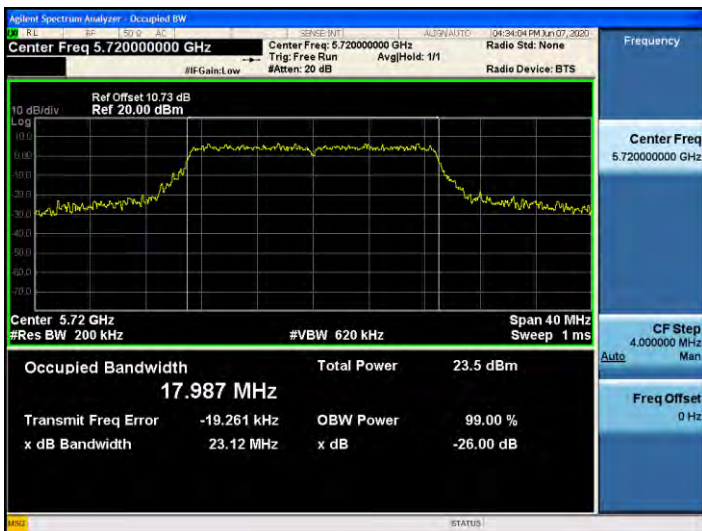
802.11n_HT20 UNII 2C BAND 26dB Bandwidth(CH 144)
