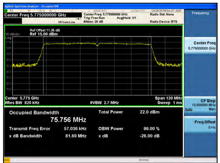
802.11ac_VHT80 UNII 3 BAND 26dB Bandwidth (CH 155)
