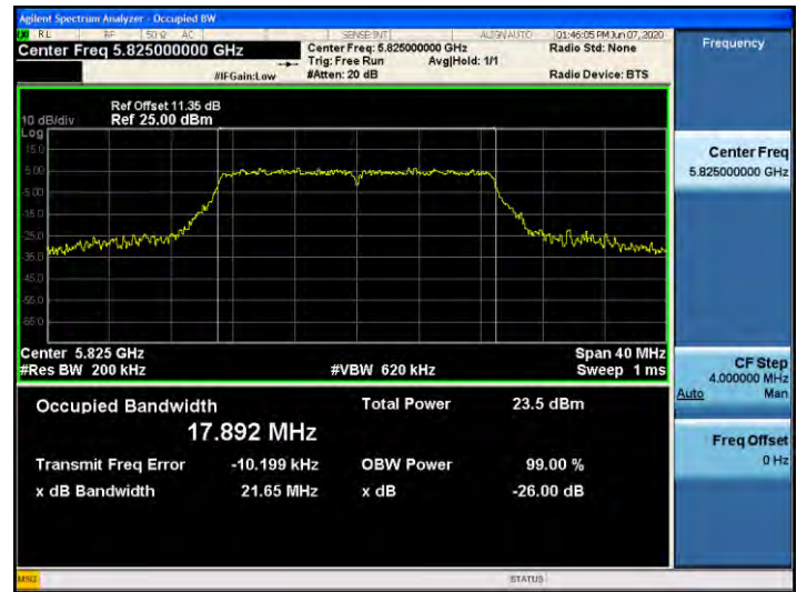
802.11ac_VHT20 UNII 3 BAND 26dB Bandwidth(CH 165)
