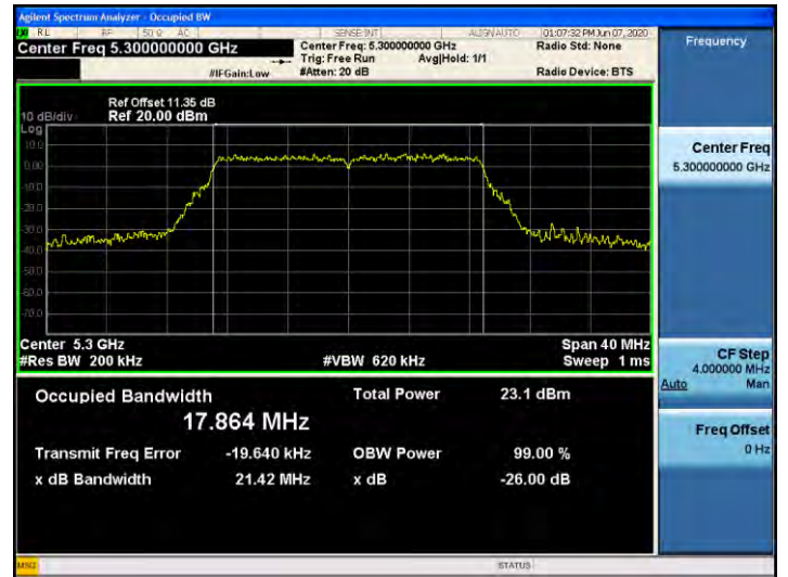
802.11ac_VHT20 UNII 3 BAND 26dB Bandwidth(CH 165)
