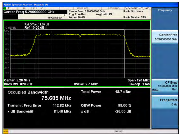
802.11ac_VHT80 UNII 3 BAND 26dB Bandwidth (CH 155)
