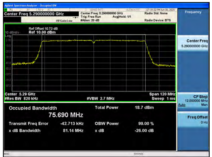
802.11ac_VHT80 UNII 3 BAND 26dB Bandwidth (CH 155)
