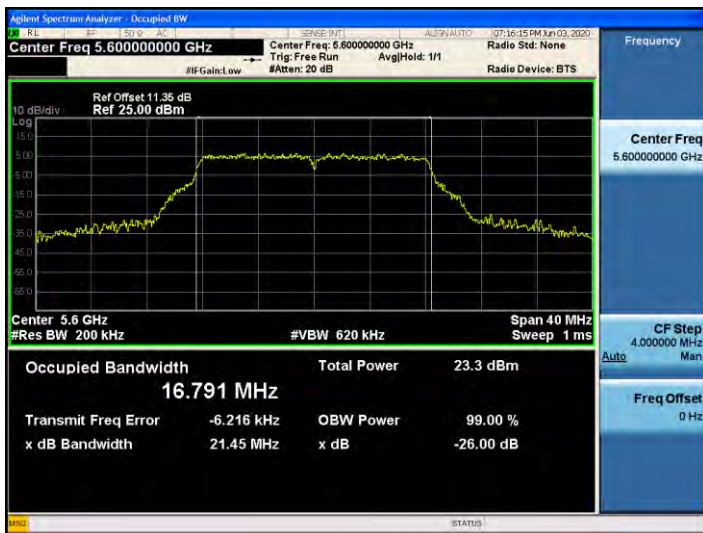
802.11a UNII 2C BAND 26dB Bandwidth (CH 120)
