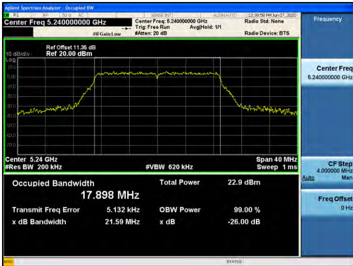
802.11n_HT20 UNII 2C BAND 26dB Bandwidth(CH 144)
