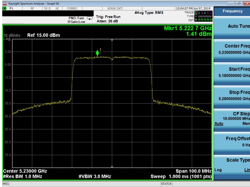
Plot 7-145. Power Spectral Density Plot SISO ANT1 (40MHz BW 802.11ax (UNII Band 1) – Ch. 46)
