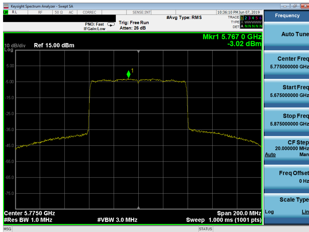
Plot 7-198. Power Spectral Density Plot SISO ANT1 (80MHz BW 802.11ax (UNII Band 3) – Ch. 155)
