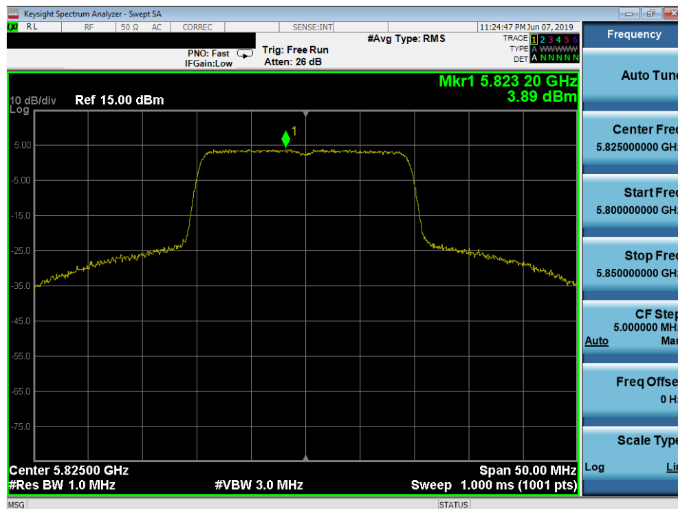
Plot 7-258. Power Spectral Density Plot SISO ANT2 (20MHz BW 802.11ax (UNII Band 3) – Ch. 165)
