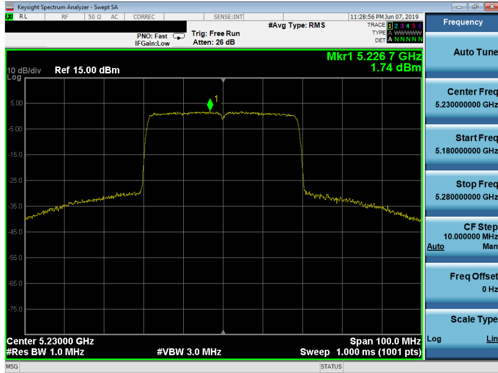
Plot 7-211. Power Spectral Density Plot SISO ANT2 (40MHz BW 802.11ax (UNII Band 1) – Ch. 46)
