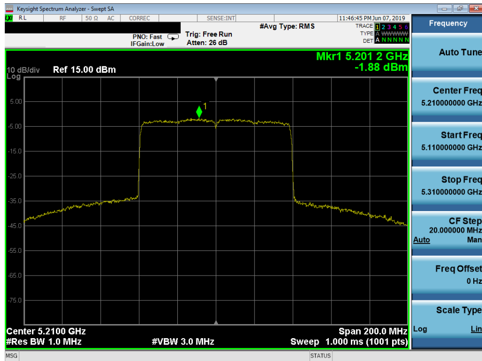
Plot 7-213. Power Spectral Density Plot SISO ANT2 (80MHz BW 802.11ax (UNII Band 1) – Ch. 42)
