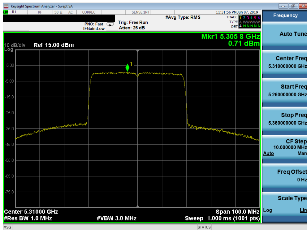
Plot 7-226. Power Spectral Density Plot SISO ANT2 (40MHz BW 802.11ax (UNII Band 2A) – Ch. 62)
