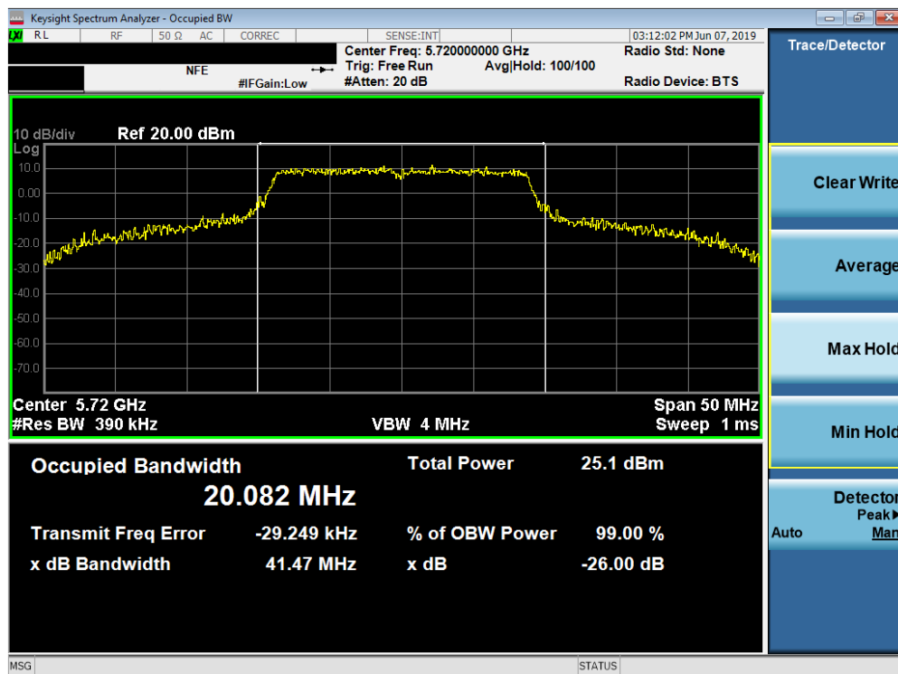
Plot 7-87. 26dB Bandwidth Plot SISO ANT2 (20MHz BW 802.11n (UNII Band 2C) – Ch. 144)
