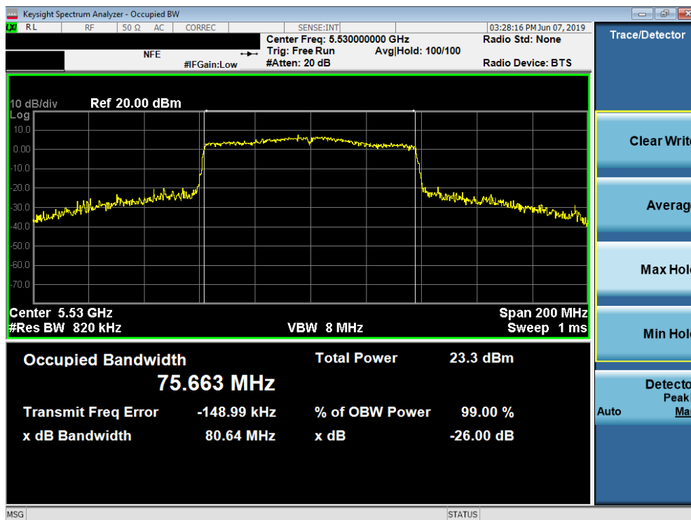
Plot 7-97. 26dB Bandwidth Plot SISO ANT2 (80MHz BW 802.11ac (UNII Band 2C) – Ch. 106)
