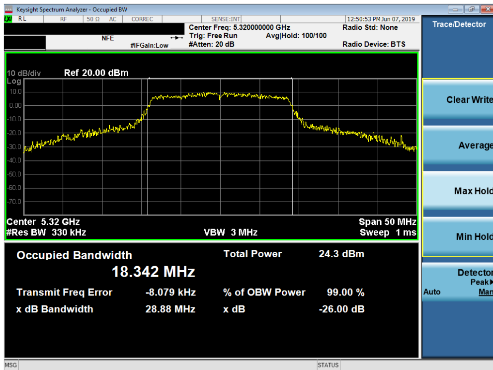
Plot 7-21. 26dB Bandwidth Plot SISO ANT1 (20MHz BW 802.11n (UNII Band 2A) – Ch. 64)
