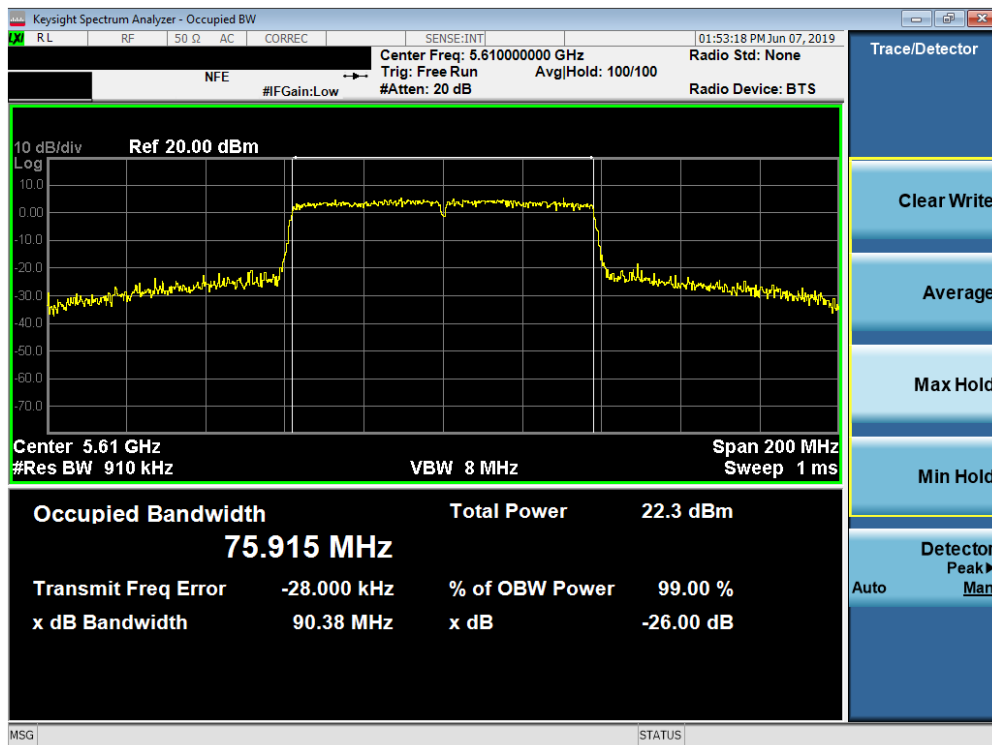
Plot 7-47. 26dB Bandwidth Plot SISO ANT1 (80MHz BW 802.11ac (UNII Band 2C) – Ch. 122)
