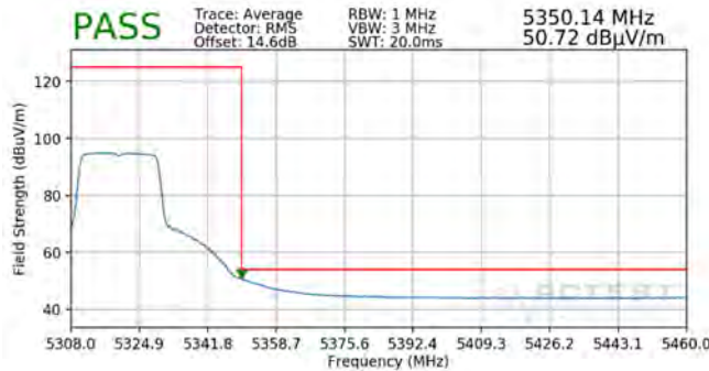
Plot 7-384. Radiated Upper Band Edge Plot SISO ANT2 (Average - UNII Band 2A - 242 Tones)
