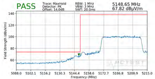
Plot 7-390. Radiated Lower Band Edge Plot SISO ANT2 (Peak – UNII Band 1 – 484 Tones)
