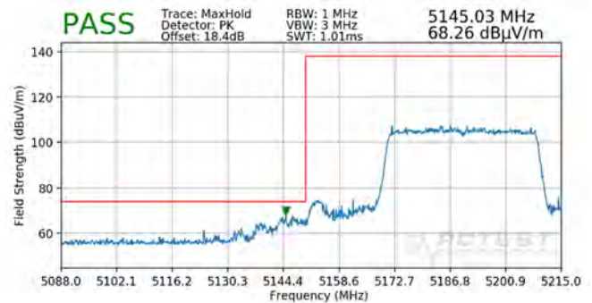
Plot 7-411. Radiated Lower Band Edge Plot MIMO (Peak – UNII Band 1 – 484 Tones)
