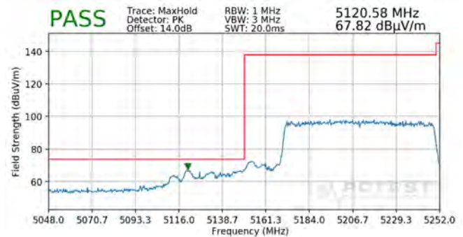
Plot 7-397. Radiated Lower Band Edge Plot SISO ANT2 (Peak – UNII Band 1 – 996 Tones)
