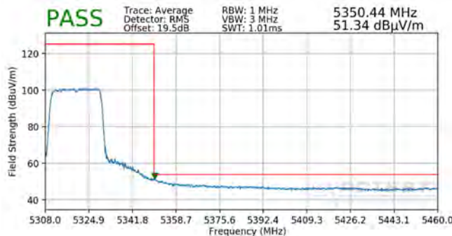
Plot 7-405. Radiated Upper Band Edge Plot MIMO (Average - UNII Band 2A - 242 Tones)
