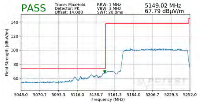
Plot 7-376. Radiated Lower Band Edge Plot SISO ANT1 (Peak – UNII Band 1 – 996 Tones)
