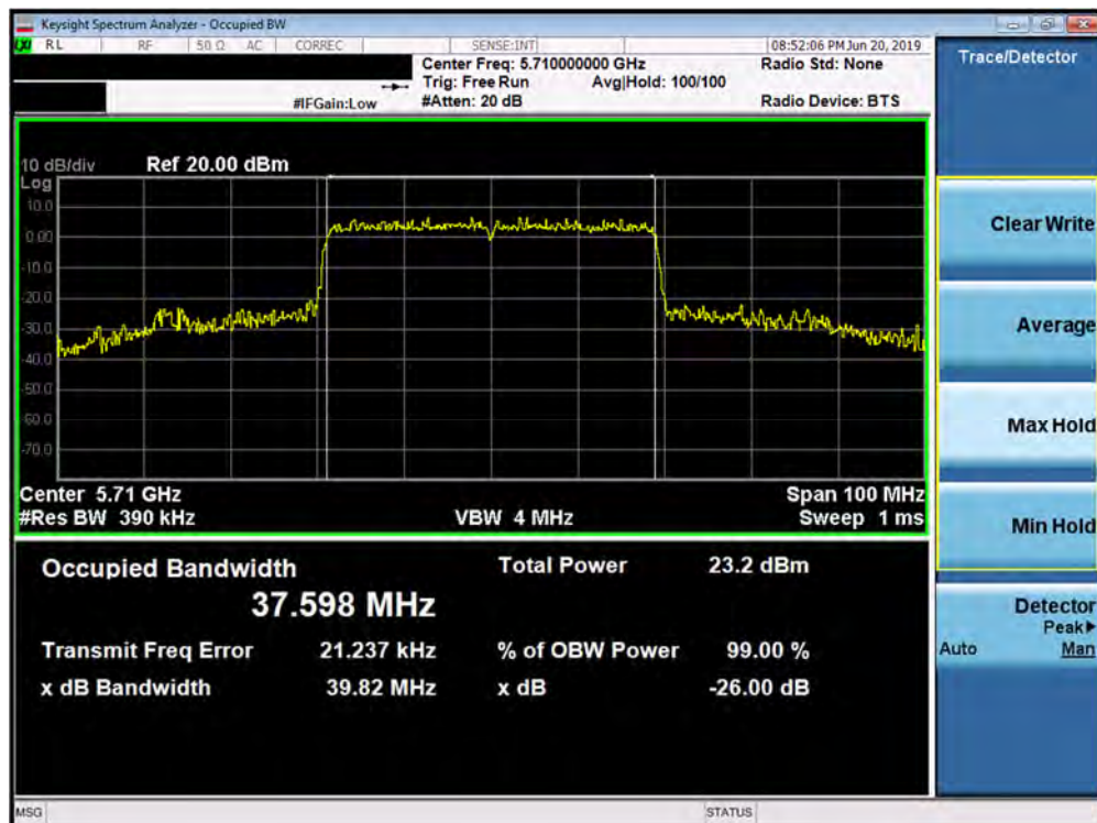
Plot 7-39. 26dB Bandwidth Plot SISO ANT1 (40MHz BW 802.11ax – Full Tones (UNII Band 2C) – Ch. 142)
