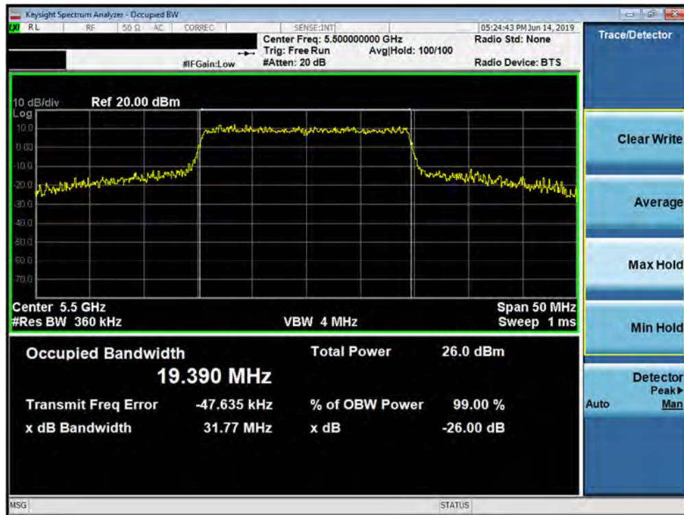
Plot 7-76. 26dB Bandwidth Plot SISO ANT2 (20MHz BW 802.11ax – Full Tones (UNII Band 2C) – Ch. 100)
