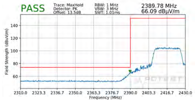
Plot 7-118. Radiated Restricted Lower Band Edge Measurement SISO ANT2 (Peak – 242 Tones)
