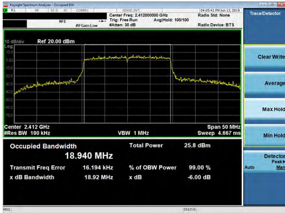
Plot 7-10. 6dB Bandwidth Plot SISO ANT2 (802.11ax OFDMA – 242 Tones – Ch. 1)
