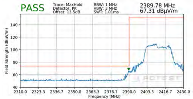
Plot 7-94. Radiated Restricted Lower Band Edge Measurement SISO ANT1 (Peak – 106 Tones)
