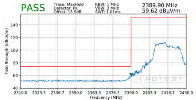
Plot 7-96. Radiated Restricted Lower Band Edge Measurement SISO ANT1 (Peak – 106 Tones)
