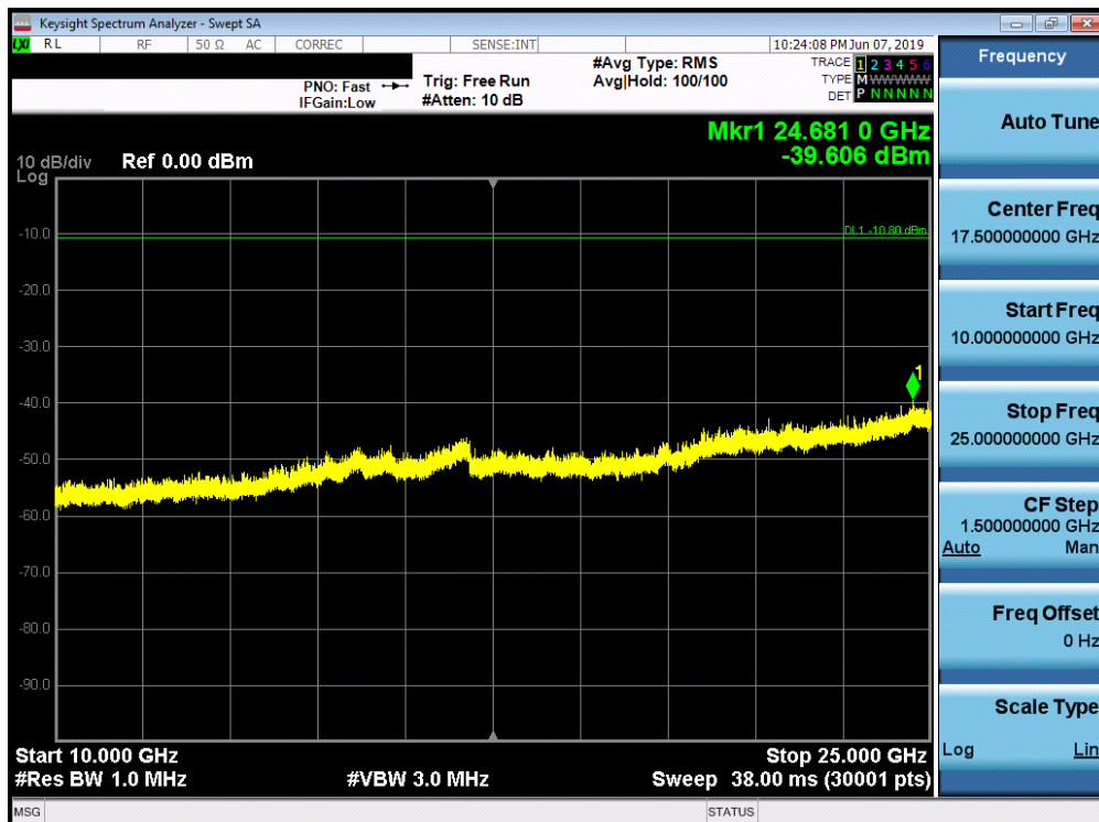
Plot 7-54. Conducted Spurious Plot SISO ANT1 (802.11ax OFDMA – 242 Tones – Ch. 6)
