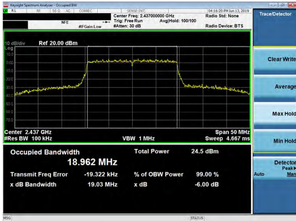
Plot 7-11. 6dB Bandwidth Plot SISO ANT2 (802.11ax OFDMA – 242 Tones – Ch. 6)
