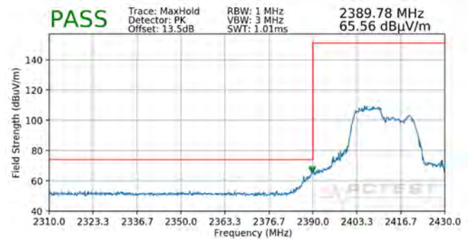
Plot 7-108. Radiated Restricted Lower Band Edge Measurement SISO ANT2 (Peak – 106 Tones)
