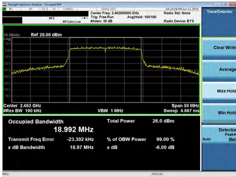
Plot 7-12. 6dB Bandwidth Plot SISO ANT2 (802.11ax OFDMA – 242 Tones – Ch. 11)
