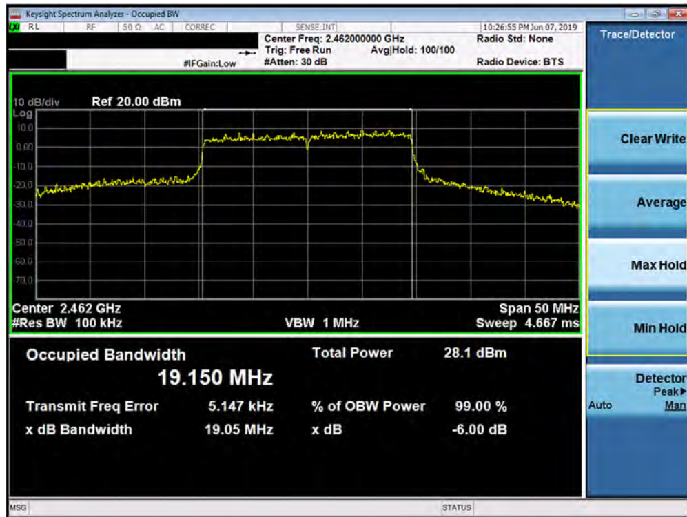
Plot 7-6. 6dB Bandwidth Plot SISO ANT1 (802.11ax OFDMA - 242 Tones - Ch. 11)
