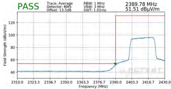
Plot 7-131. Radiated Restricted Lower Band Edge Measurement MIMO (Average – 242 Tones)
