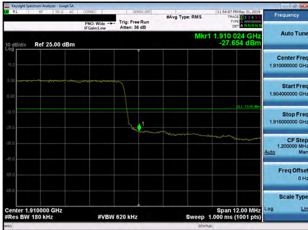
Plot 7-262. Upper Band Edge Plot (Band 2 - 15.0MHz QPSK - Full RB Configuration)
