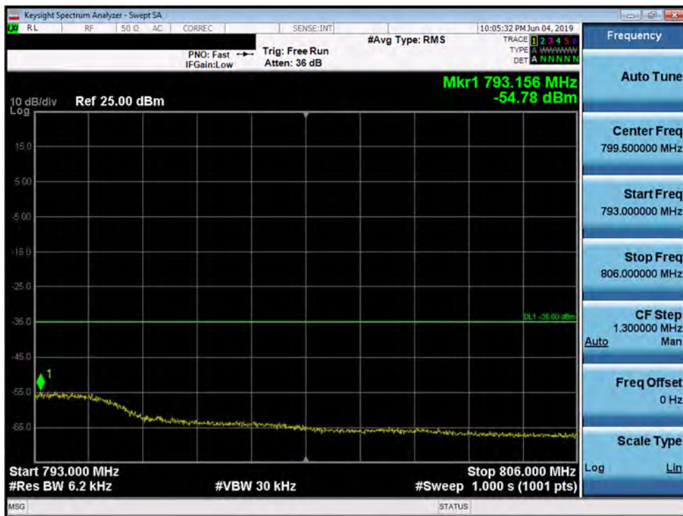
Plot 7-193. Upper Emission Mask Plot (Band 13 - 5.0MHz QPSK - Full RB Configuration)
