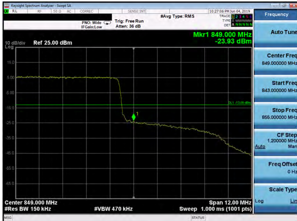
Plot 7-207. Upper Band Edge Plot (Band 26 - 15.0MHz QPSK - Full RB Configuration)
