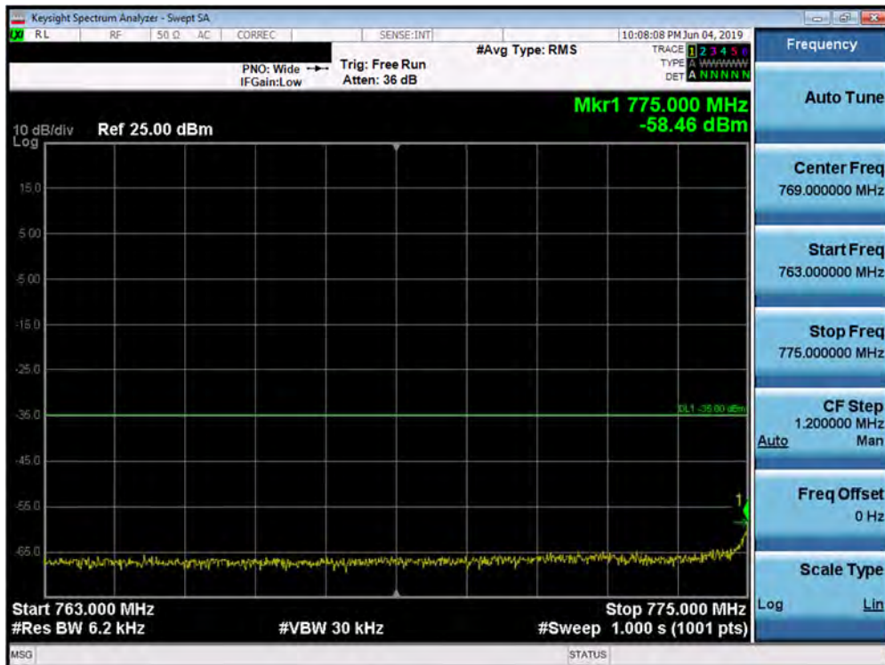
Plot 7-195. Lower Emission Mask Plot (Band 13 - 10.0MHz QPSK - Full RB Configuration)
