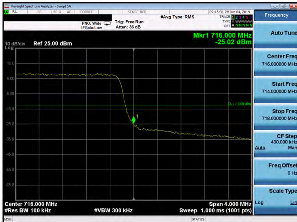
Plot 7-187. Upper Band Edge Plot (Band 12 - 5.0MHz QPSK - Full RB Configuration)
