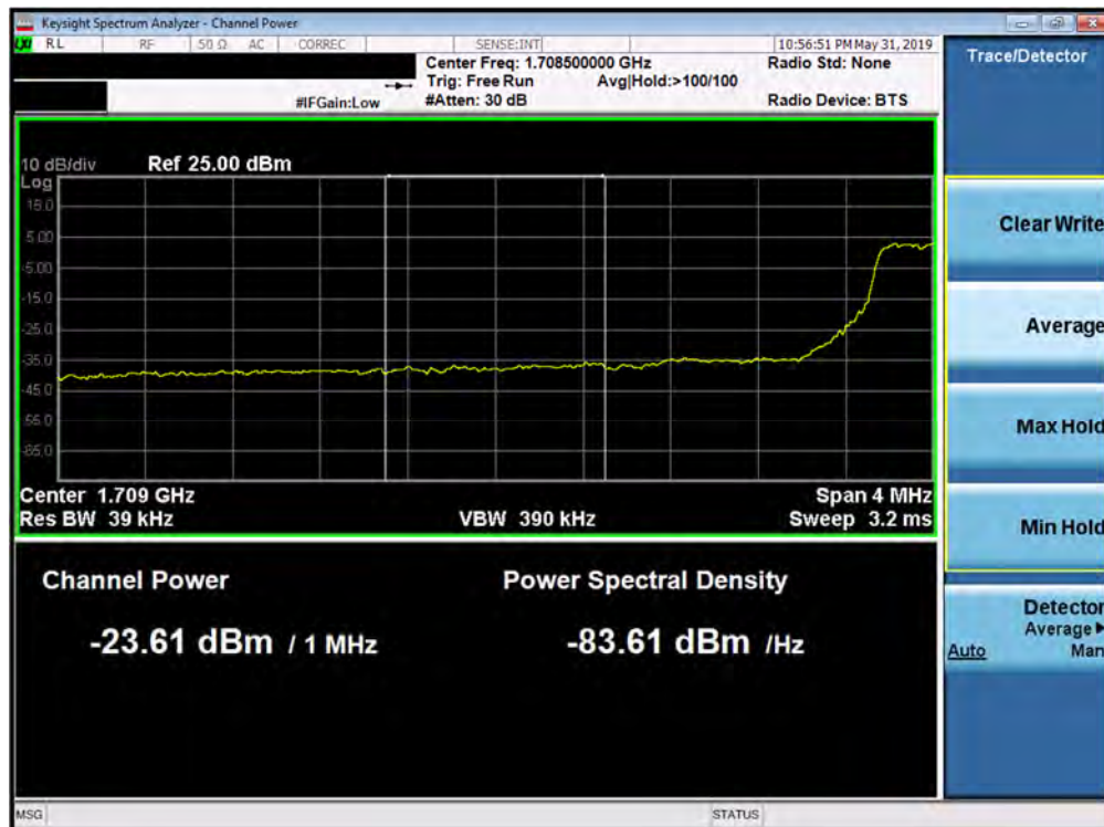
Plot 7-221. Lower Extended Band Edge Plot (Band 66/4 - 5.0MHz QPSK - Full RB Configuration)
