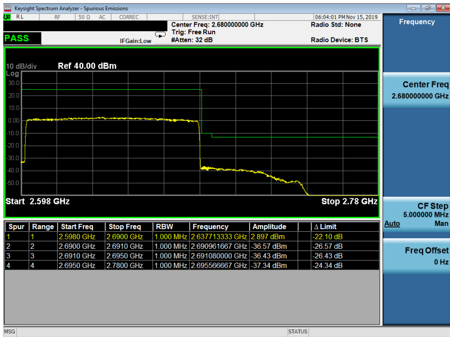
Plot 7-49. Upper ACP Plot (n41 - 90MHz DFT-QPSK - Full RB Configuration)
