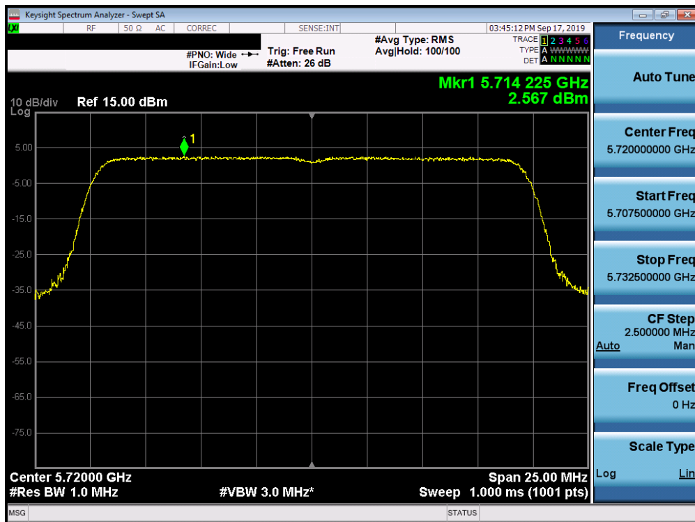
Plot 7-240. Power Spectral Density Plot SISO ANT2 (20MHz BW 802.11ax (UNII Band 2C) – Ch. 144)
