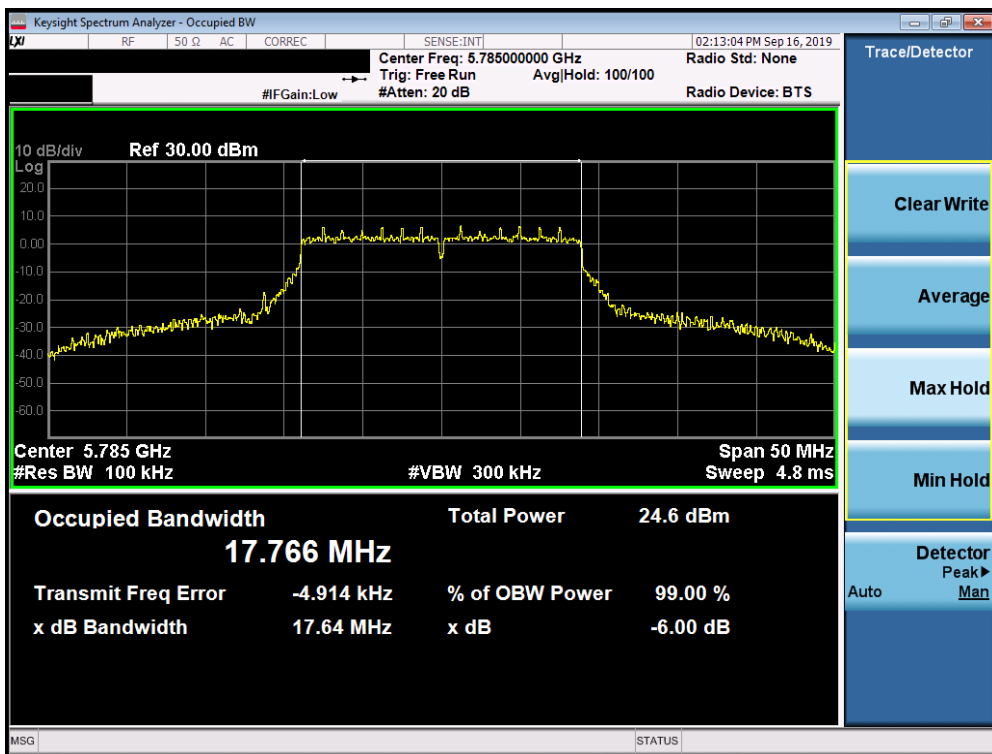
Plot 7-122. 6dB Bandwidth Plot SISO ANT2 (20MHz BW 802.11n (UNII Band 3) – Ch. 157)
