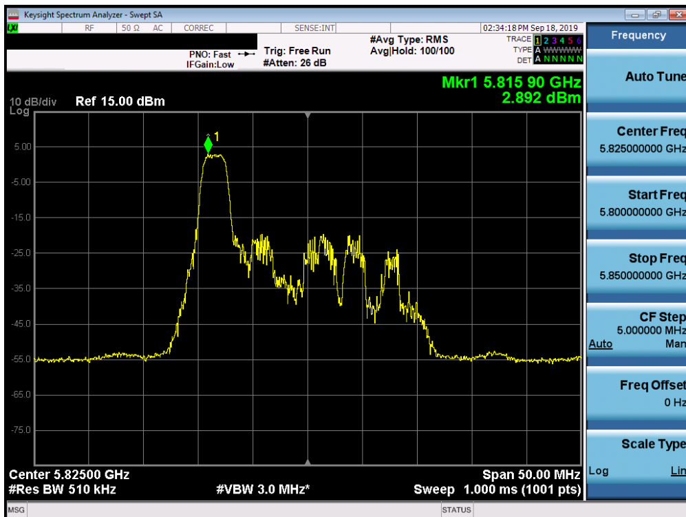
Plot 7-240. Power Spectral Density Plot MIMO ANT2 (20 MHz BW 802.11ax – Full Tones (UNII Band 3) – Ch. 165)
