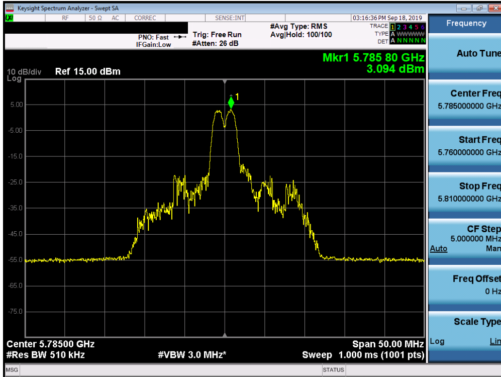
Plot 7-185. Power Spectral Density Plot MIMO ANT1 (20MHz BW 802.11ax – Full Tones (UNII Band 3) – Ch. 157)
