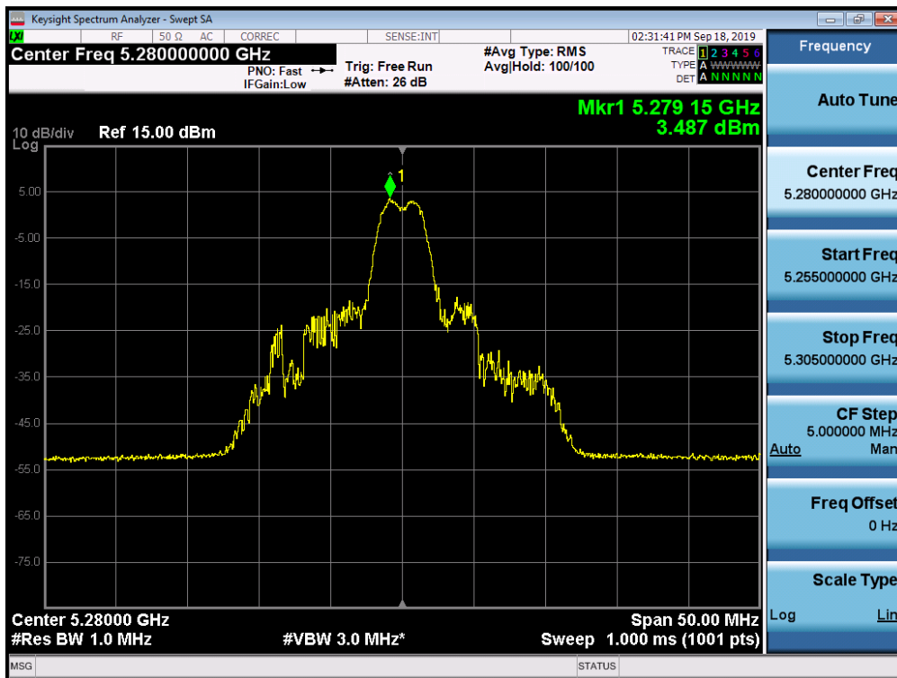
Plot 7-224. Power Spectral Density Plot MIMO ANT2 (20MHz BW 802.11ax – 26 Tones (UNII Band 2A) – Ch. 56)
