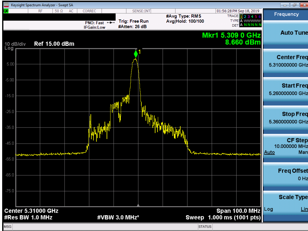
Plot 7-119. Power Spectral Density Plot SISO ANT2 (40MHz BW 802.11ax – 26 Tones (UNII Band 2A) – Ch. 62)
