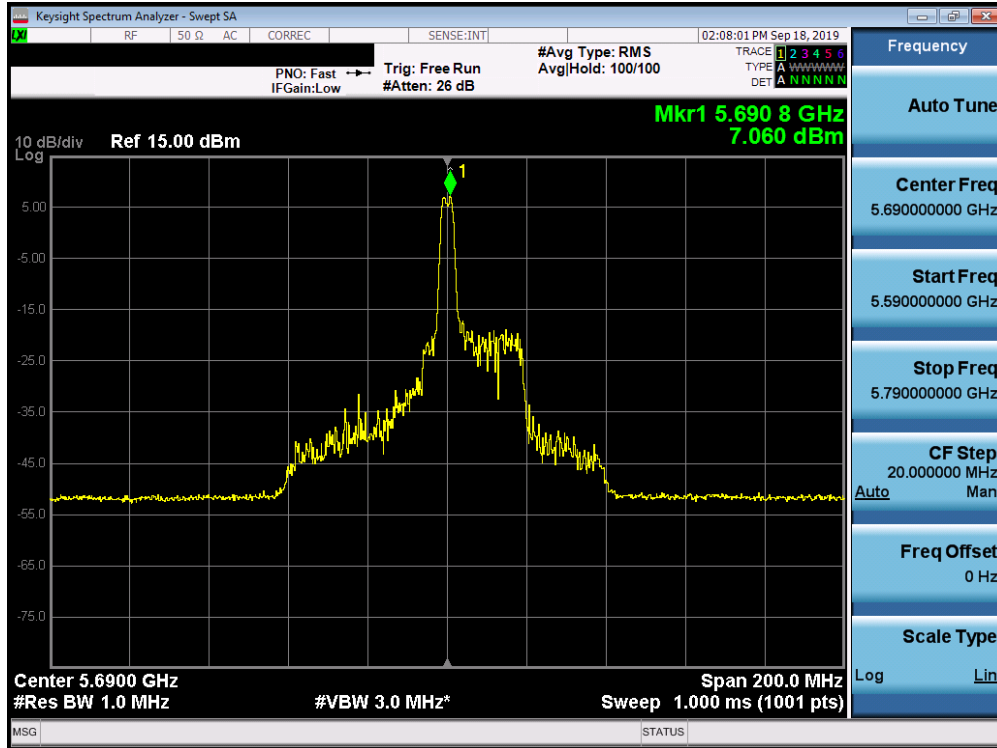
Plot 7-129. Power Spectral Density Plot SISO ANT2 (80MHz BW 802.11ax – 26 Tones (UNII Band 2C) – Ch. 138)
