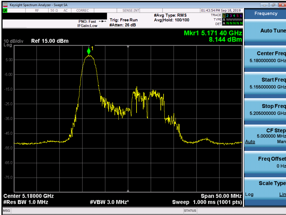
Plot 7-109. Power Spectral Density Plot SISO ANT2 (20MHz BW 802.11ax – 26 Tones (UNII Band 1) – Ch. 36)
