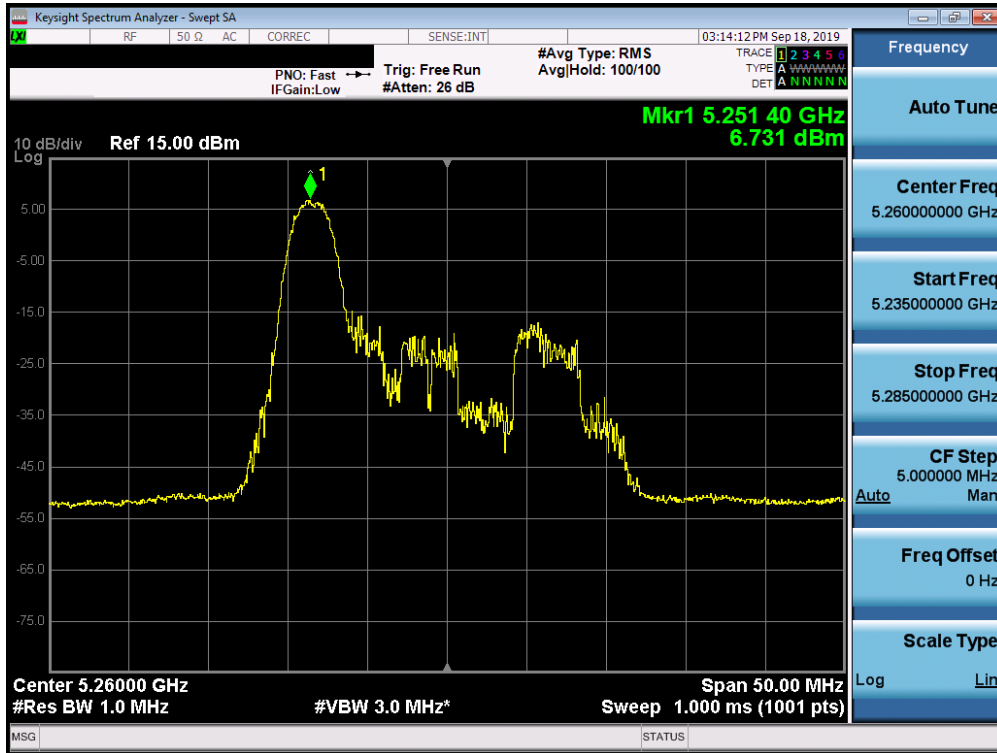
Plot 7-169. Power Spectral Density Plot MIMO ANT1 (20MHz BW 802.11ax – 26 Tones (UNII Band 2A) – Ch. 52)
