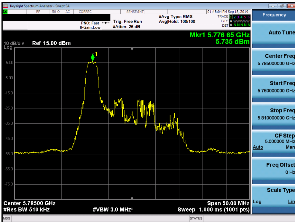
Plot 7-131. Power Spectral Density Plot SISO ANT2 (20MHz BW 802.11ax – 26 Tones (UNII Band 3) – Ch. 157)
