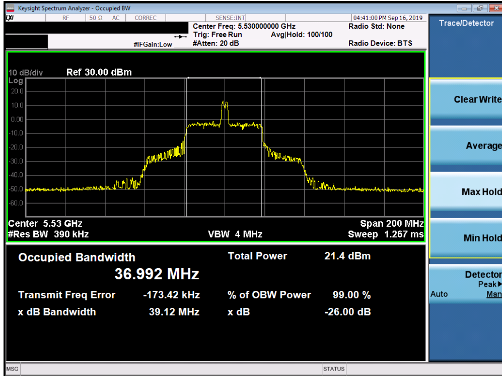
Plot 7-19. 26dB Bandwidth Plot SISO ANT1 (80MHz BW 802.11ax – 26 Tones (UNII Band 2C) – Ch. 106)
