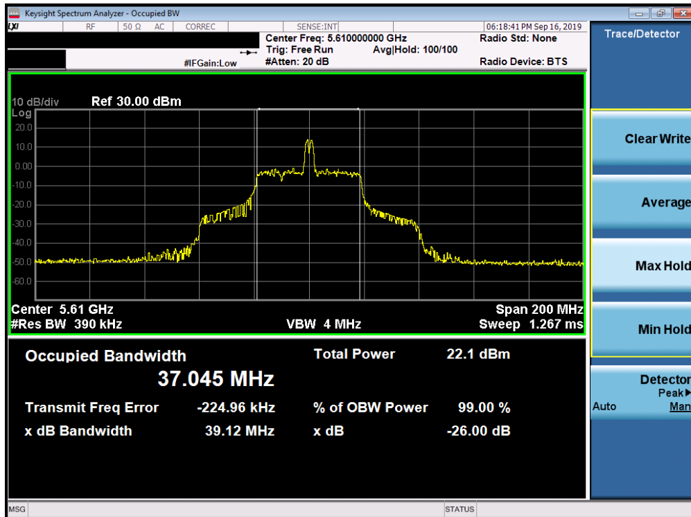
Plot 7-41. 26dB Bandwidth Plot SISO ANT2 (80MHz BW 802.11ax – 26 Tones (UNII Band 2C) – Ch. 122)
