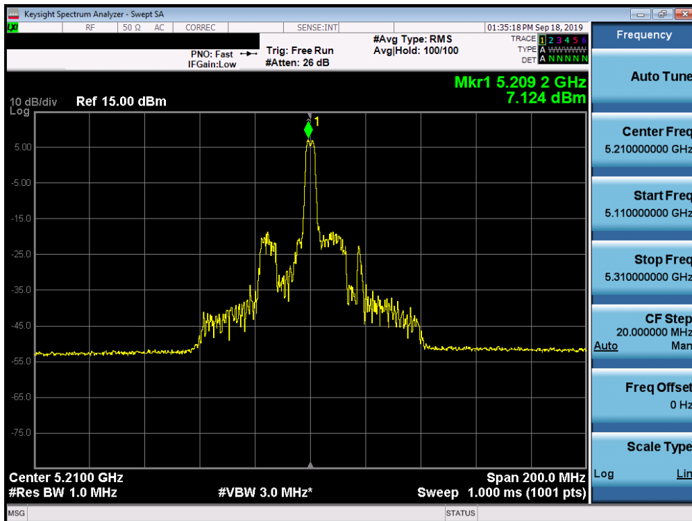
Plot 7-60. Power Spectral Density Plot SISO ANT1 (80MHz BW 802.11ax – 26 Tones (UNII Band 1) – Ch. 42)
