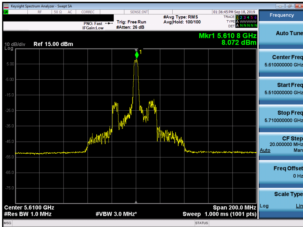
Plot 7-74. Power Spectral Density Plot SISO ANT1 (80MHz BW 802.11ax – 26 Tones (UNII Band 2C) – Ch. 122)
