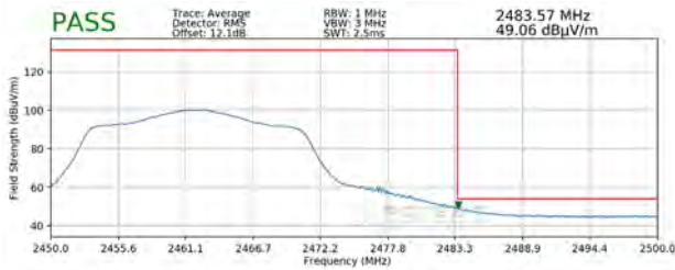
Plot 7-93. Radiated Restricted Band Edge Measurement SISO ANT1 with WCP (Average)
