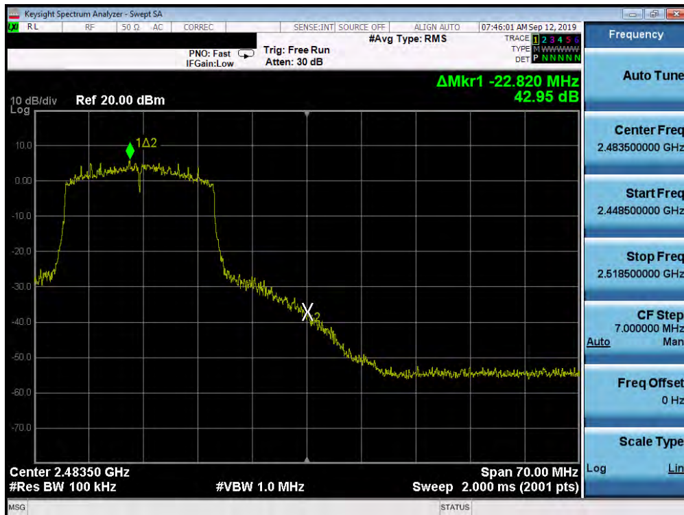
Plot 7-64. Band Edge Plot SISO ANT2 (802.11ax (2.4GHz) – Ch. 11)
