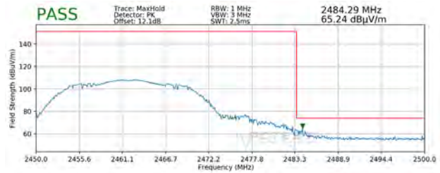
Plot 7-94. Radiated Restricted Band Edge Measurement SISO ANT1 with WCP (Peak)
