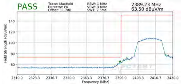
Plot 7-102. Radiated Restricted Lower Band Edge Measurement MIMO (Peak)
