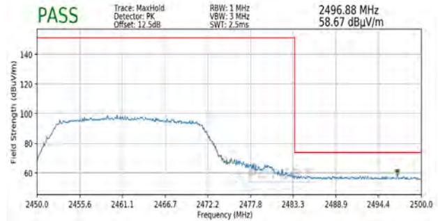
Plot 7-100. Radiated Restricted Band Edge Measurement SISO ANT2 with WCP (Peak)
