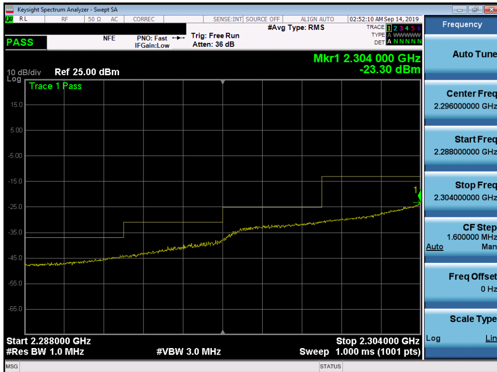
Plot 7-342. Lower Extended Band Edge Plot (Band 30 - 10.0MHz QPSK - Full RB Configuration)
