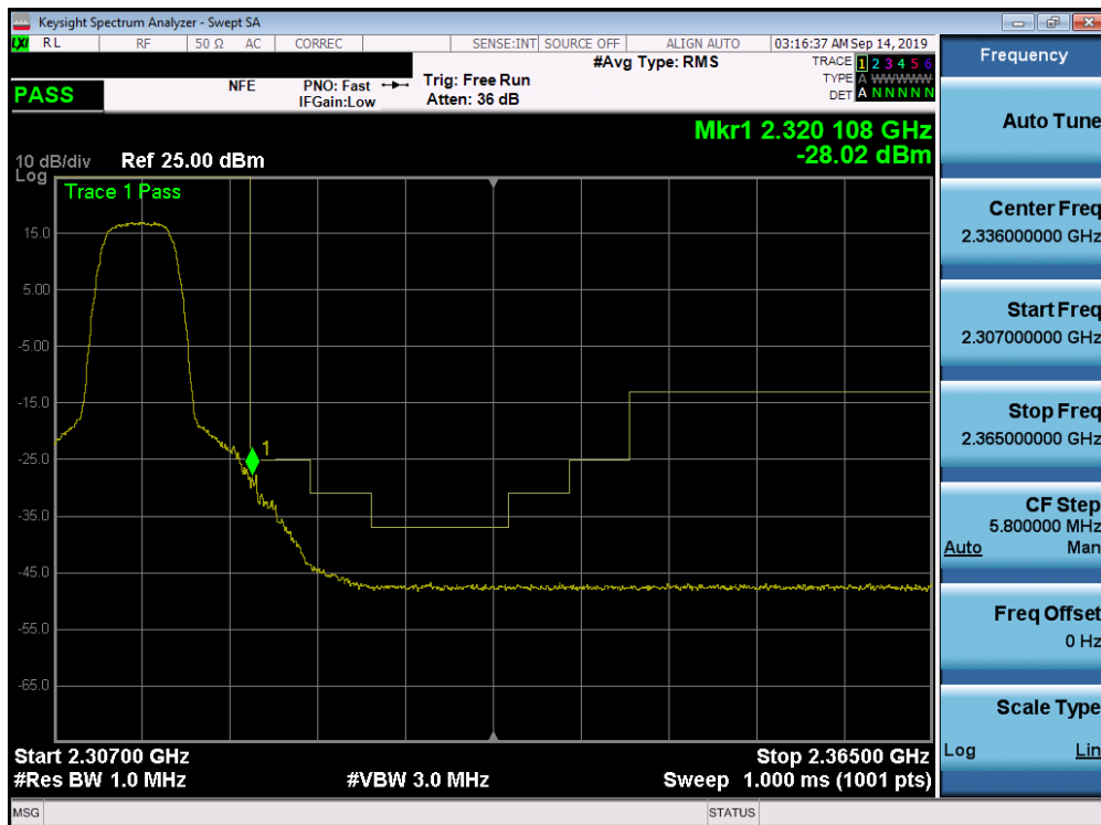
Plot 7-340. Upper Extended Band Edge Plot (Band 30 - 5.0MHz QPSK - Full RB Configuration)
