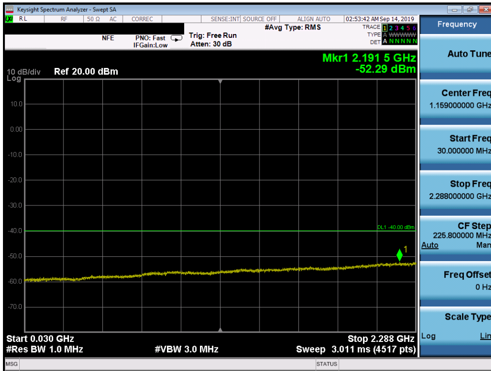
Plot 7-216. Conducted Spurious Plot (Band 30 - 10.0MHz QPSK - RB Size 1, RB Offset 0 - High Channel)
