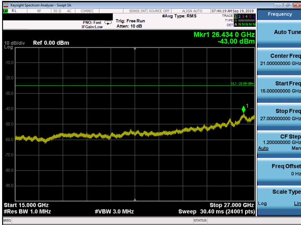
Plot 7-221. Conducted Spurious Plot (Band 7 - 20.0MHz QPSK - RB Size 1, RB Offset 0 - Low Channel)
