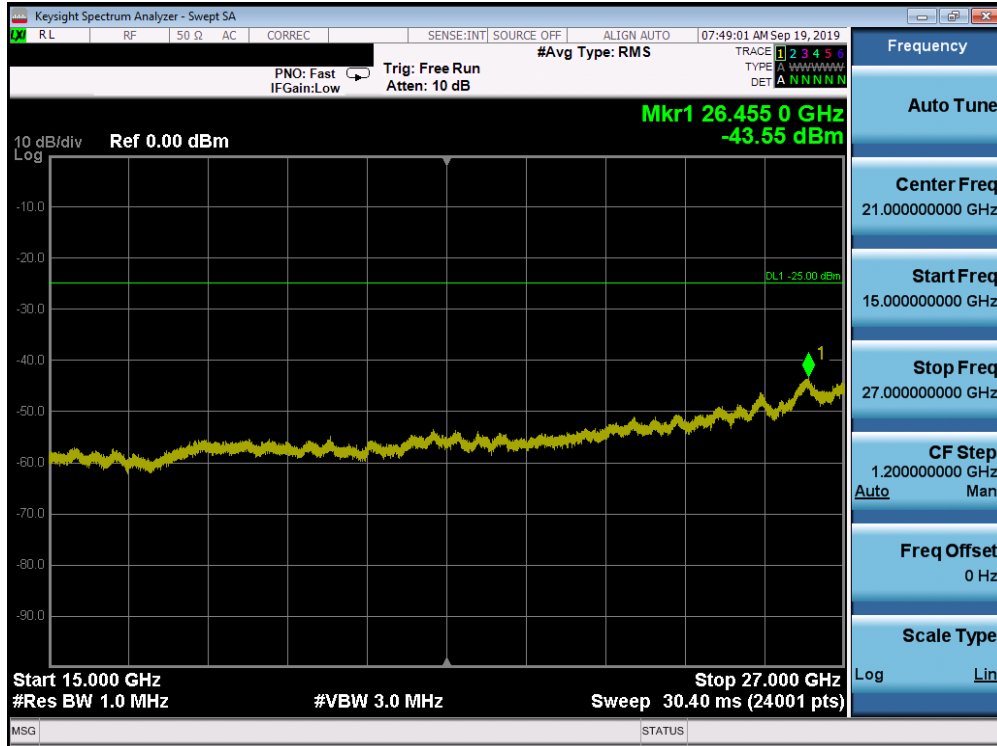
Plot 7-227. Conducted Spurious Plot (Band 7 - 20.0MHz QPSK - RB Size 1, RB Offset 0 - High Channel)
