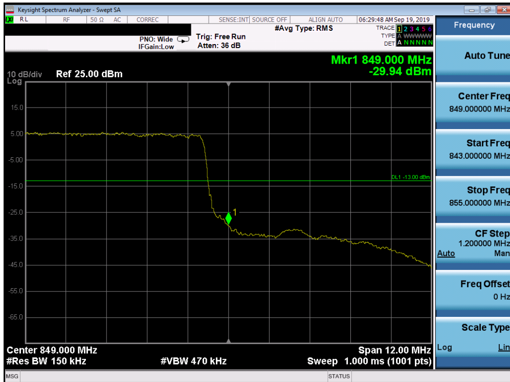
Plot 7-264. Upper Band Edge Plot (Band 26 - 15.0MHz QPSK - Full RB Configuration)
