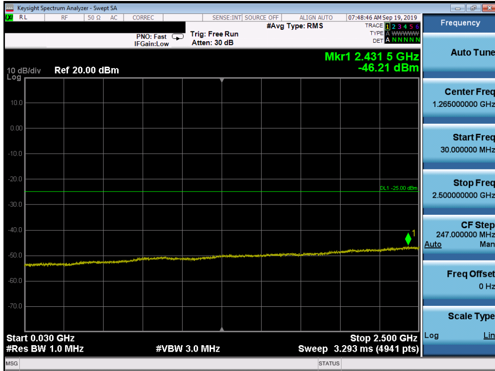
Plot 7-225. Conducted Spurious Plot (Band 7 - 20.0MHz QPSK - RB Size 1, RB Offset 0 - High Channel)
