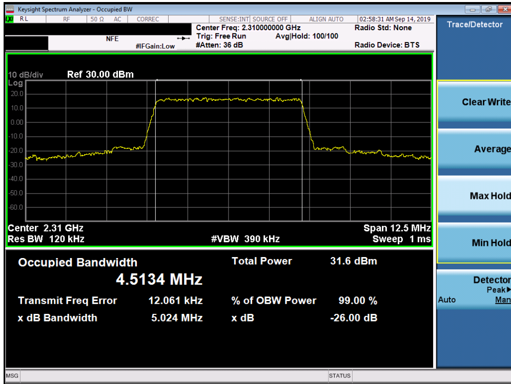
Plot 7-109. Occupied Bandwidth Plot (Band 30 - 5.0MHz QPSK - Full RB Configuration)
