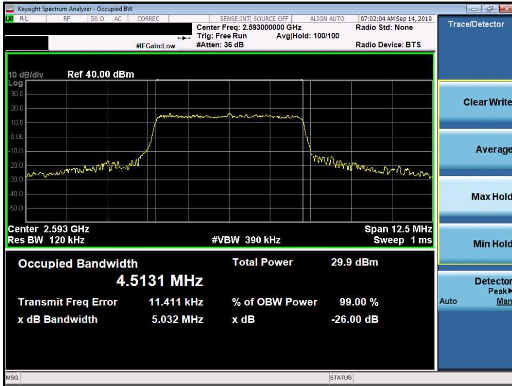
Plot 7-151. Occupied Bandwidth Plot (Band 41 PC 3 - 5.0MHz 64-QAM - Full RB Configuration)
