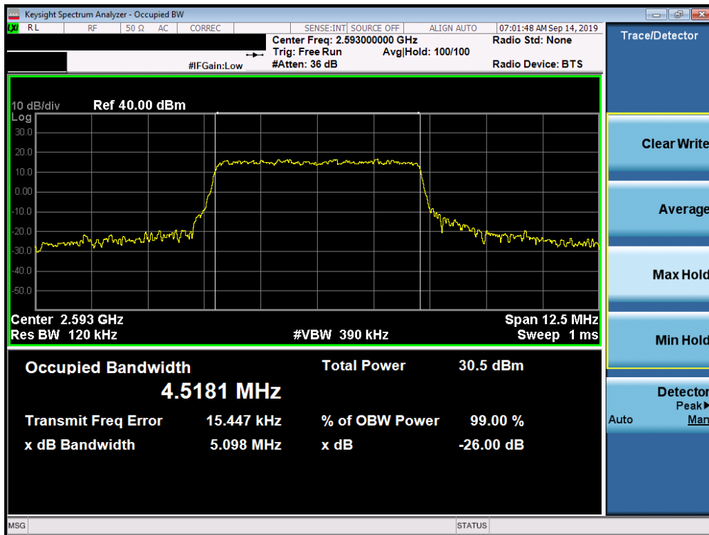
Plot 7-150. Occupied Bandwidth Plot (Band 41 PC 3 - 5.0MHz 16-QAM - Full RB Configuration)
