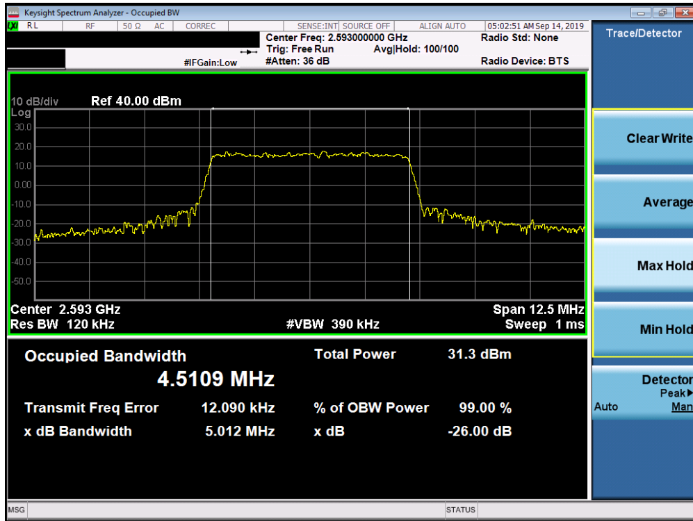
Plot 7-133. Occupied Bandwidth Plot (Band 41 PC 2 - 5.0MHz QPSK - Full RB Configuration)
