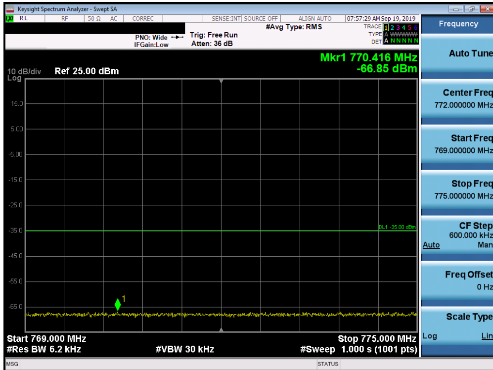
Plot 7-44. Lower Emission Mask Plot (LTE Band 14, 5MHz QPSK – RB Size 25)
