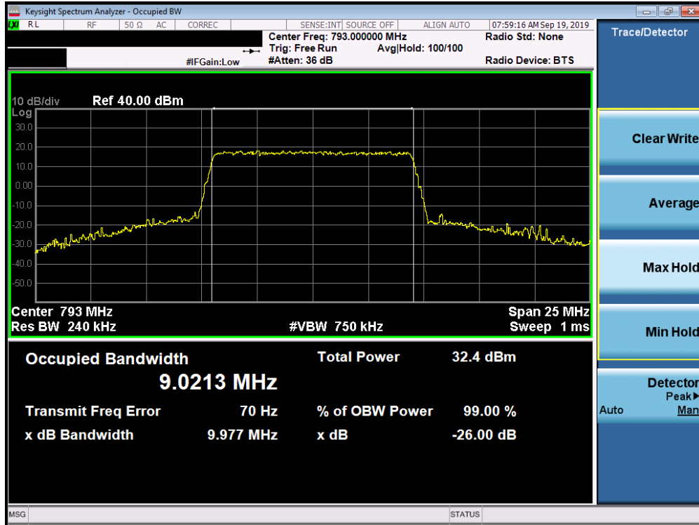
Plot 7-25. Occupied Bandwidth Plot (LTE Band 14, 10MHz QPSK – RB Size 50)
