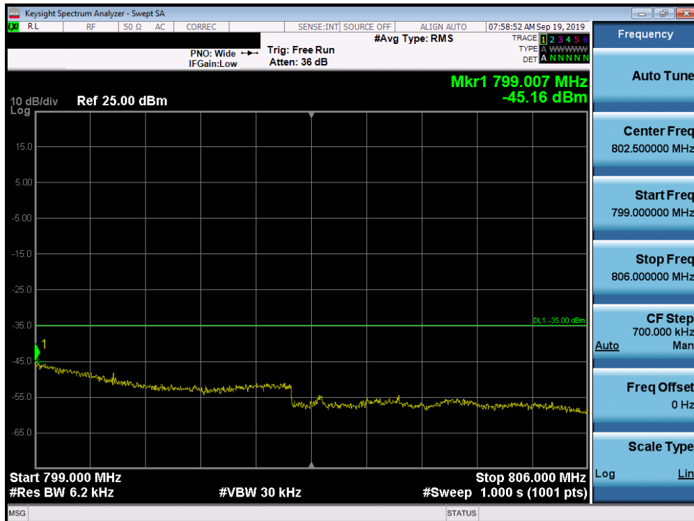
Plot 7-46. Upper Emission Mask Plot (LTE Band 14, 5MHz QPSK – RB Size 25)
