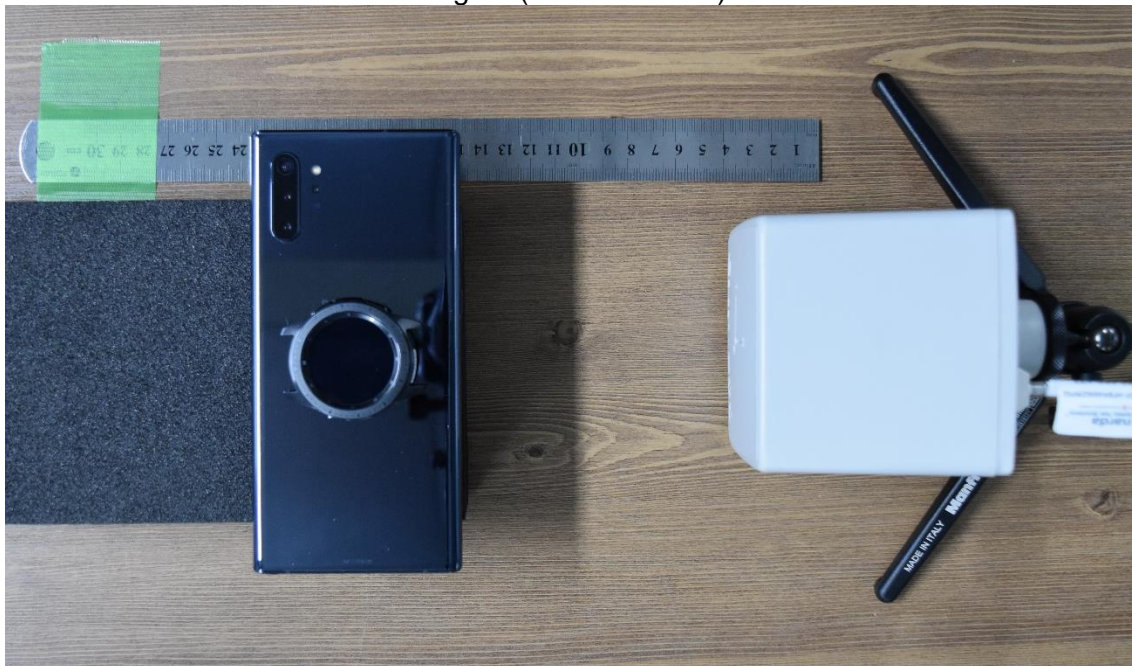
Top – charger below client (20cm distance)
