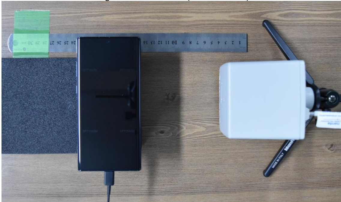
Edge 2 with USB cable (15cm distance)
